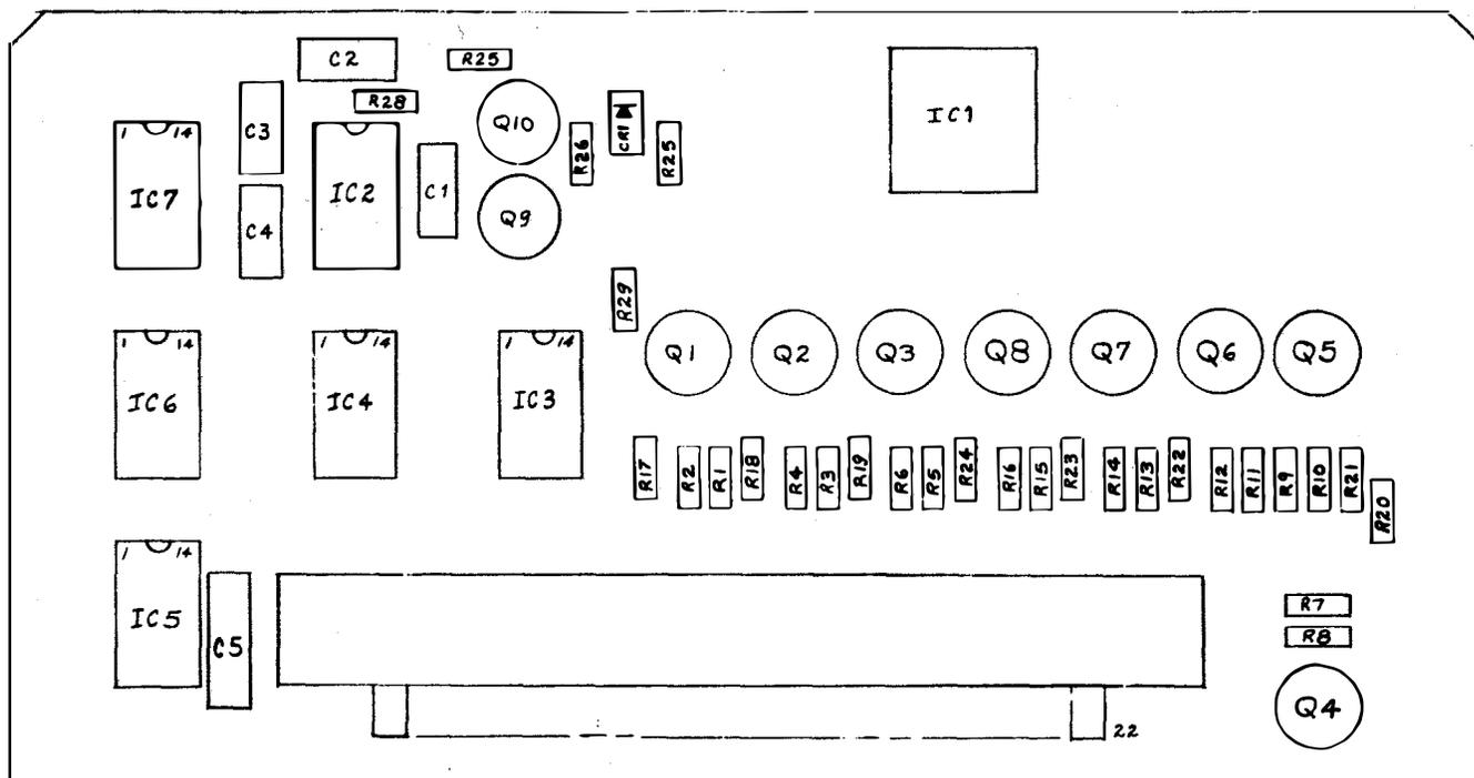
Figure 5-25. Fox Message Board 1A1A12 Component Location (36021220)
