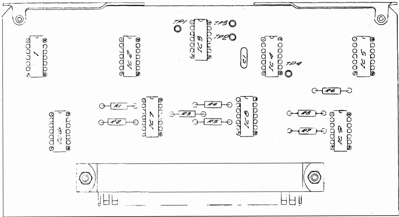
Figure 5-13. BCD Counter and Trigger II Board 1A1A7 Component Location
