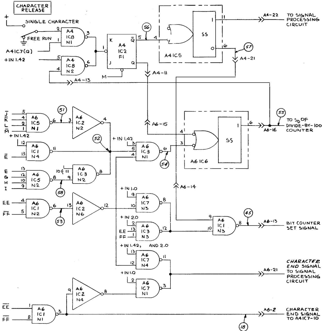
Figure 4-4. Stop Mark Generating Circuits, Simplified Schematic
