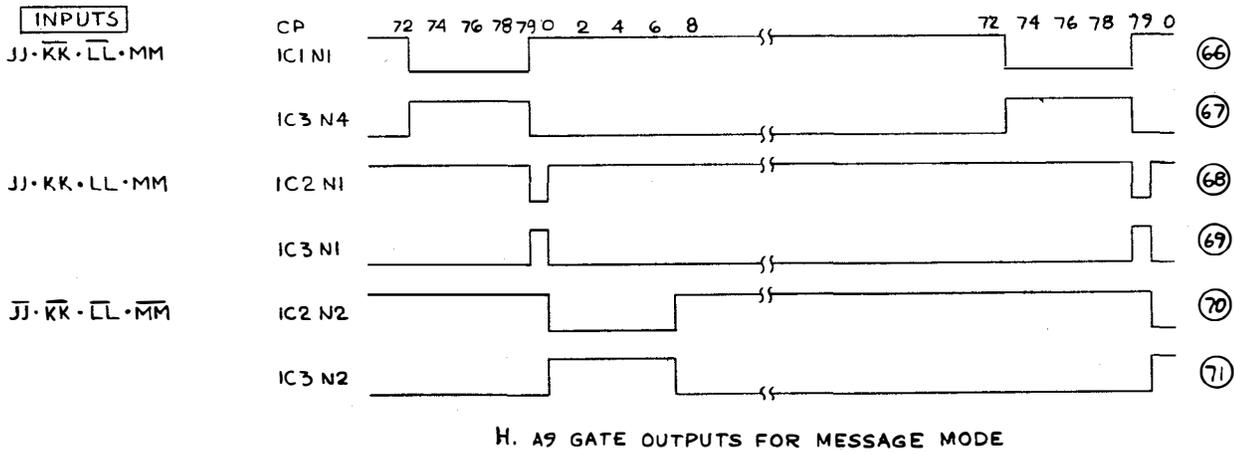
Figure 4-10. Signal Generator Timing Diagrams (Sheet 5 of 9)
