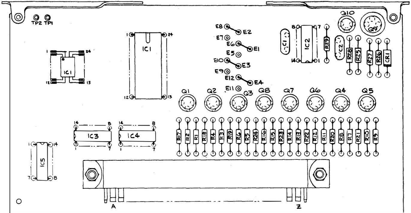
Figure 5-23. Fox Message Board 1A1A12 Component Location (36021120)
