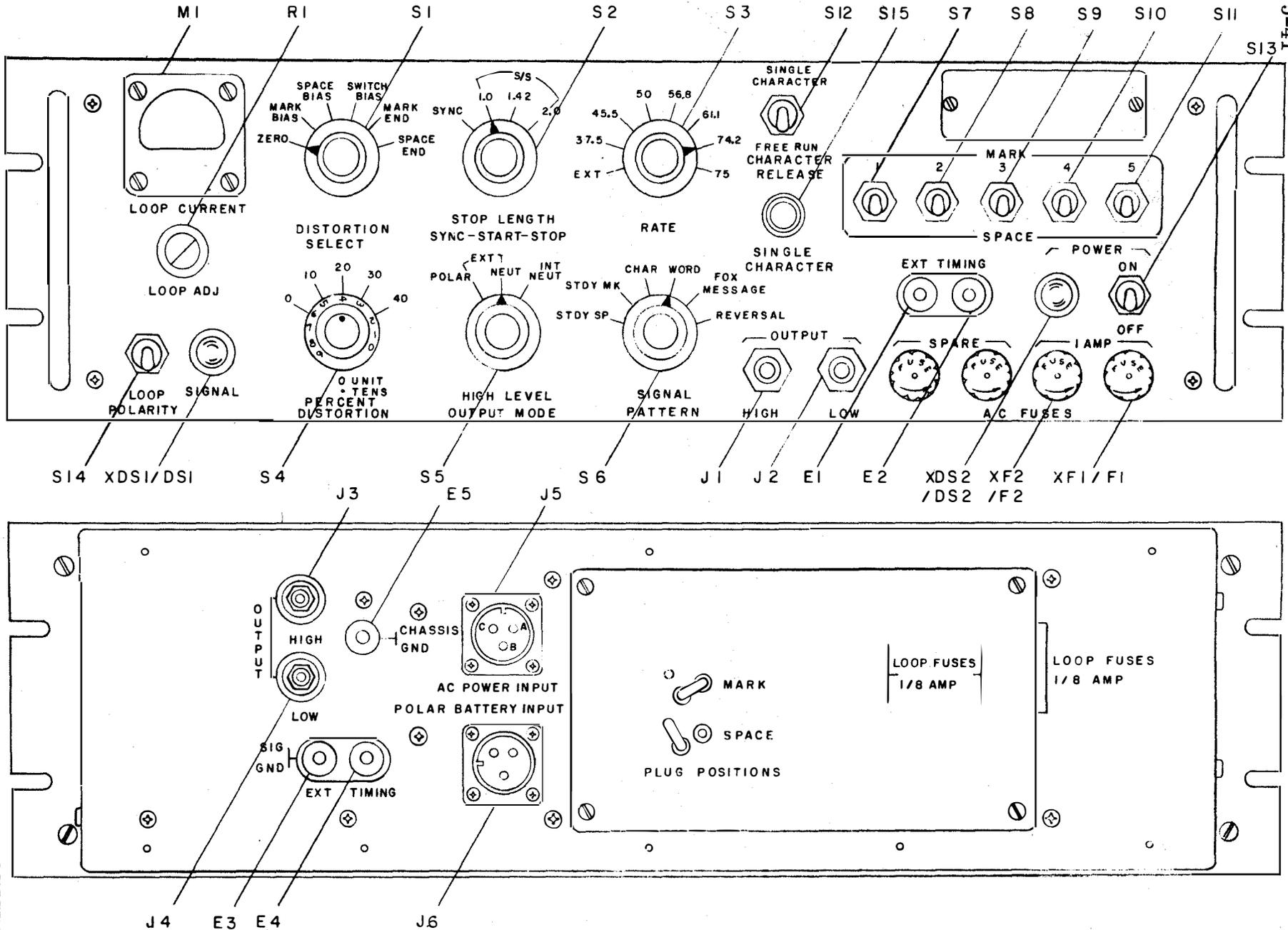
Figure 5-41. Chassis Mounted Components Location (Sheet 2 of 2)
