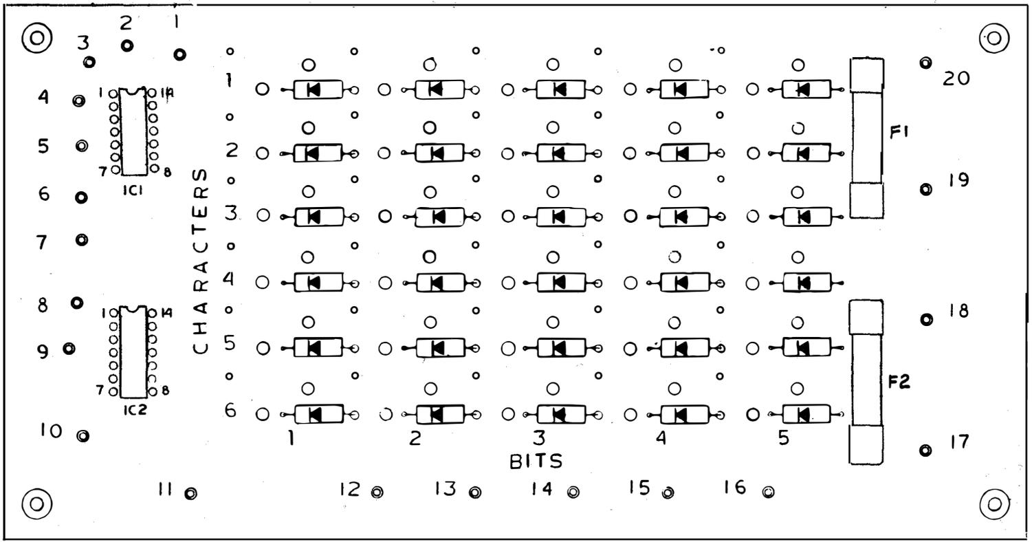
Figure 5-39. Word Matrix Board 1A2 Component Location
