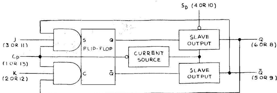
Figure 4-2. J-K Flip-Flops, Block Diagram
