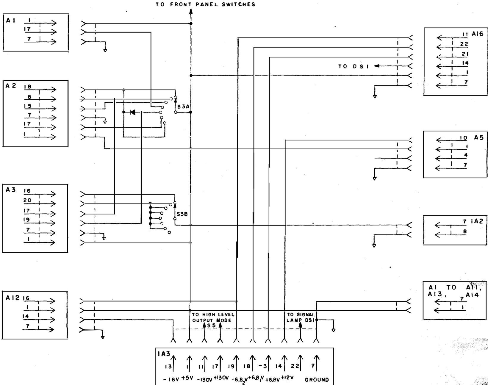
Figure 4-12. Signal Generator Power Distribution Diagram
