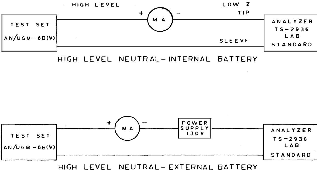
Figure 4-14. Test Setup, Neutral
