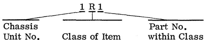
Read as: First (1) resistor (R) of chassis unit (1).
