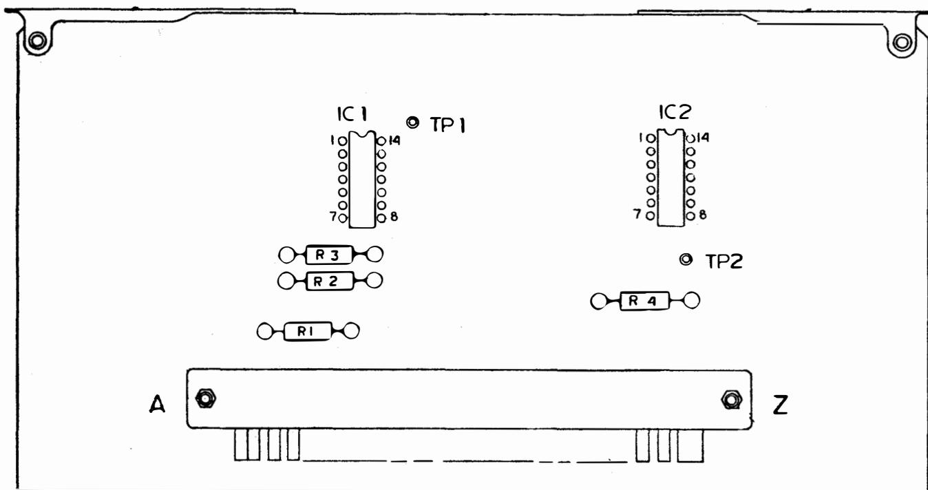
Figure 5-31. Message Select Gates 1A1A15 Components Location
