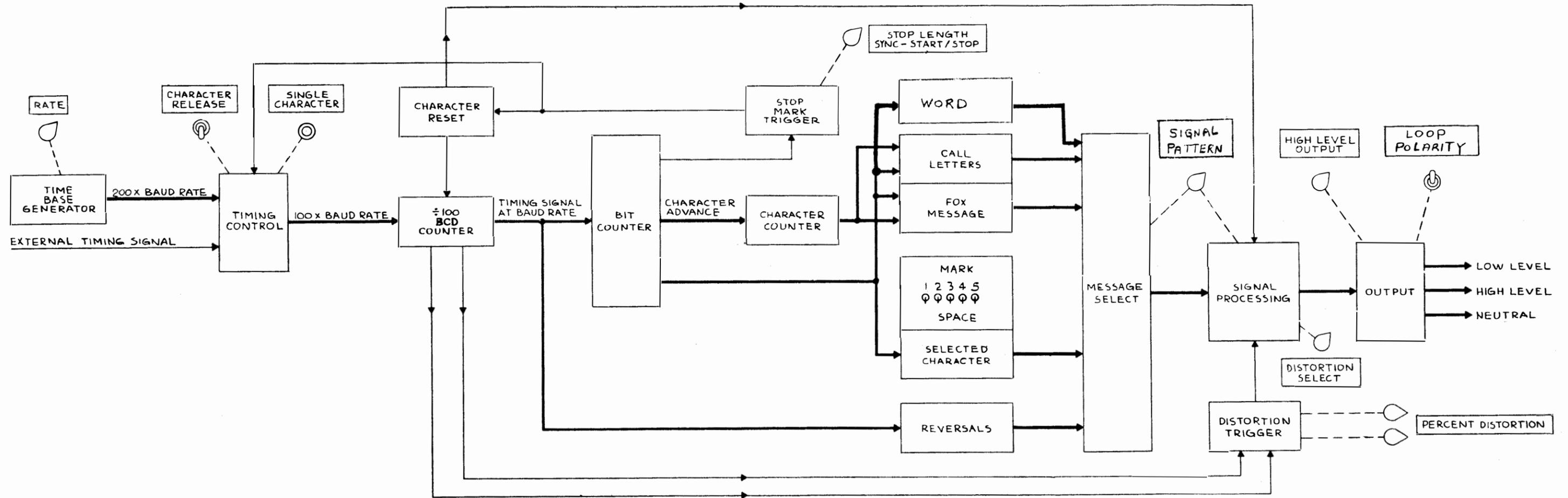
Figure 4-1. Signal Generator Functional Block Diagram
