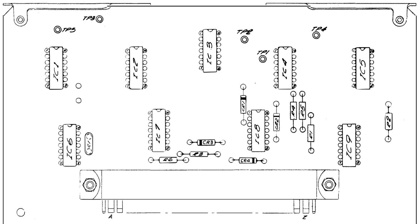
Figure 5-15. Signal Processor Board 1A1A8 Component Location
