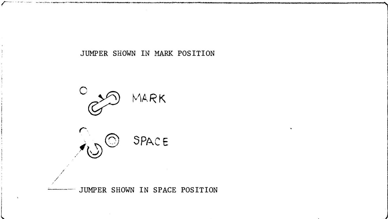
This illustration shows the position of the strapping plugs for obtaining either marks or spaces.
