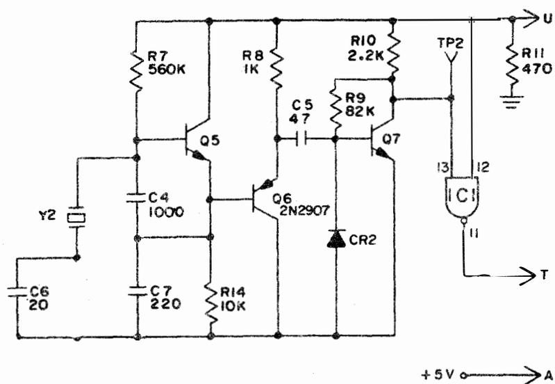
Figure 5-2. Oscillator Board 1A1A1, Schematic
