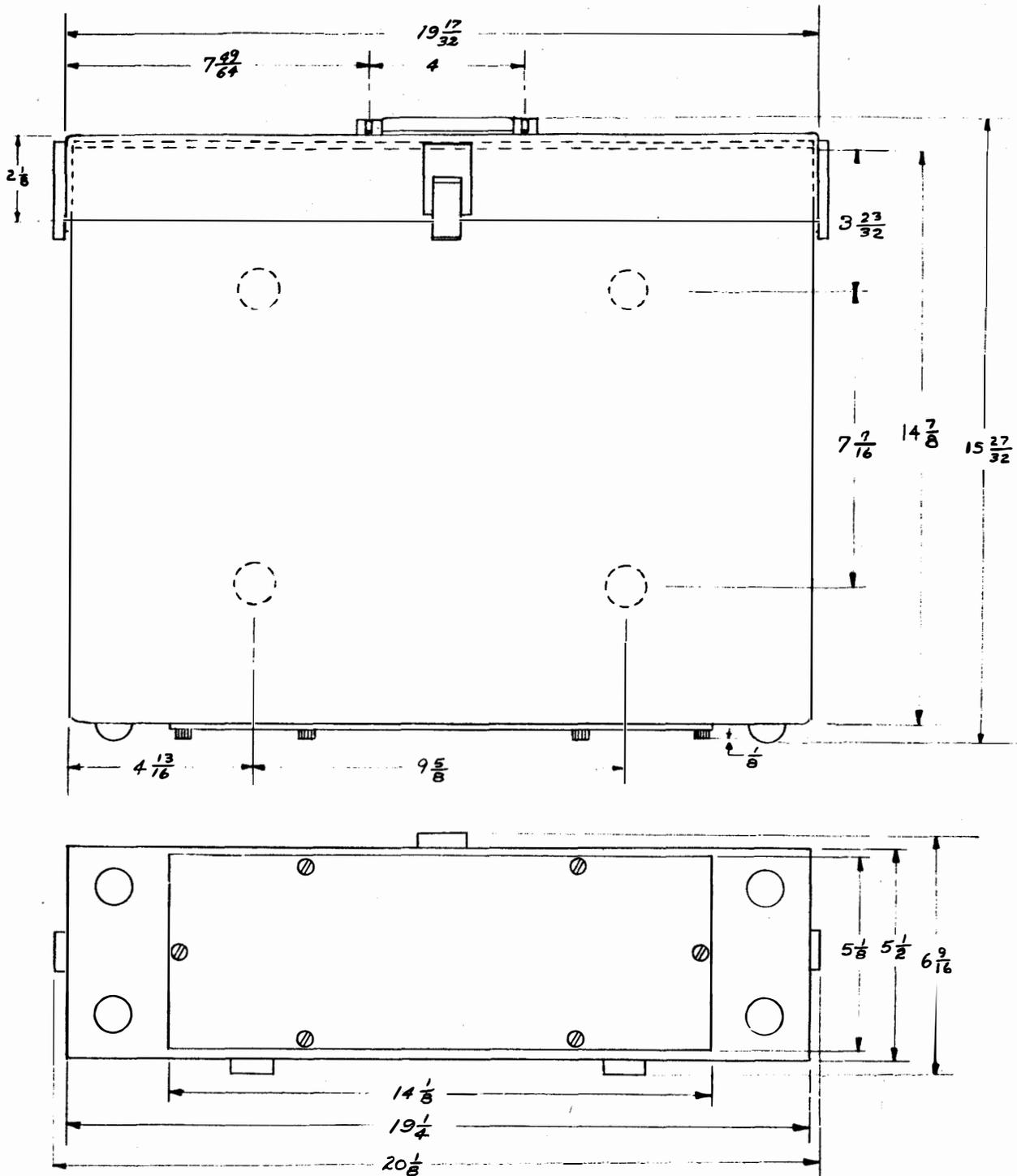
Figure 2-1. Case for Test Set, Telegraph AN/UGM-8B(V)
