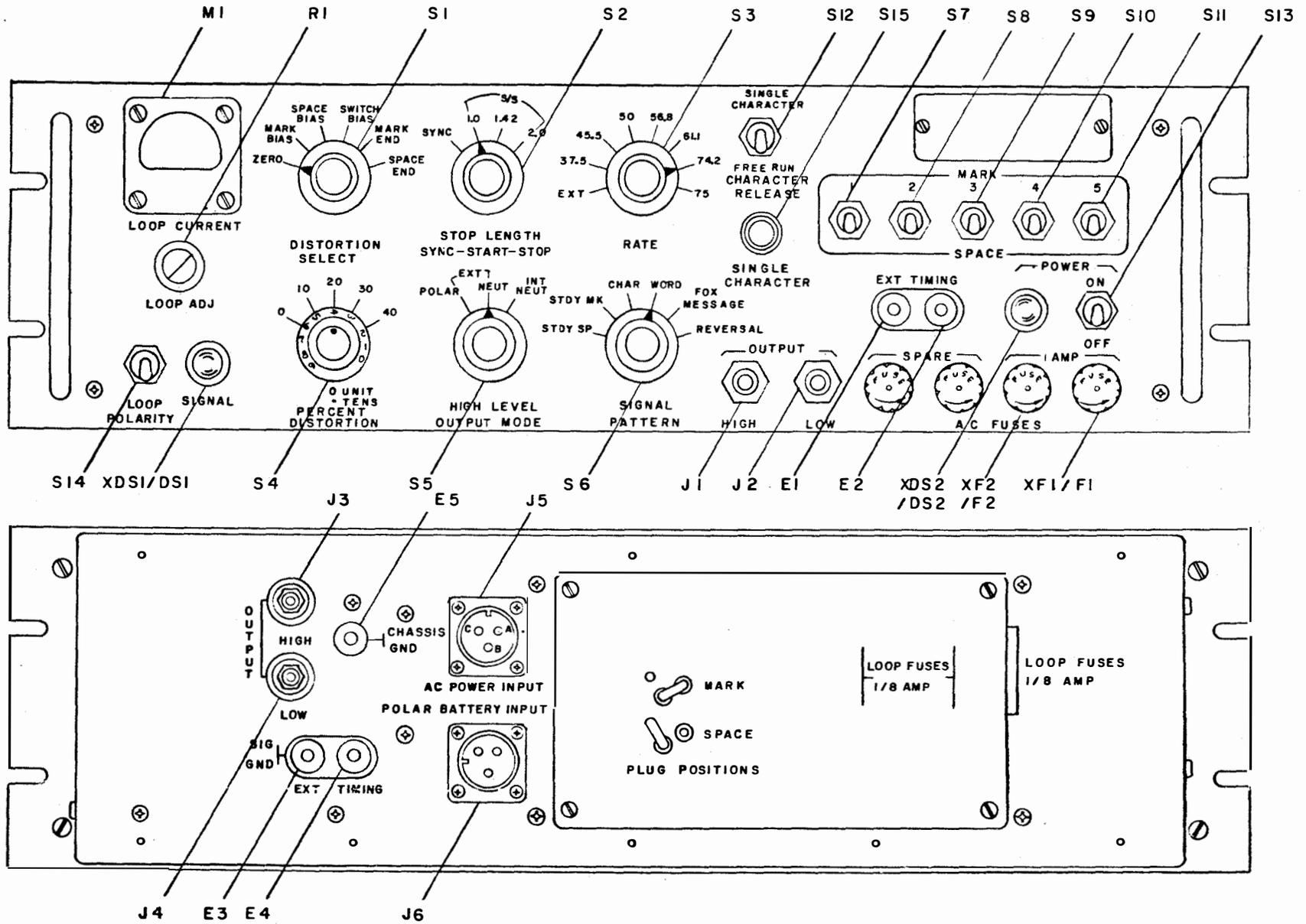
Figure 3-3. Signal Generator Controls and Indicators
