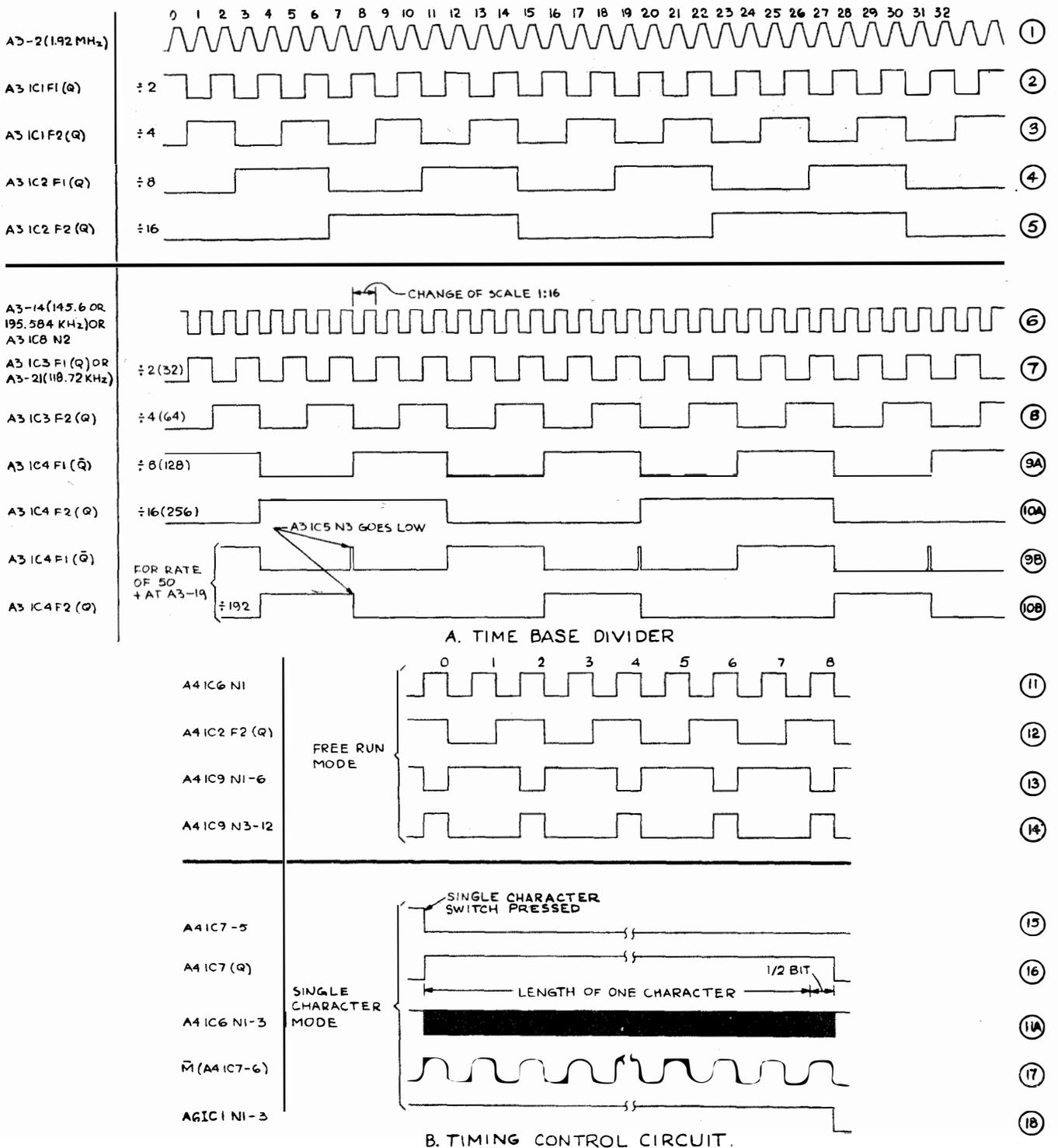
Figure 4-10. Signal Generator Timing Diagrams (Sheet 1 of 9)
