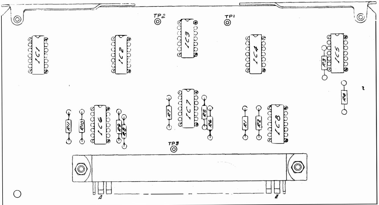
Figure 5-5. Time Base Divider Board 1A1A3 Component Location
