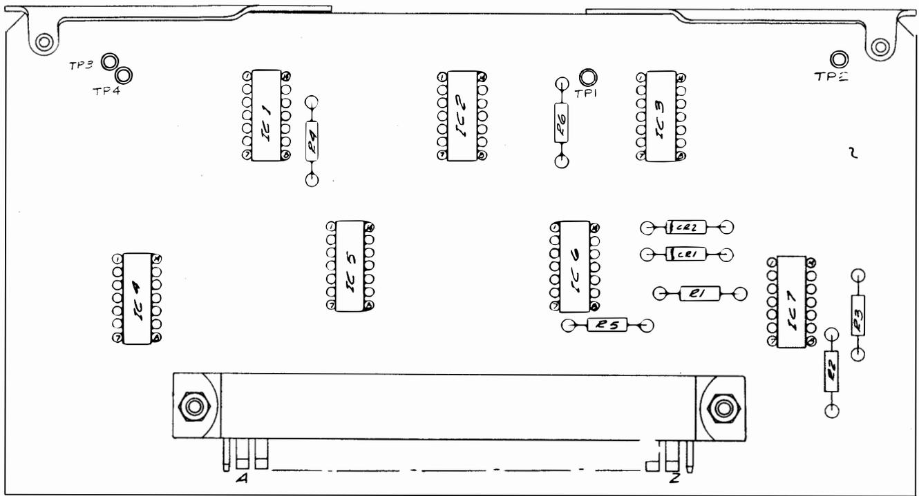
Figure 5-11. Stop Mark Trigger Board 1A1A6 Component Location
