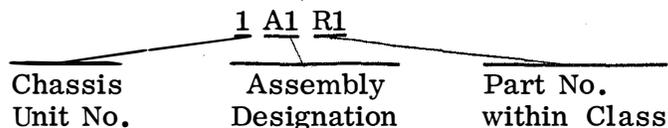
Read as: First (1) resistor (R) of first (1) assembly (A) of chassis unit (1)
