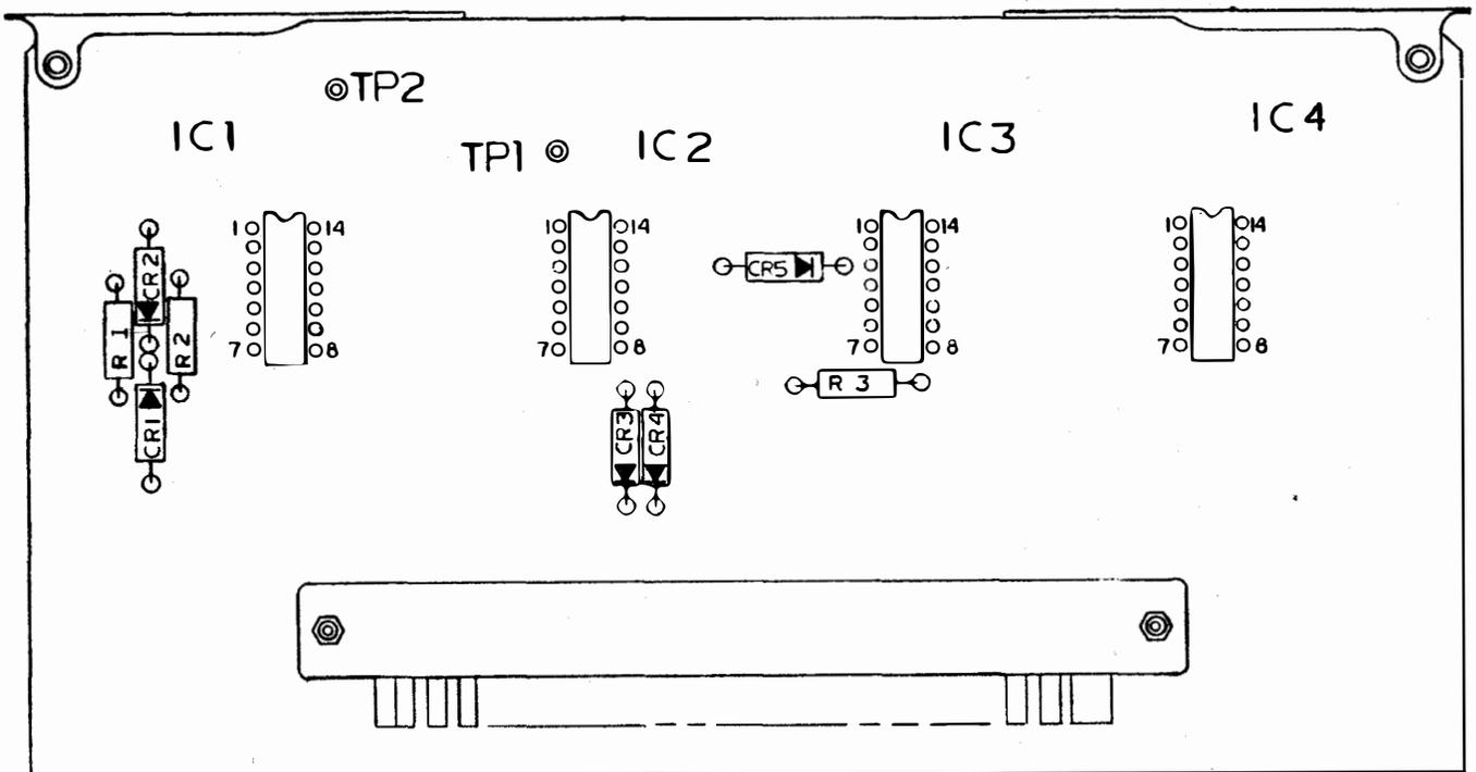
Figure 5-35. Word Matrix Control and Carriage Return 1A1A17 Component Location
