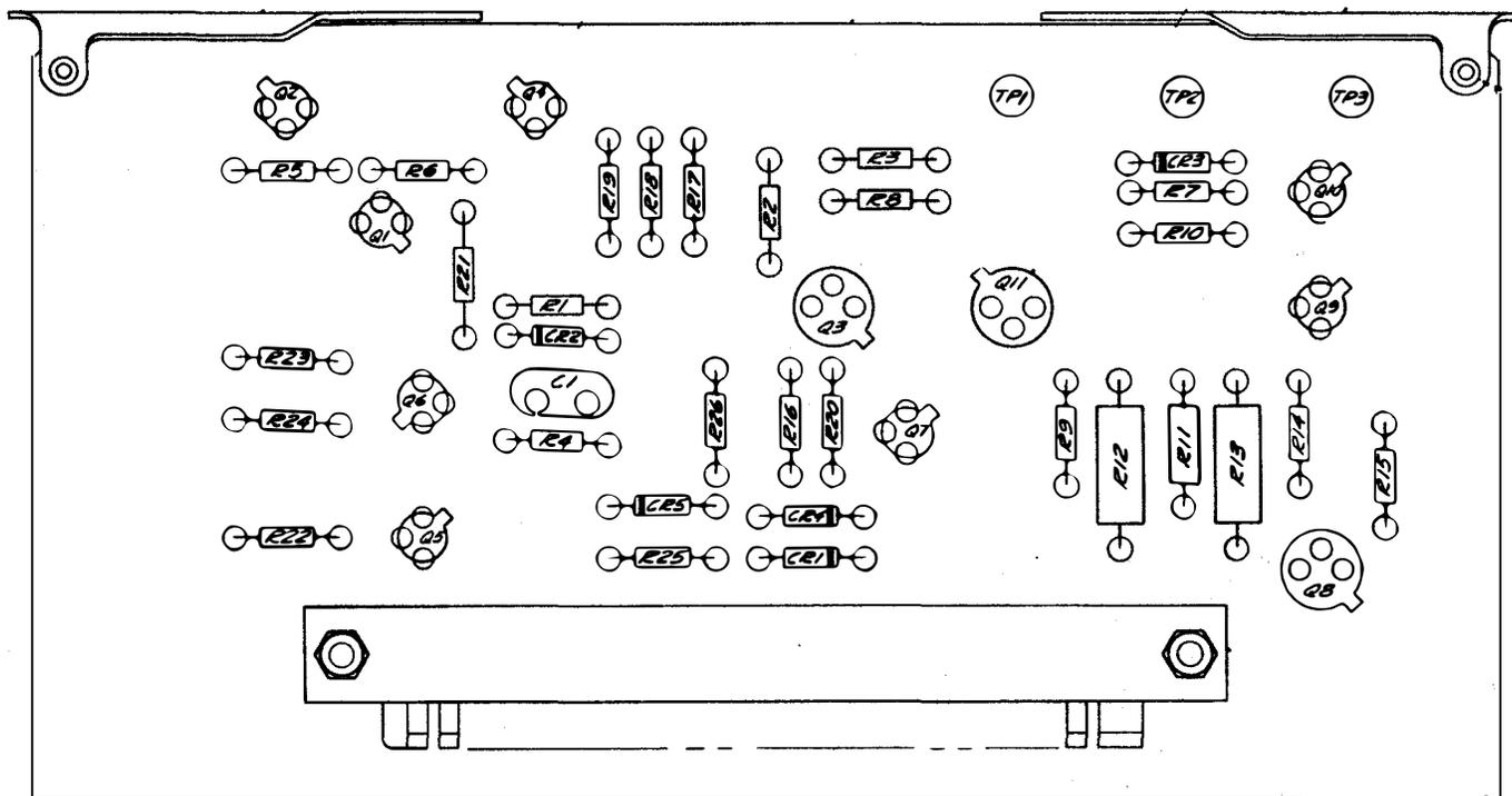
Figure 5-33. Output Driver 1A1A16 Component Location
