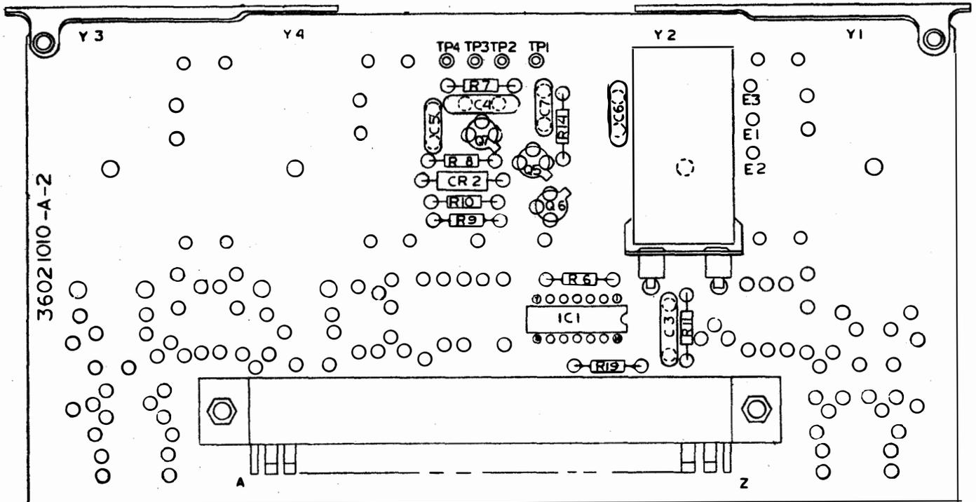
Figure 5-1. Oscillator Board 1A1A1 Component Location
