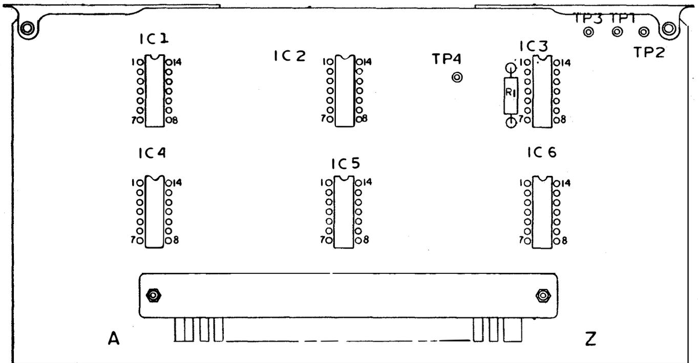
Figure 5-17. Character Counter II Board 1A1A9 Component Location
