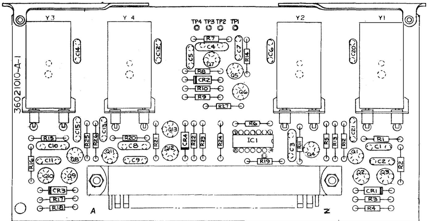
Figure 5-3. Oscillator Board 1A1A2, Component Location
