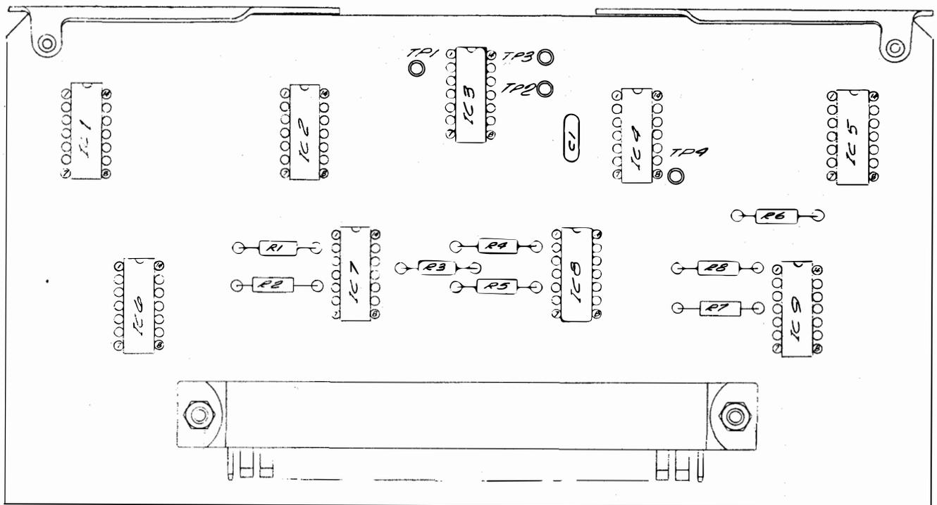
Figure 5-9. BCD Counter and Trigger I Board 1A1A5 Component Location
