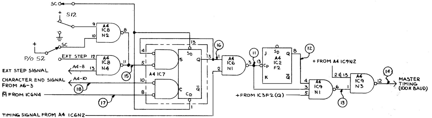
Figure 4-3. Timing Control Circuits, Simplified Schematic
