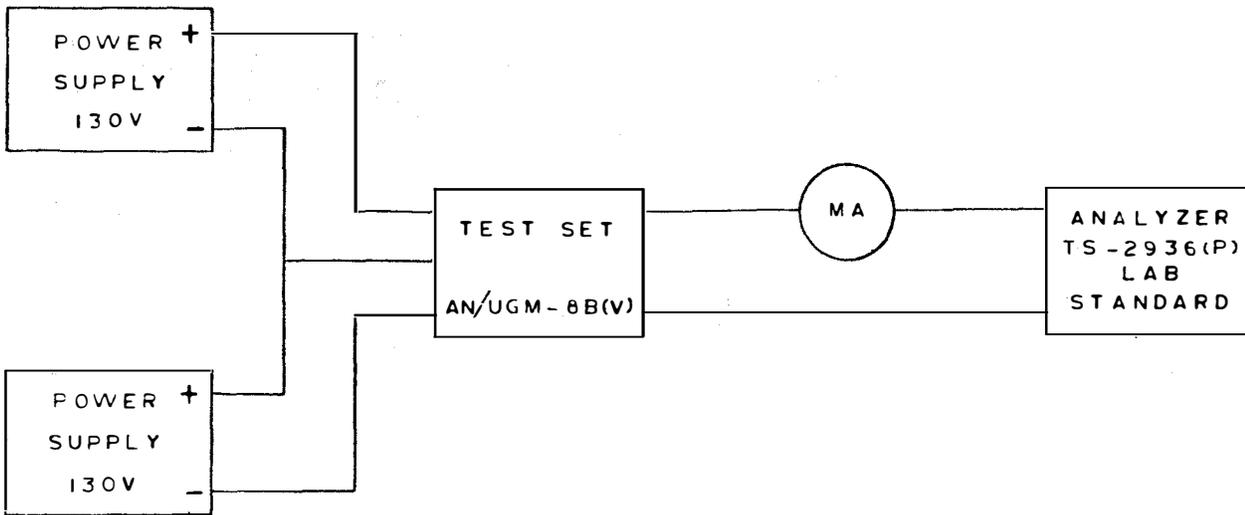
Figure 4-13. Test Setup, High Level Polar
