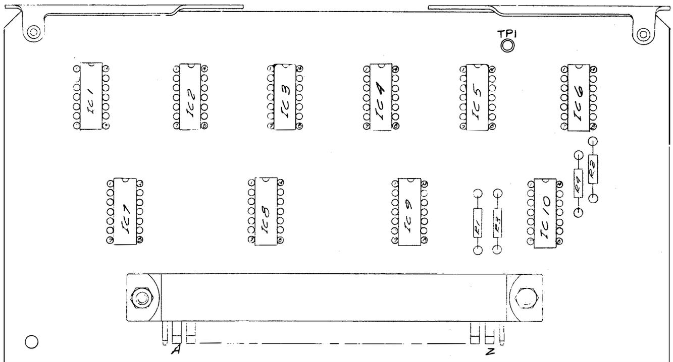
Figure 5-19. Bit Counter and Gates Board 1A1A10 Component Location
