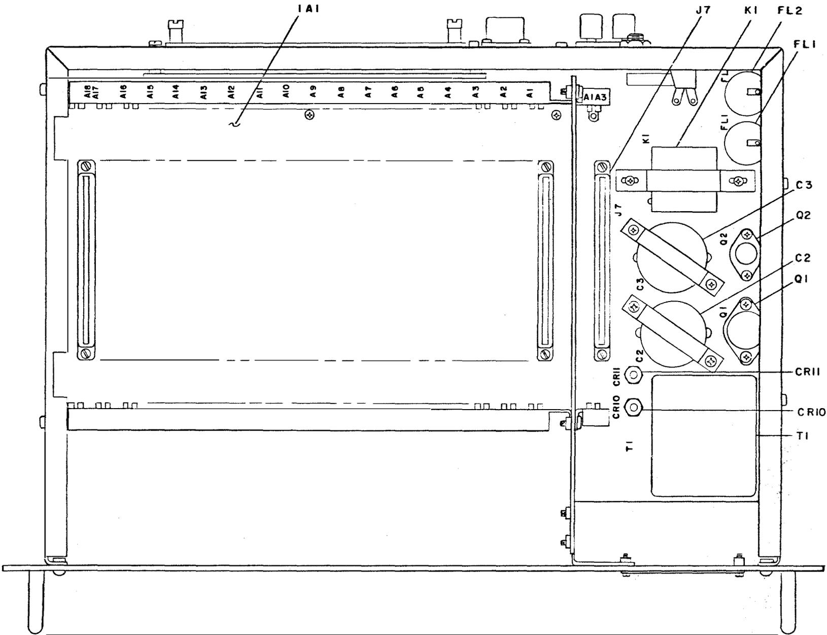
Figure 5-41. Chassis Mounted Components Location (Sheet 1 of 2)
