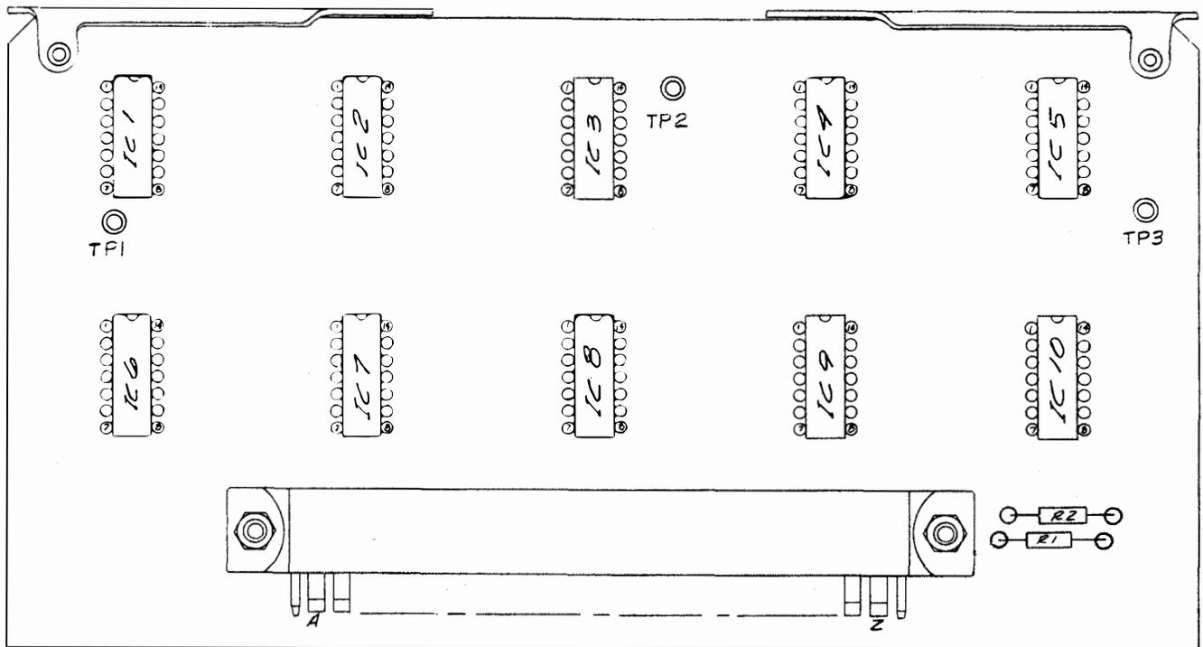
Figure 5-29. Character Counter I Board 1A1A14 Component Location
