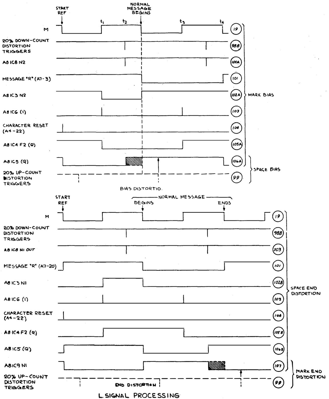
Figure 4-10. Signal Generator Timing Diagrams (Sheet 9 of 9)
