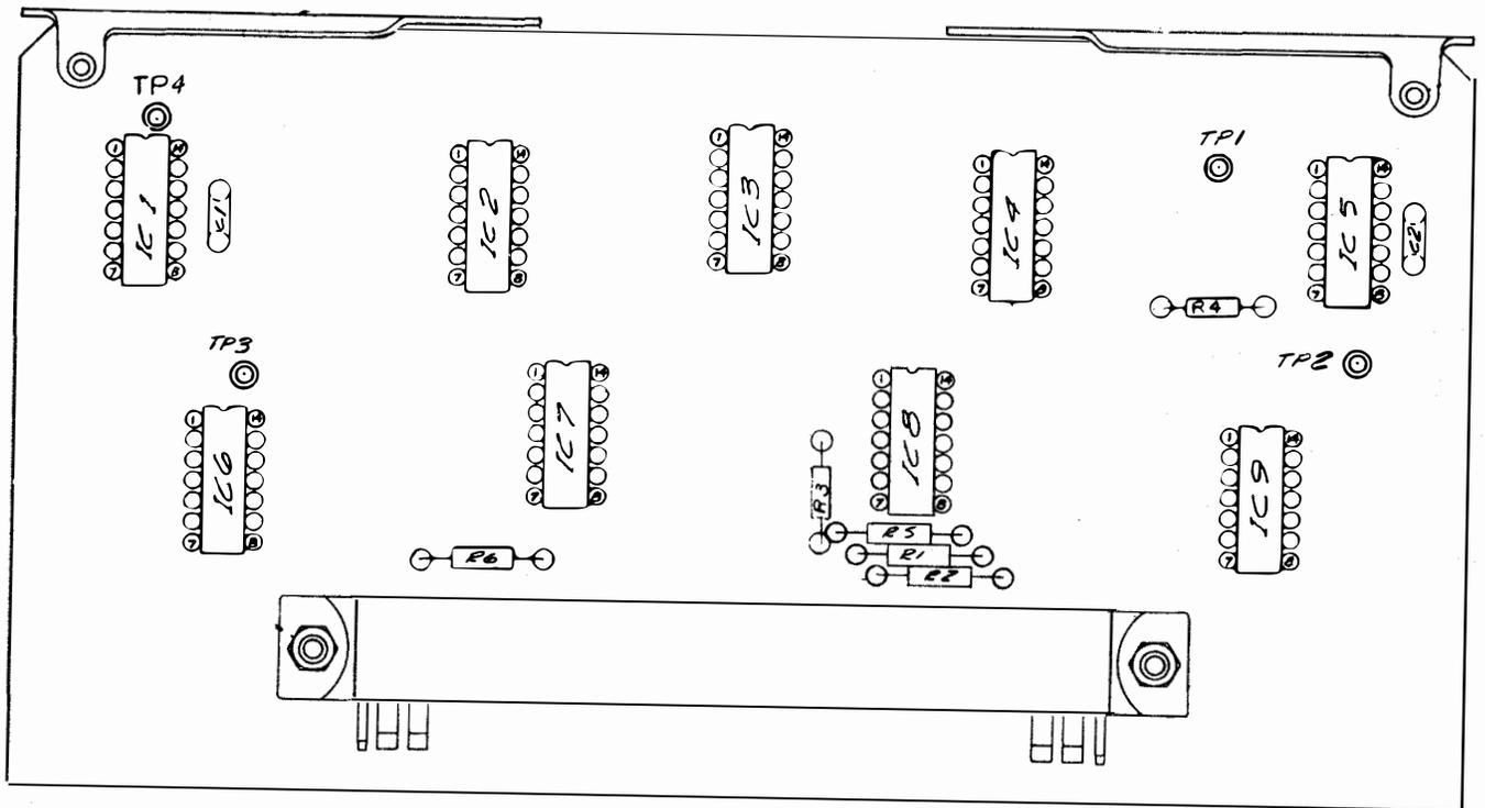
Figure 5-7. Timing Control Board 1A1A4 Component Location
