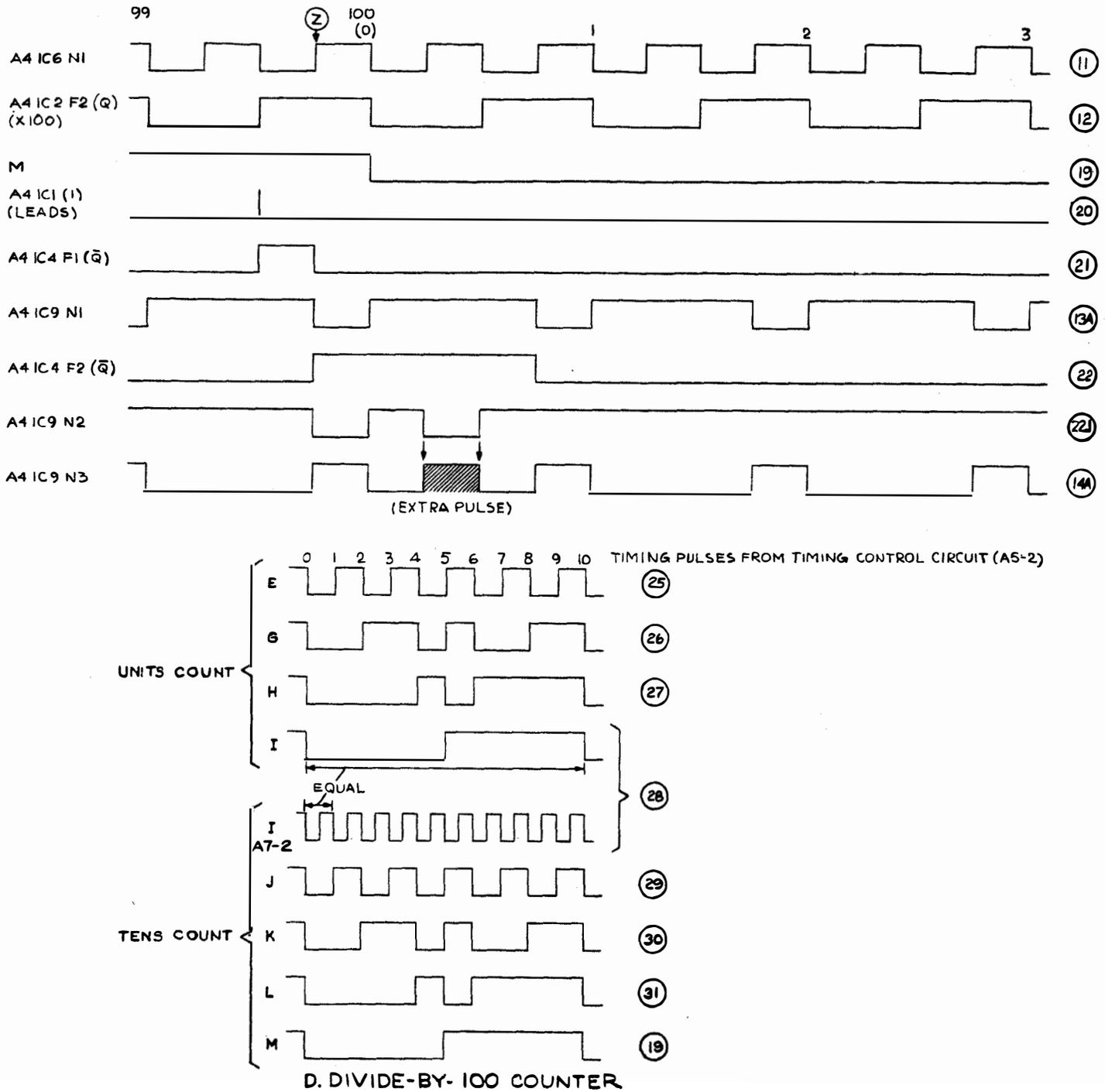
Figure 4-10. Signal Generator Timing Diagrams (Sheet 2 of 9)
