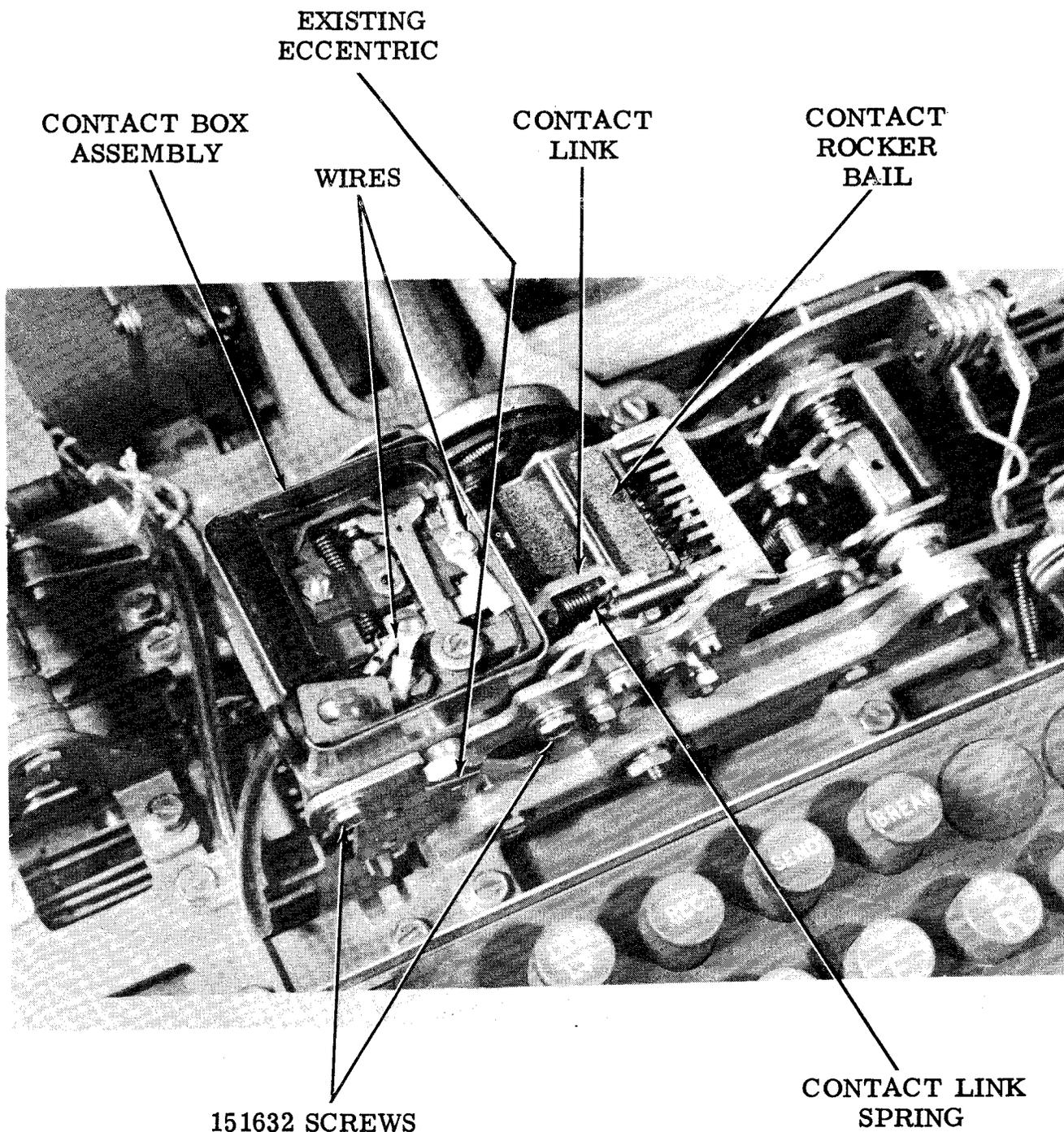
Figure 8 - Keyboard (LAK) Showing Signal Generator
