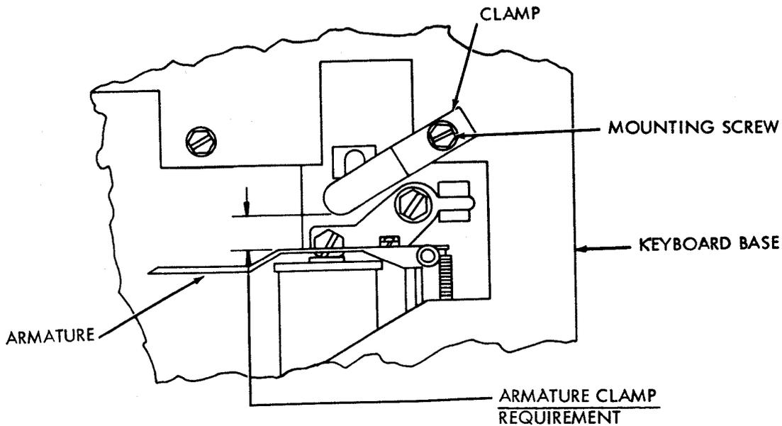
NOTE: TO MAKE KEYBOARD OPERABLE WITHOUT ELECTRICAL PULSE TO OPERATE STEPPING MAGNET LOOSEN CLAMP MOUNTING SCREW AND ROTATE CLAMP COUNTERCLOCKWISE TO HOLD THE ARMATURE IN THE OPERATING POSITION. MAINTAIN 0.005 INCH TO 0.015 INCH CLEARANCE BETWEEN CLUTCH TRIP BAR AND ARMATURE LEVER.
