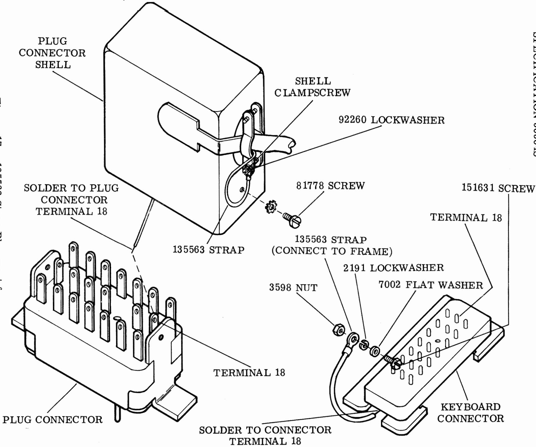
Figure 18 - Magnet and Contact Assembly Wiring
