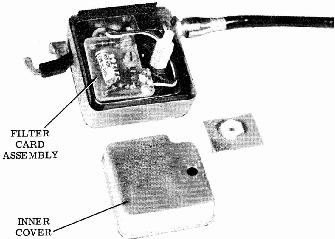
Figure 4 - Typical Signal Generator with Inner Cover Removed
