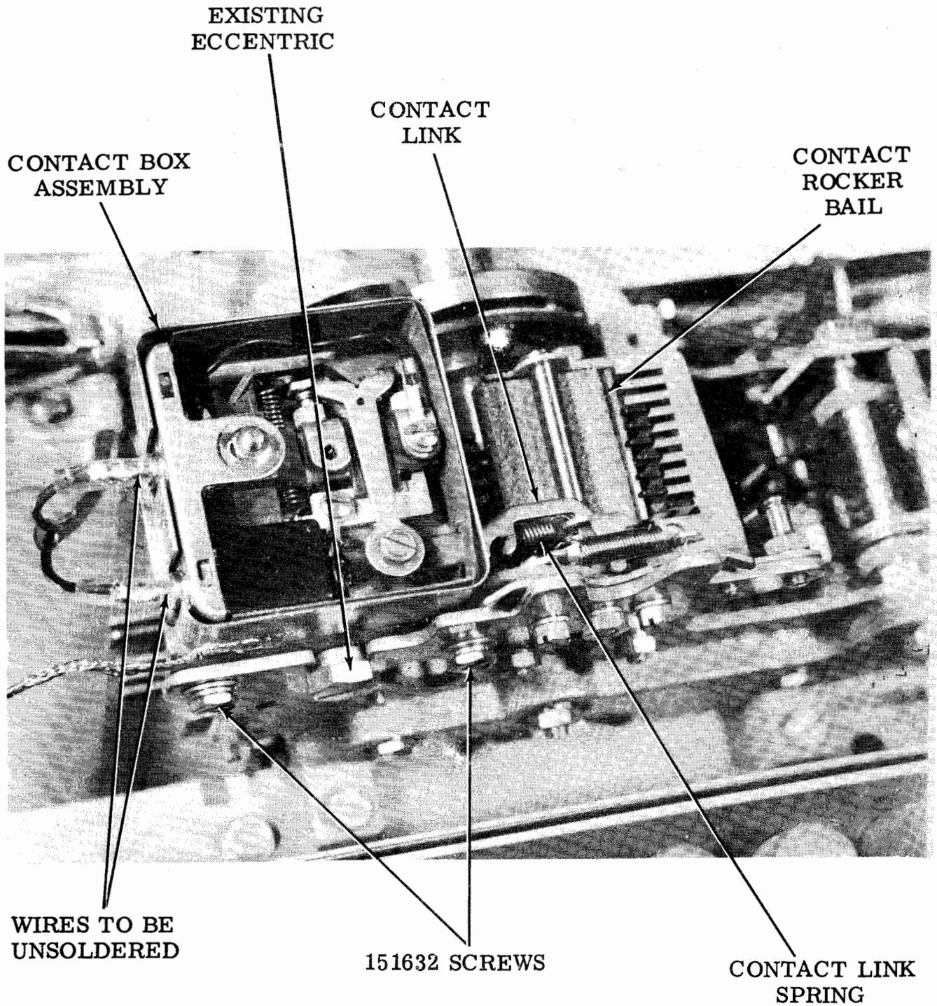
Figure 13 - Keyboard (LK) Showing Signal Generator
