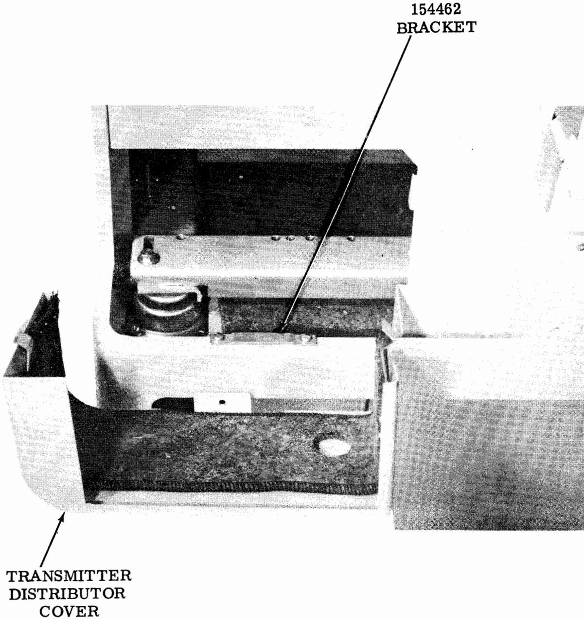
Figure 7 - Cabinet (ASR) Showing Transmitter Distributor Cover Removed
