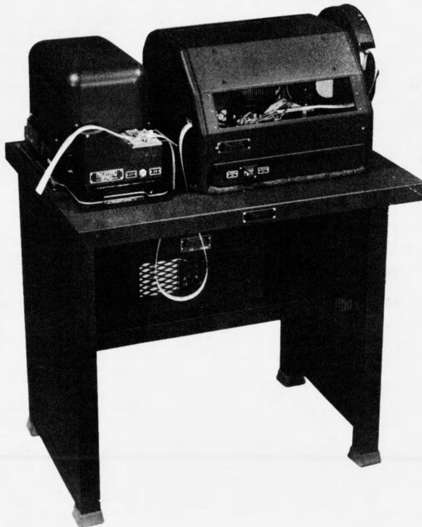
**TELETYPE MODEL 14 RECEIVING-ONLY TYPING REPERFORATOR
