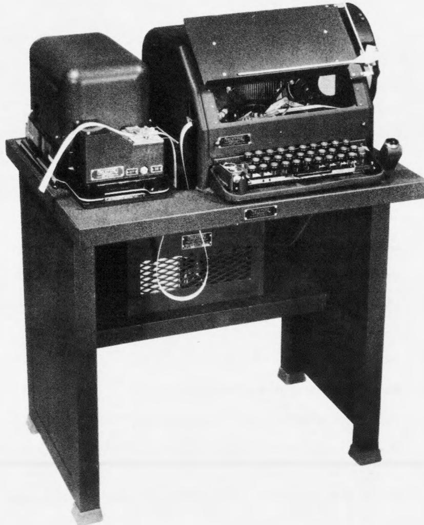
**TELETYPE MODEL 14 SENDING-RECEIVING TYPING REPERFORATOR
