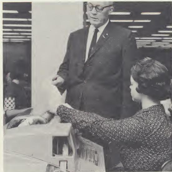
Claude M. Janes, manager, Procedures Research and Data Processing Division, observes data coming in from Marathon's distribution terminals. Data is received on a Teletype Model 35 ASR (automatic send-receive) set in page copy and punched paper tape form. Page copy is checked for any apparent errors, with the tape later being read into computers to prepare an assortment of documents and reports.
