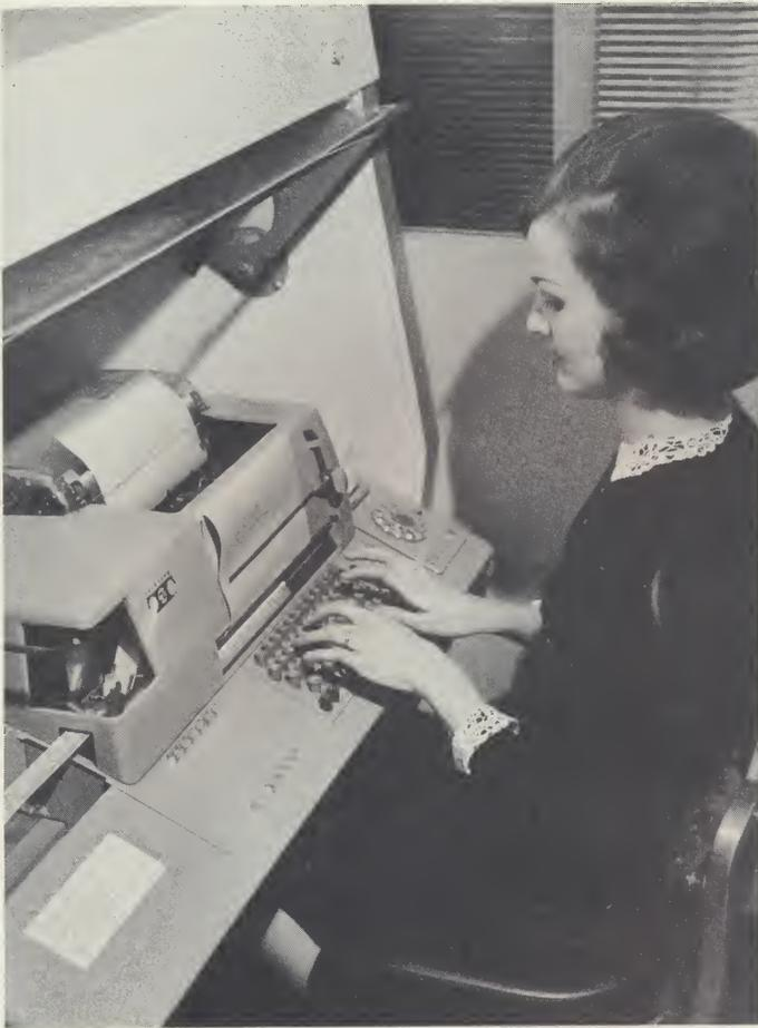
Each computer program developed at the Applied Mathematics Laboratory is punched into paper tape by the operator of a Teletype Model 35 ASR (automatic send-receive) set, as demonstrated by Mrs. Betty Hall, computer programmer. Tapes are then stored until an engineer or scientist has application for a particular one, at which time the tape is inserted into the ASR set's tape reader and transmitted to the computer.
