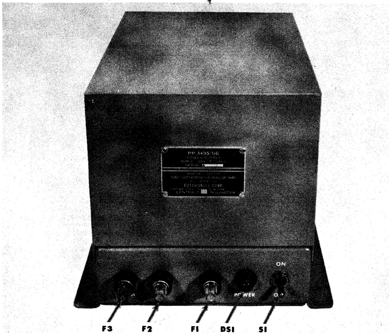
Figure 3-1. Power Supply PP-3495/UG, Front View
