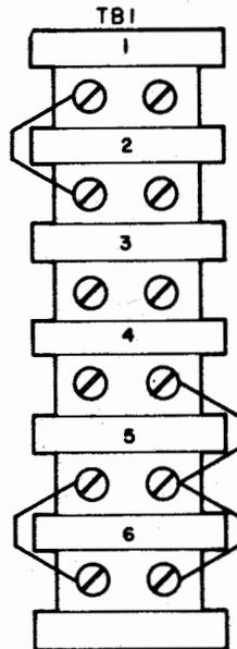
Figure 2-2. Terminal Board Connection 48-Volt Output
