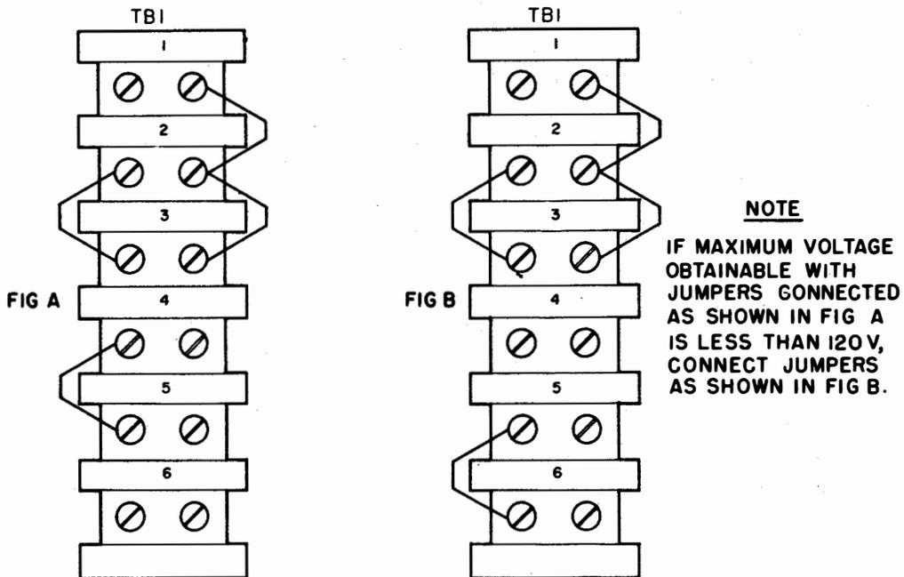
Figure 2-3. Terminal Board Connections 120-Volt Output
