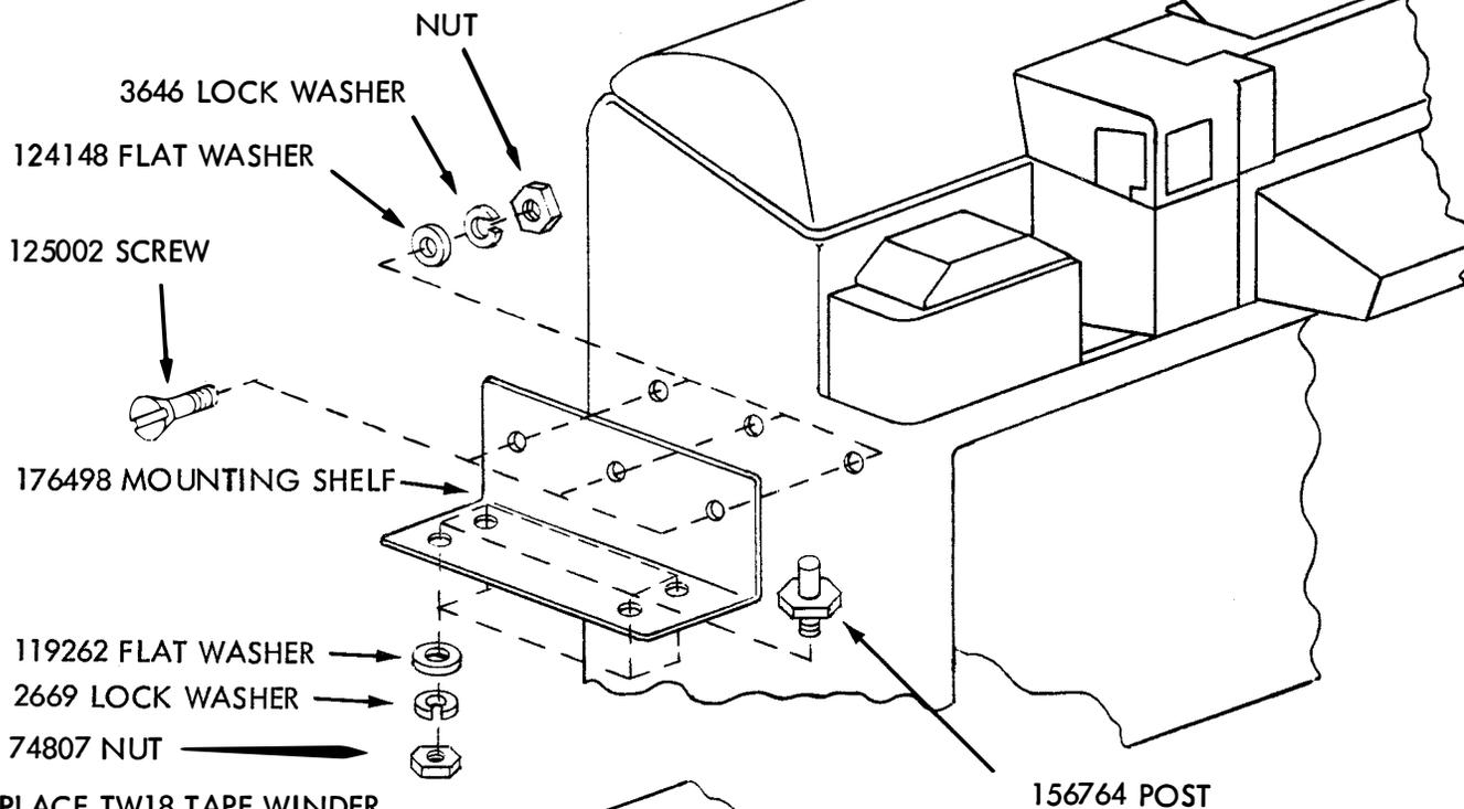
PLACE TW18 TAPE WINDER WITH ENCLOSURE OVER 156764 POSTS
