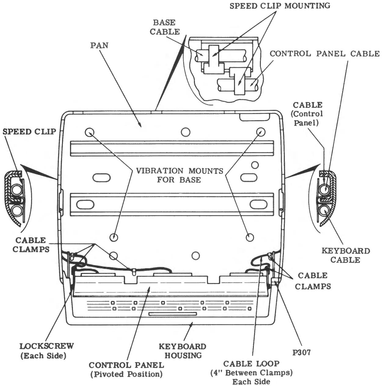
Figure 9 - Pan Cable Routing
