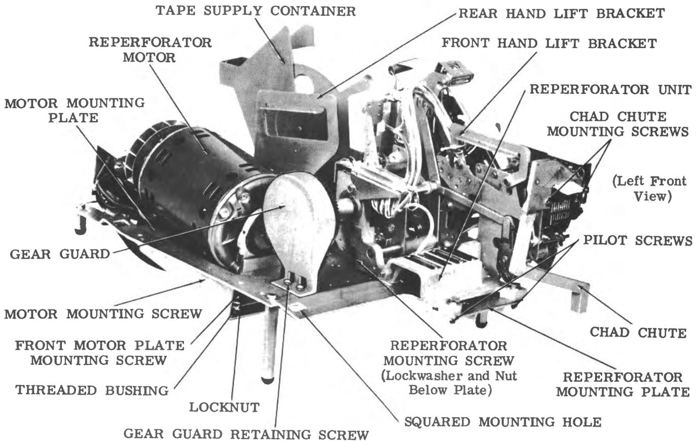
Figure 18 - Reperforator, Mounting Plate, and Motor
