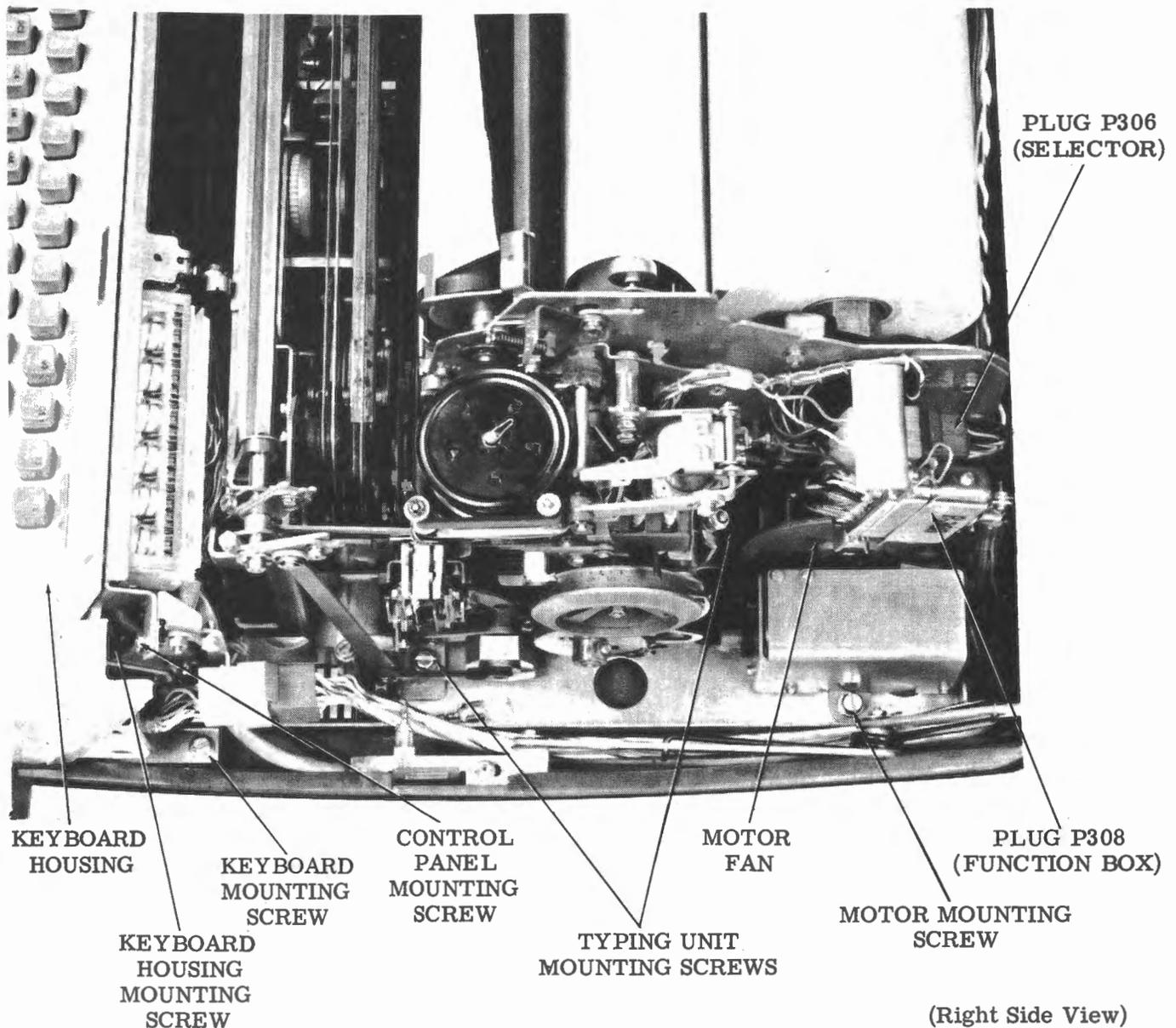
Figure 3 - Typing Unit and Control Panel
