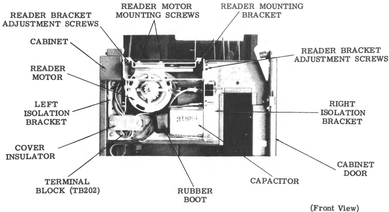
Figure 20 - Reader Motor Removal
