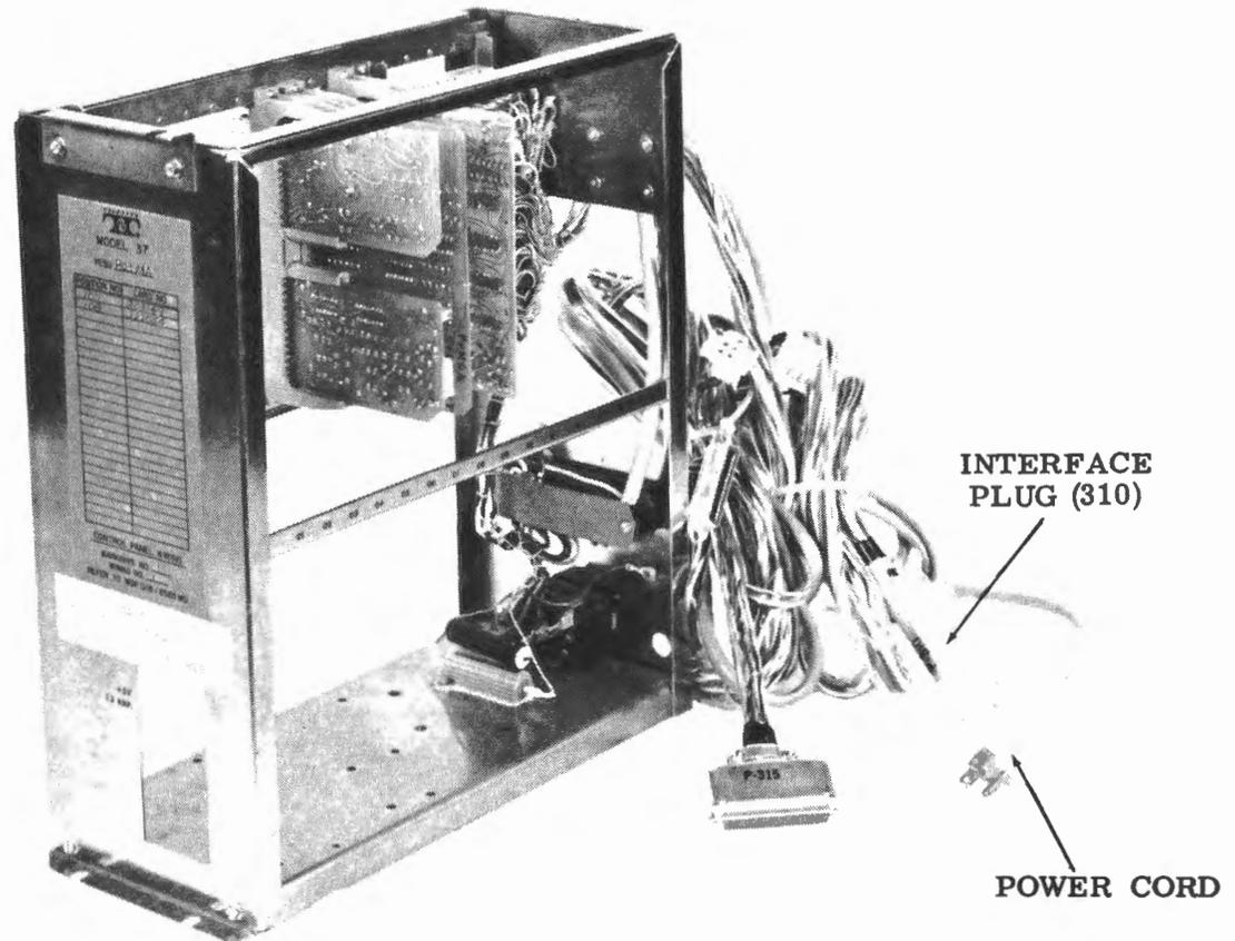
Figure 23 - 37 Tape Module Electrical Service Unit
