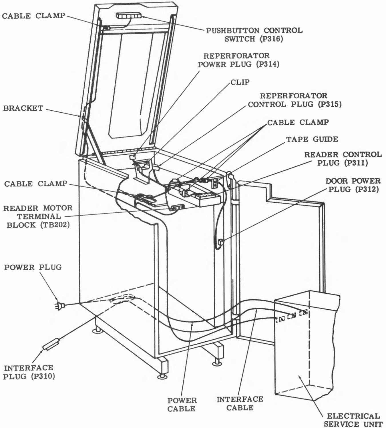
Figure 22 - Tape Module Cable Routing
