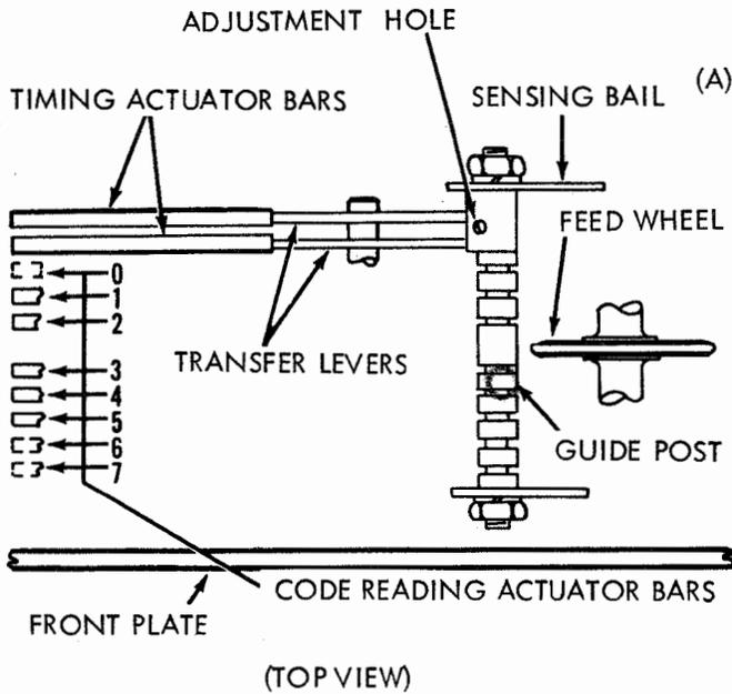
(A) TIMING (UNIVERSAL) CONTACT ACTUATOR REQUIREMENT
