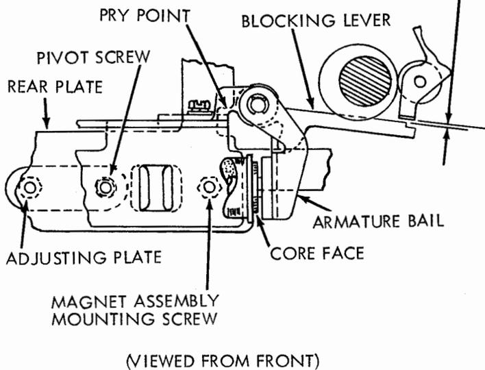
ADJUSTMENTS (D), (E) AND (F-2) APPLY TO TRANSFER TYPE CONTACT ASSEMBLIES ONLY; ALL OTHER ADJUSTMENTS APPLY TO BOTH TRANSFER TYPE AND MAKE ONLY TYPE CONTACT ASSEMBLIES. ADJUSTMENTS (A) THROUGH (E) ARE PRELIMINARY. PRELIMINARY ADJUSTMENTS SHOULD BE MADE WITH THE CONTACT ASSEMBLY REMOVED FROM THE READER. FOR EACH ADJUSTMENT, START WITH THE CONTACT PILE-UP FARTHEST FROM THE BENDING TOOL HANDLE TO AVOID DISTURBING COMPLETED ADJUSTMENTS.
