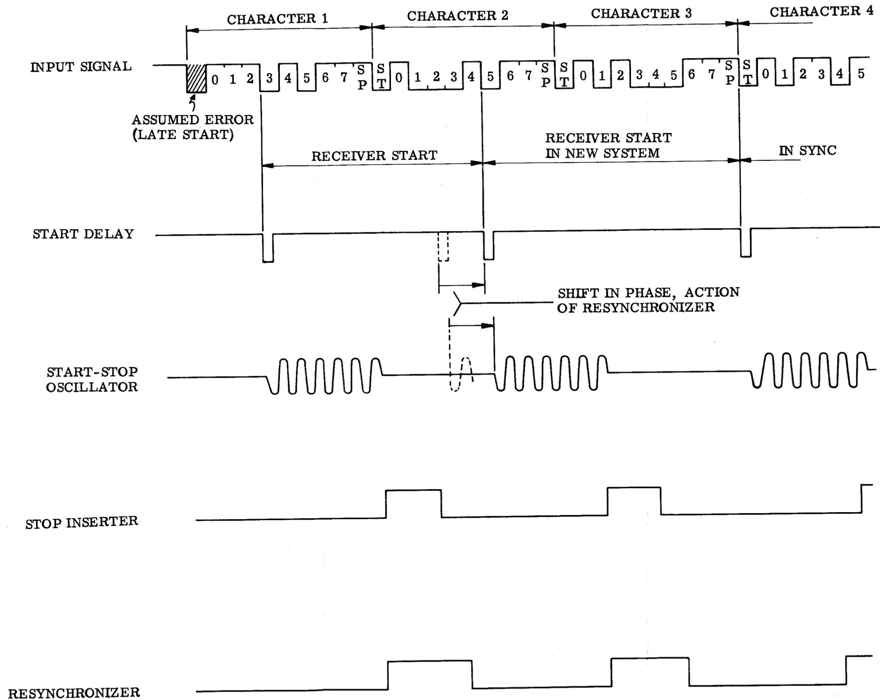
Figure 10 - Resynchronizer Circuit Timing Diagram
