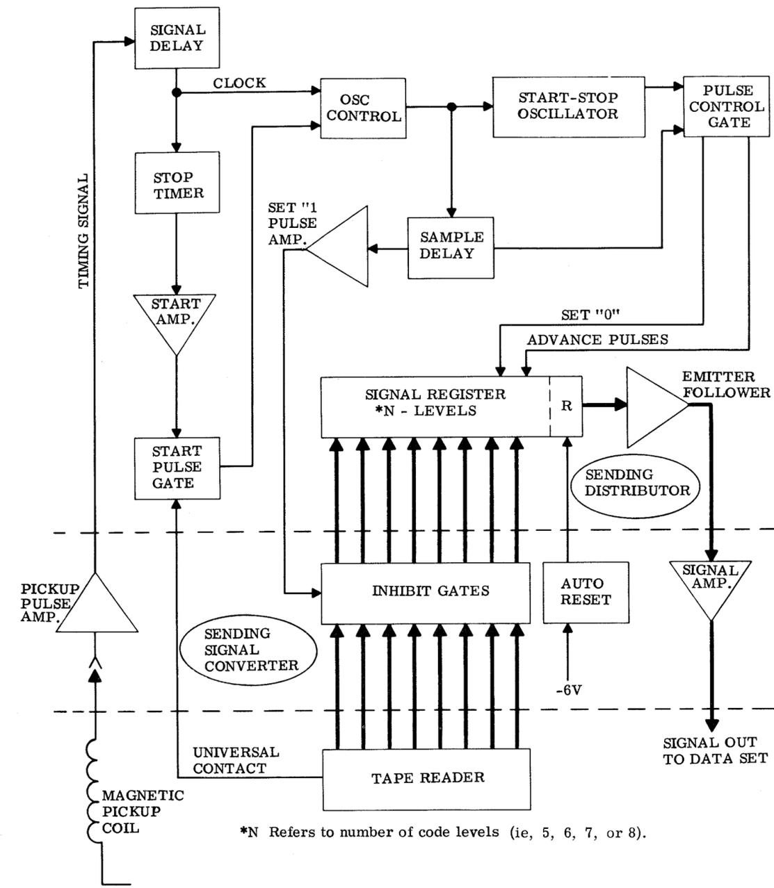
Figure 2 - Tape Sender Block Diagram
