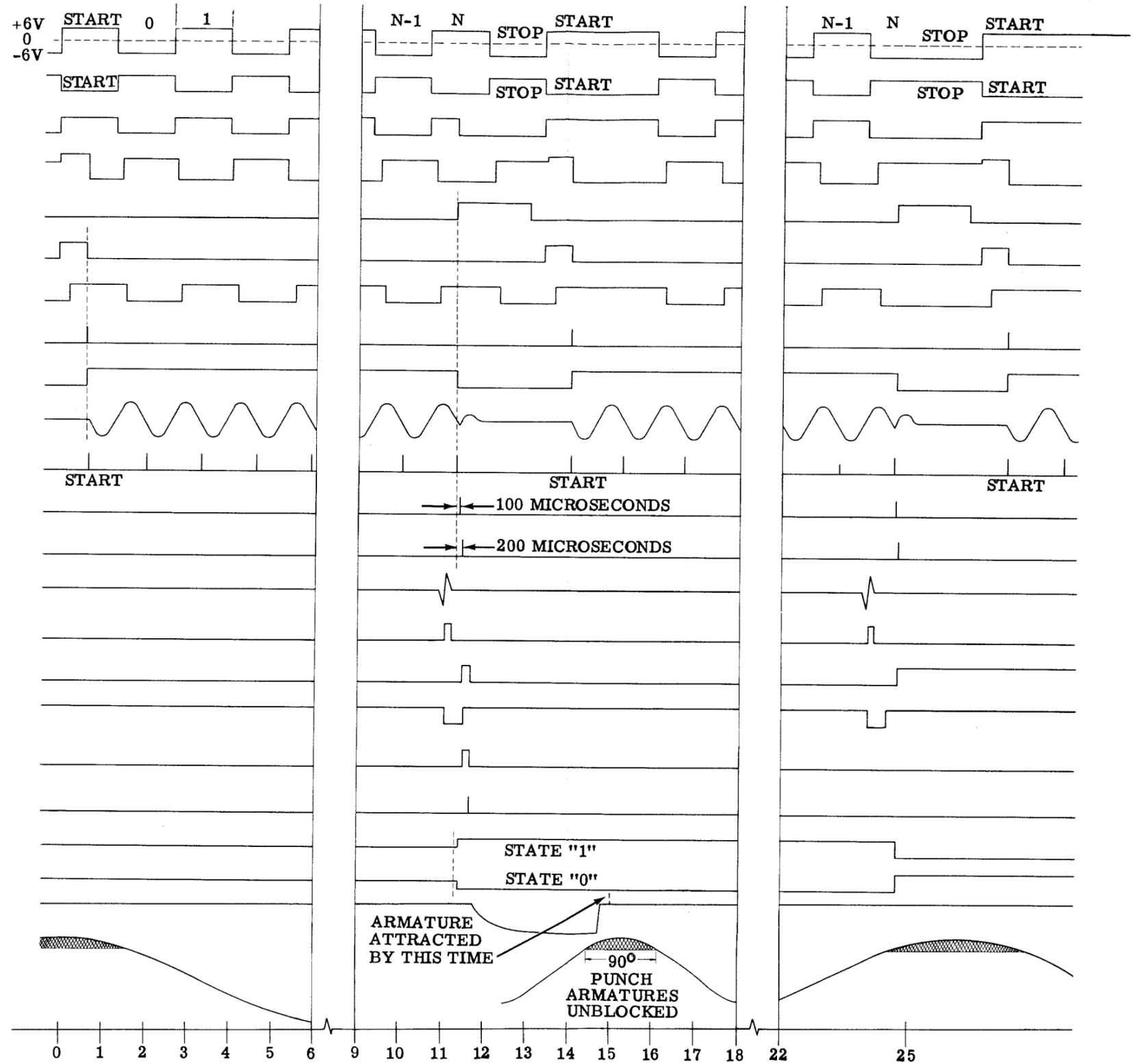
Figure 8 - Tape Receiver Timing Diagram
