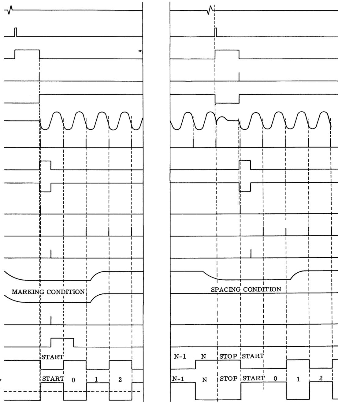
Figure 3 - Tape Sender Timing Diagram
