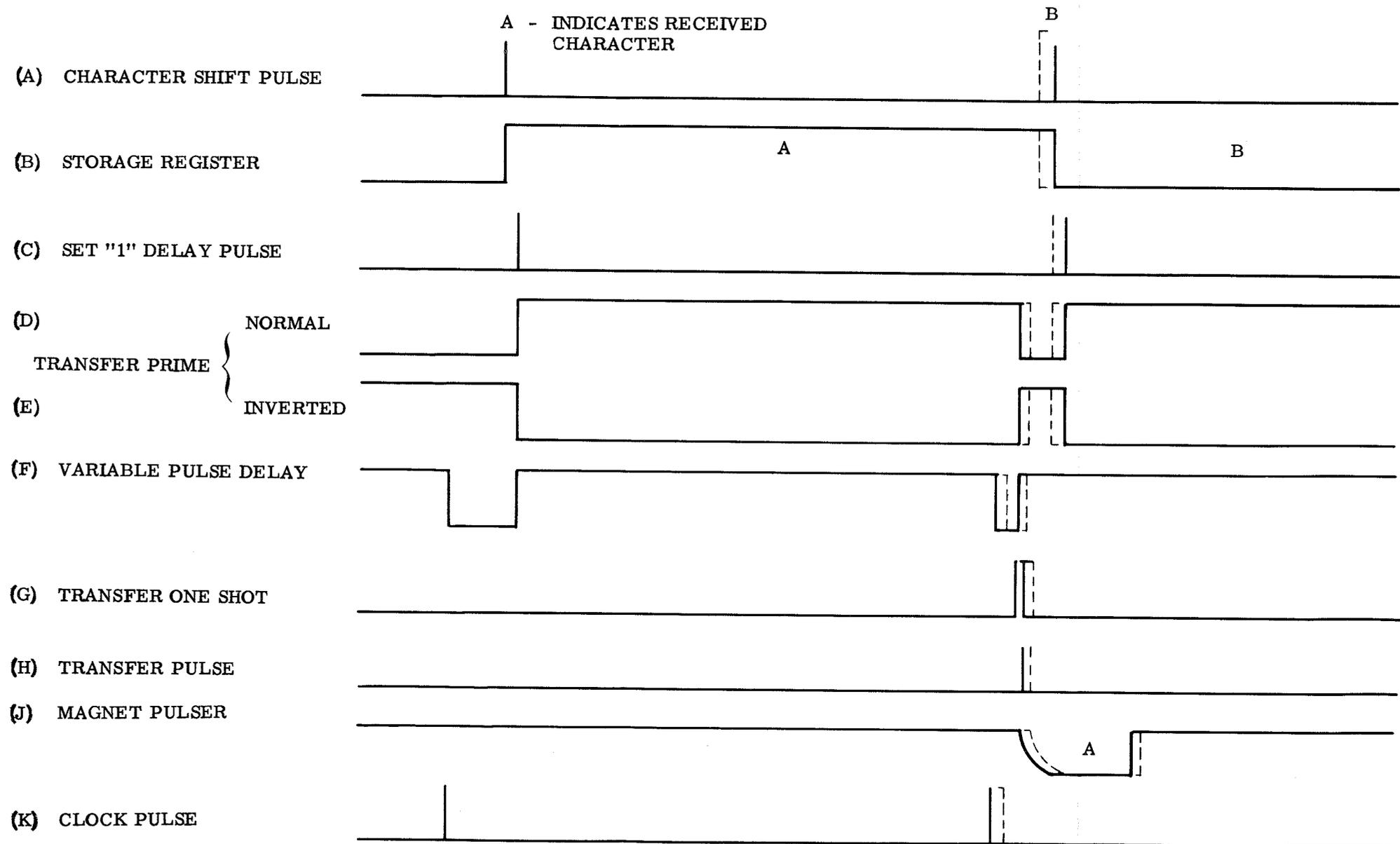
Figure 6 - Transfer Circuitry Timing Diagram,
