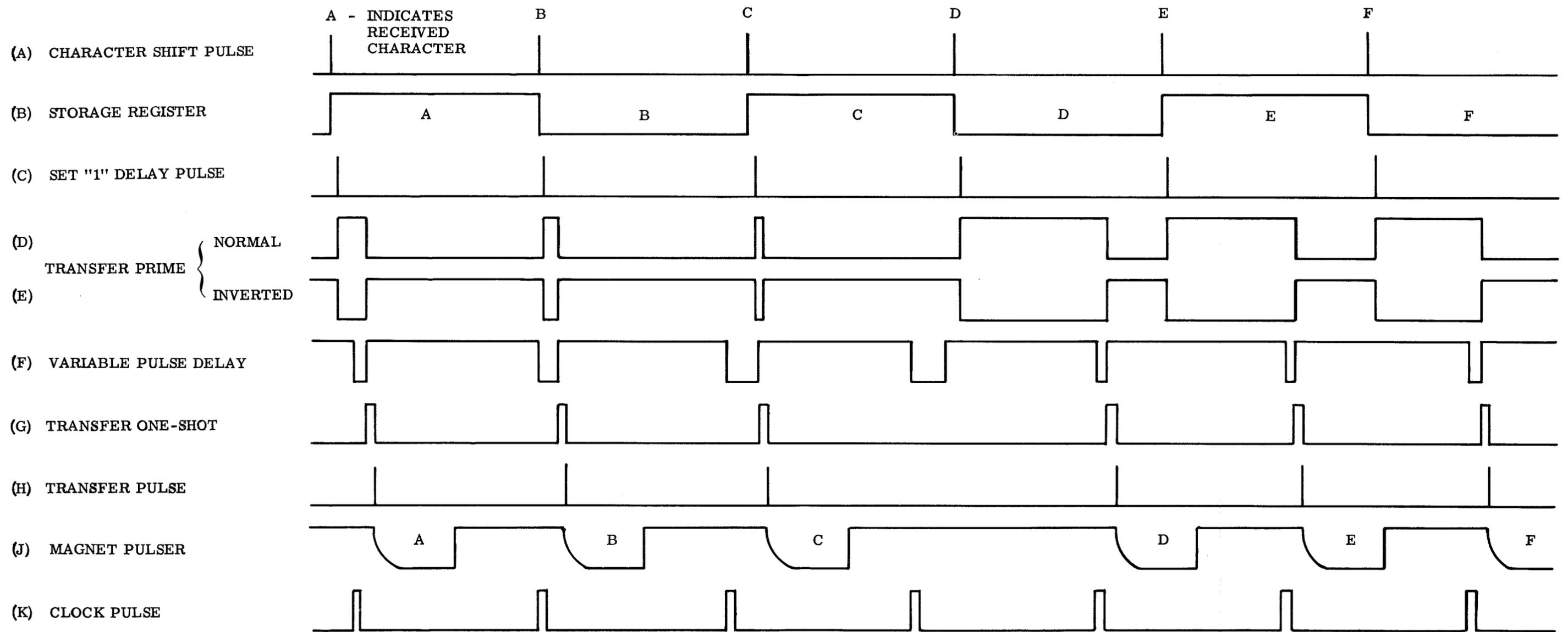
Figure 7 - Transfer Circuitry Timing Diagram, Several Cycles of Operation
