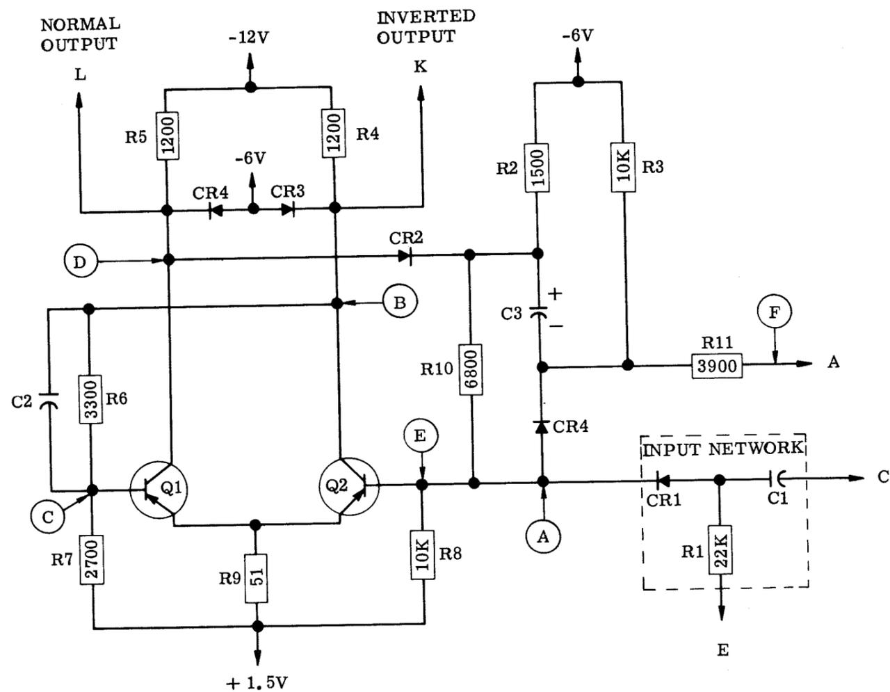
(A) Variable Pulse Delay Circuit
