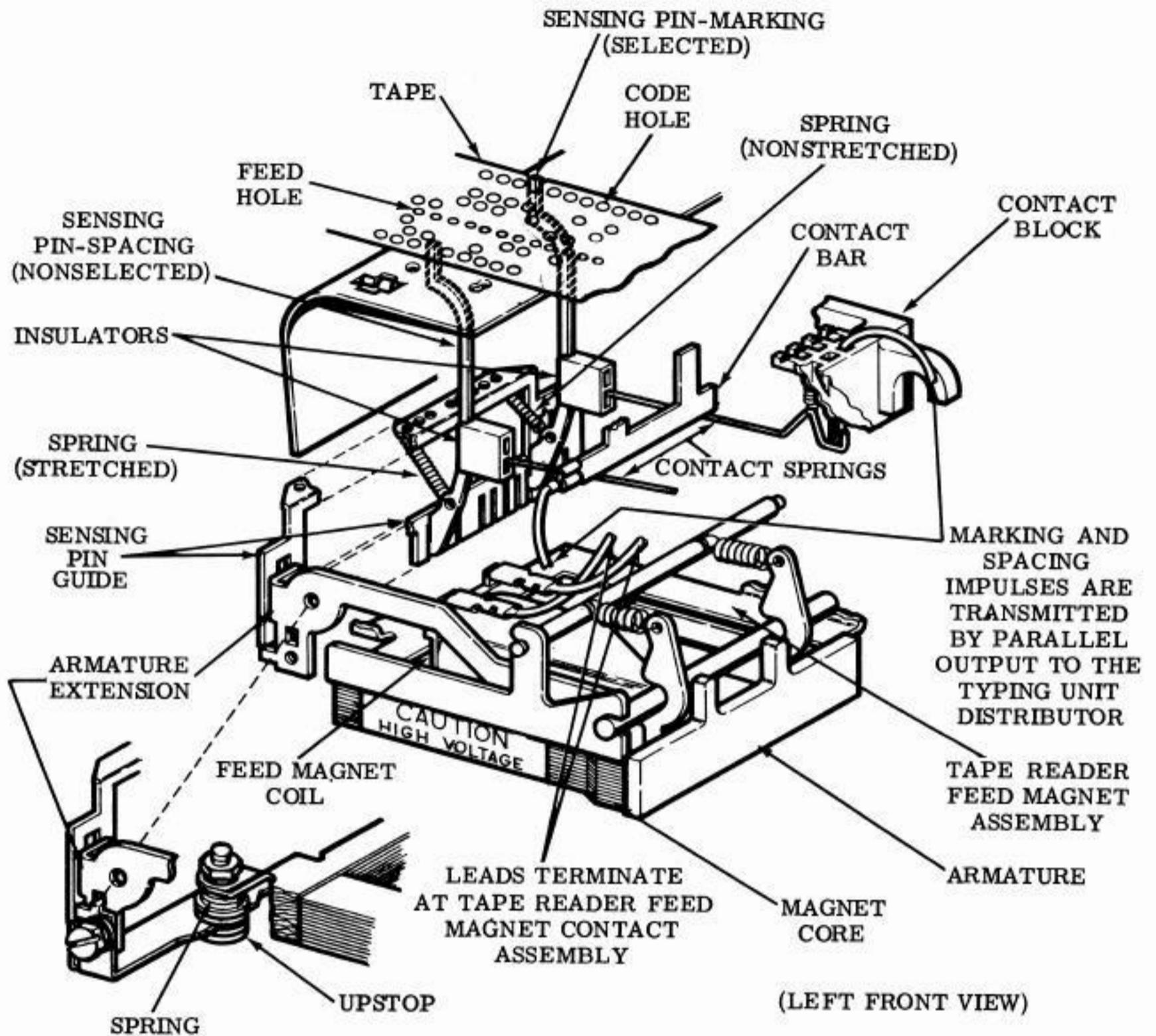
Figure 5 — Feed Magnet and Sensing Mechanism
