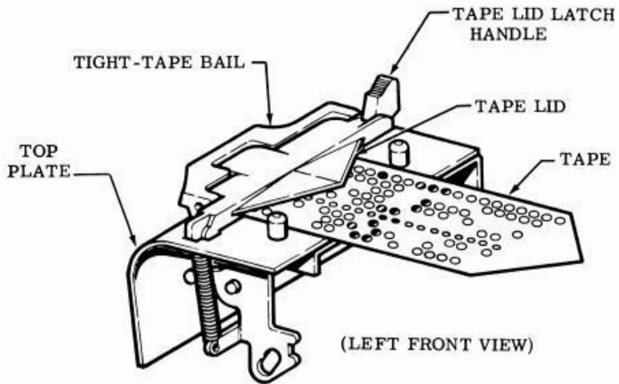
Figure 2 - Tape Lid Mechanism
