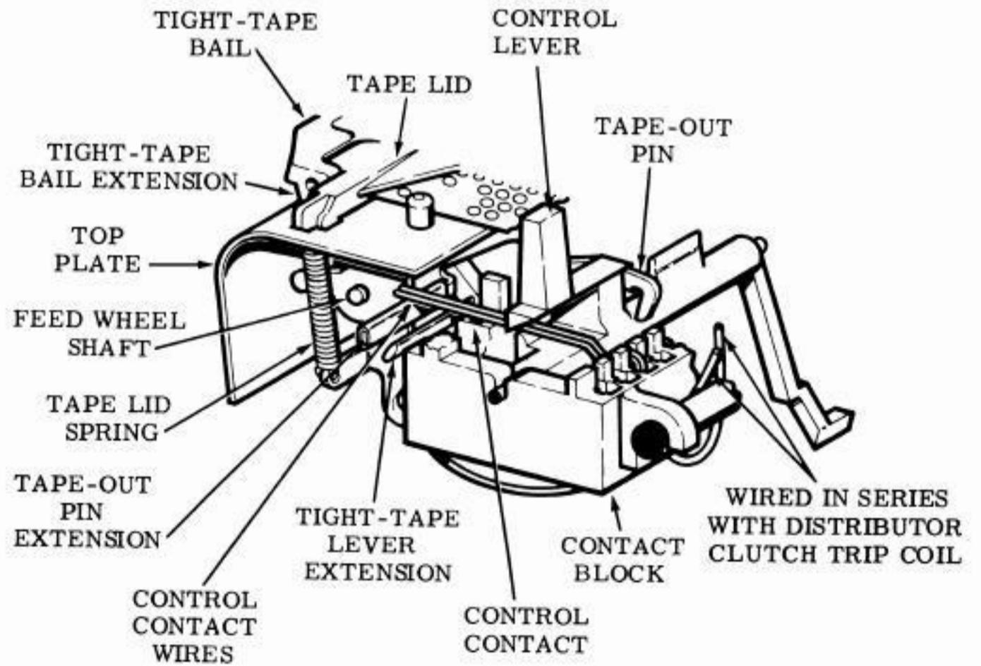
Figure 3 - Control Mechanism
