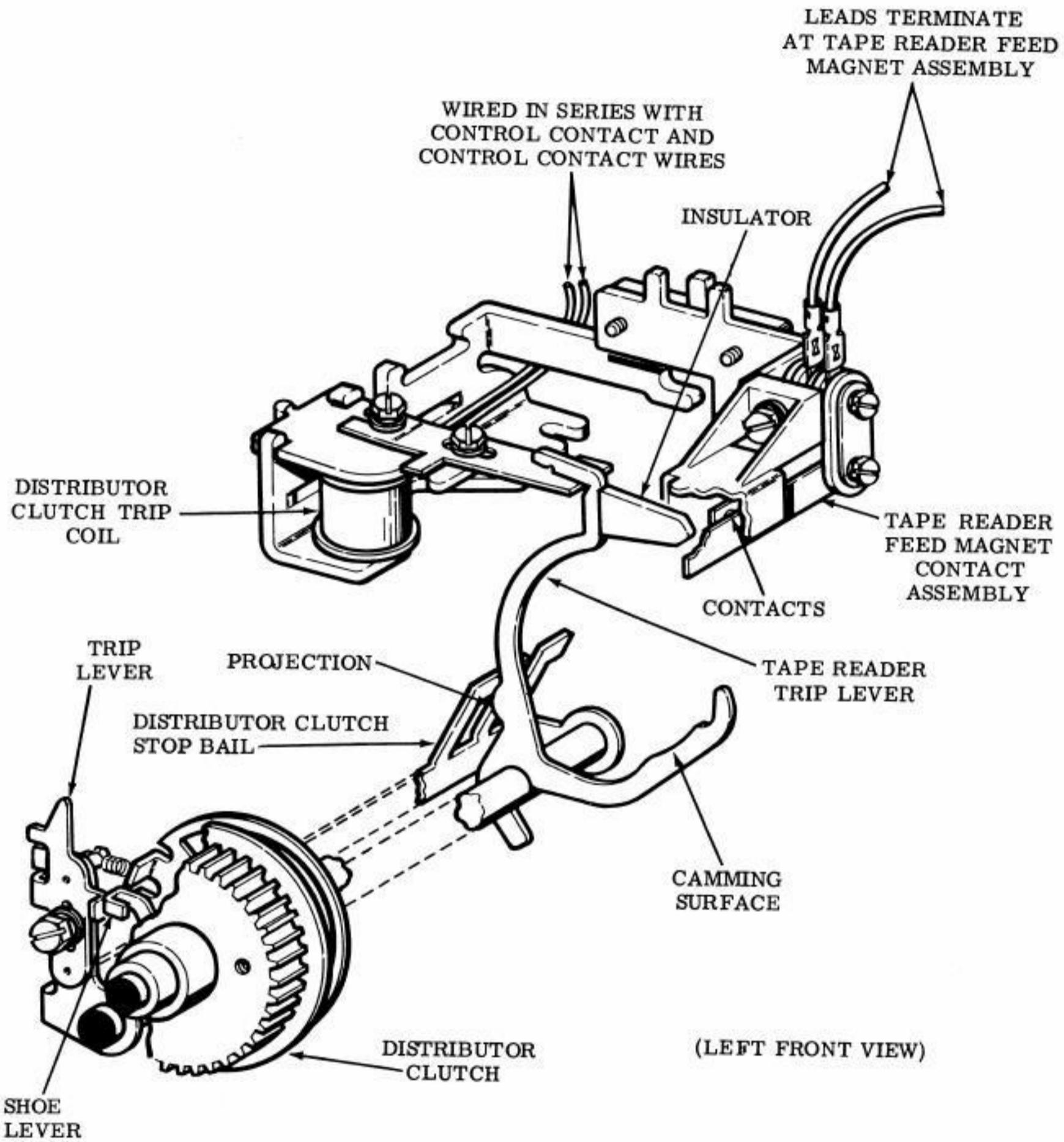
Figure 4 - Distributor Clutch Trip Mechanism
