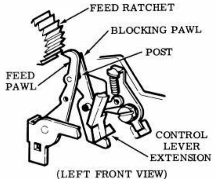
Figure 7 - FREE Position (Tape Feed Mechanism)
