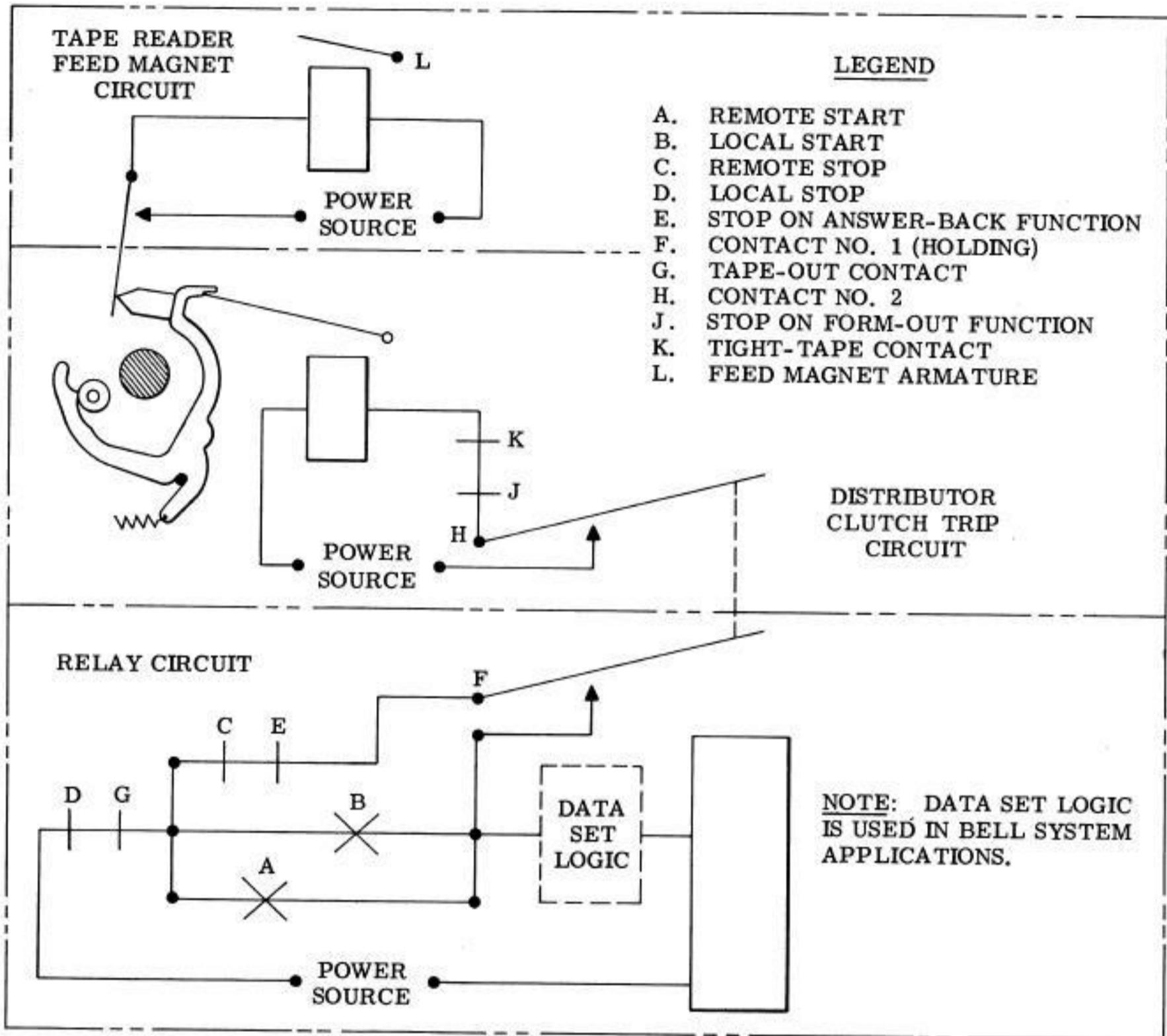
Figure 8 - Automatic Reader Control Schematic
