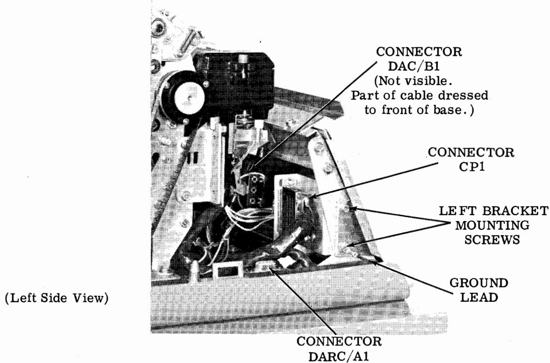
Figure 4 - Control Panel and Base
