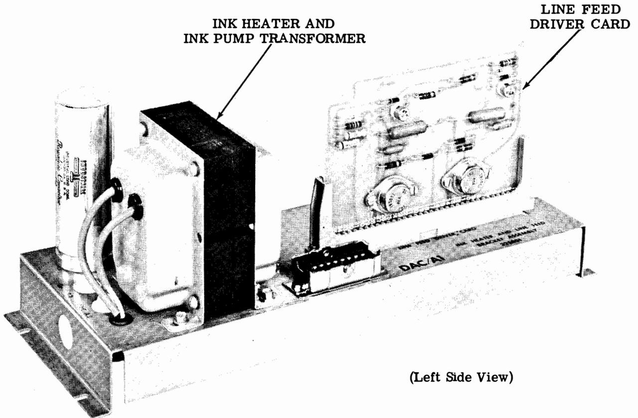
Figure 15 - Ink Heater and Line Feed Bracket Assembly
