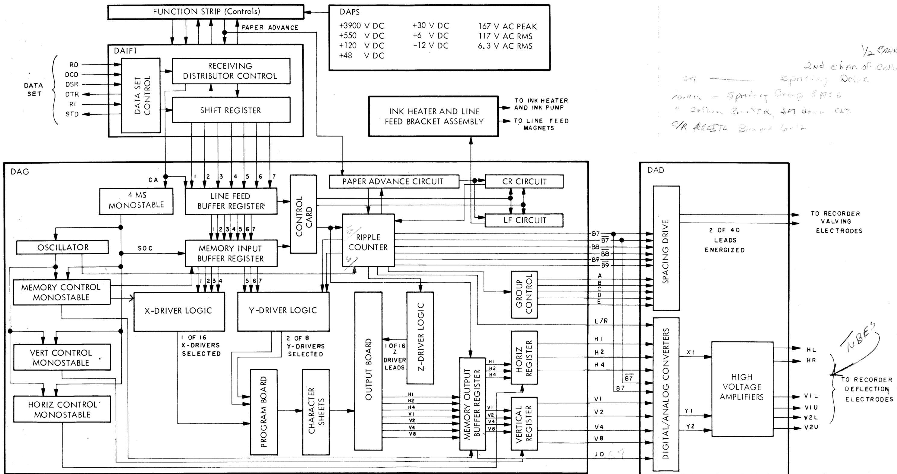
Figure 4 - Block Diagram of DATASPEED Printer (Receive-Only) Electronic Circuits (Serial Interface)
