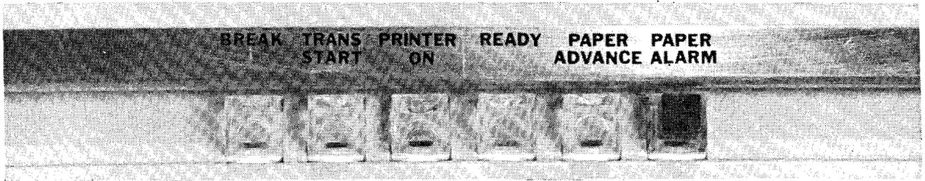
Figure 5 - Operator Controls (At Front of Cover)
