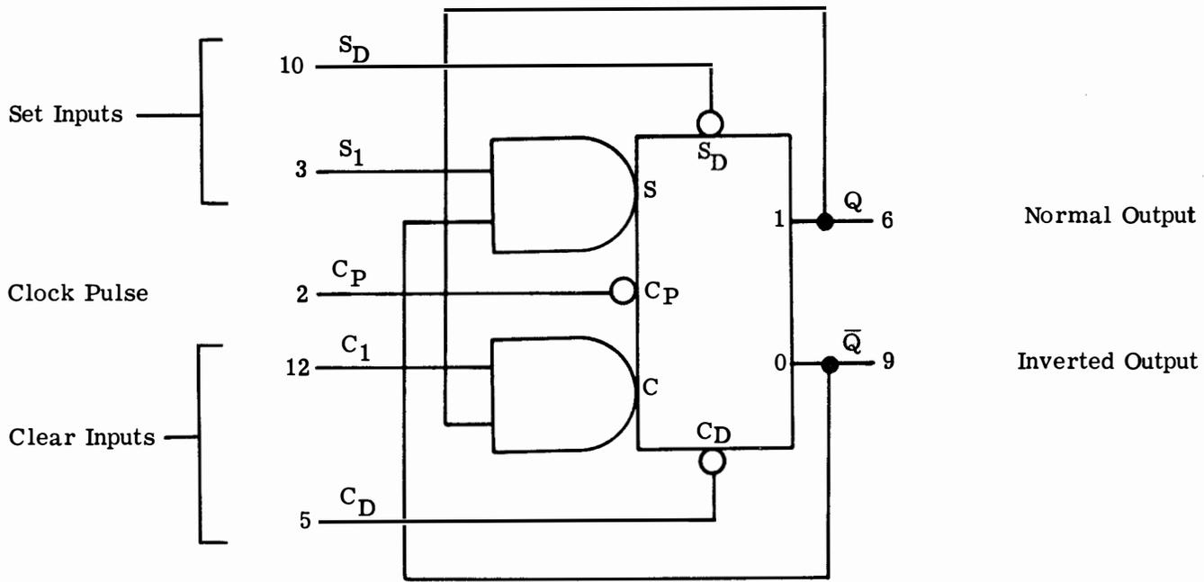
Clocked Flip-Flop Connected for J-K Operation
