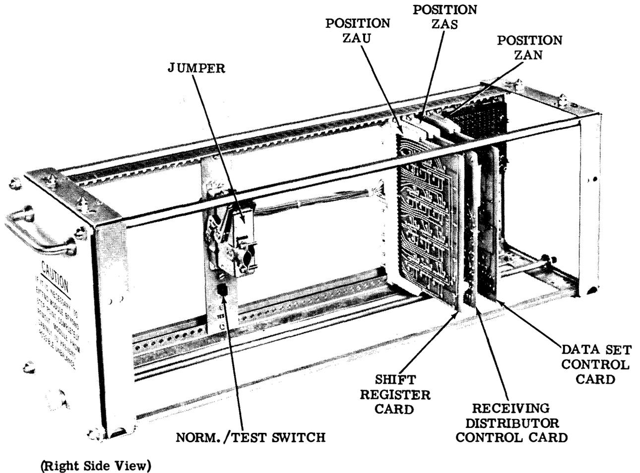
Figure 6 - DAIF1 Serial Interface Module
