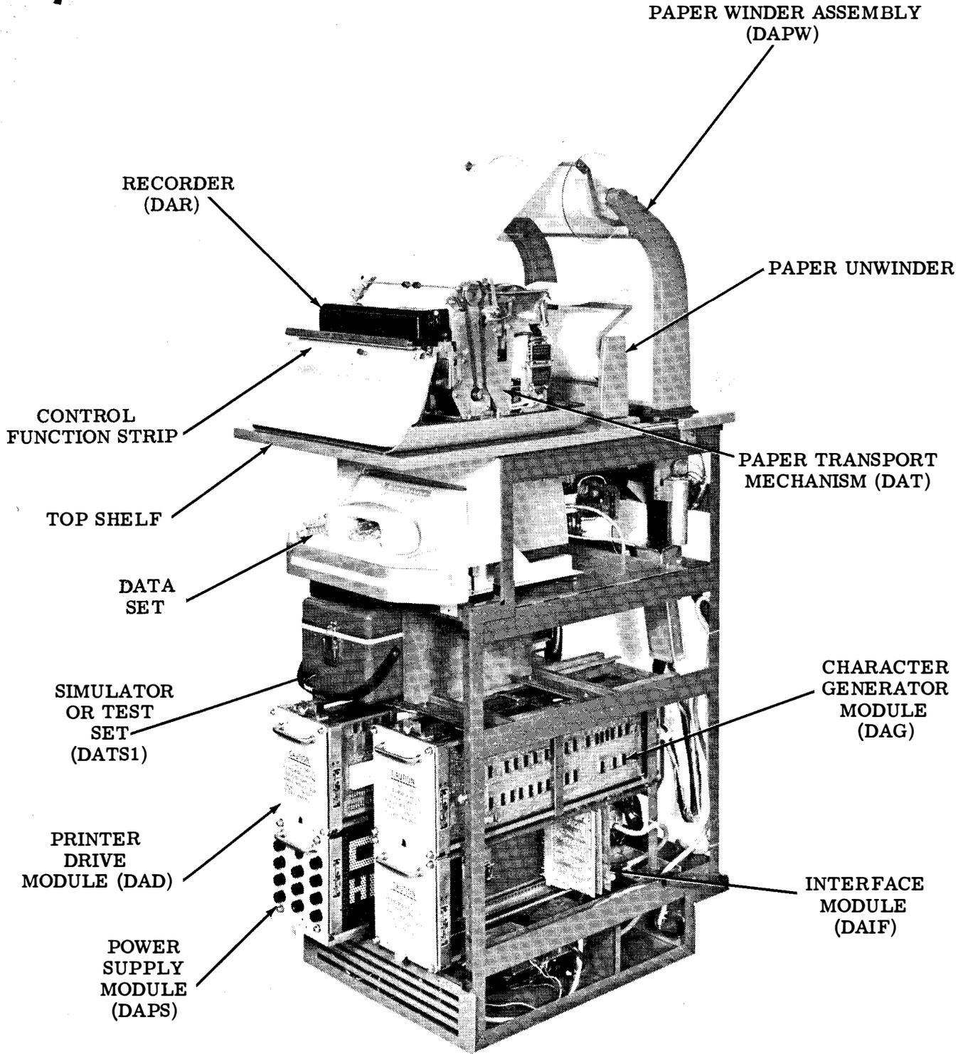
Figure 3 - DATASPEED Printer With Cabinet Panels and Cover Removed and Top Shelf and Modules Extended
