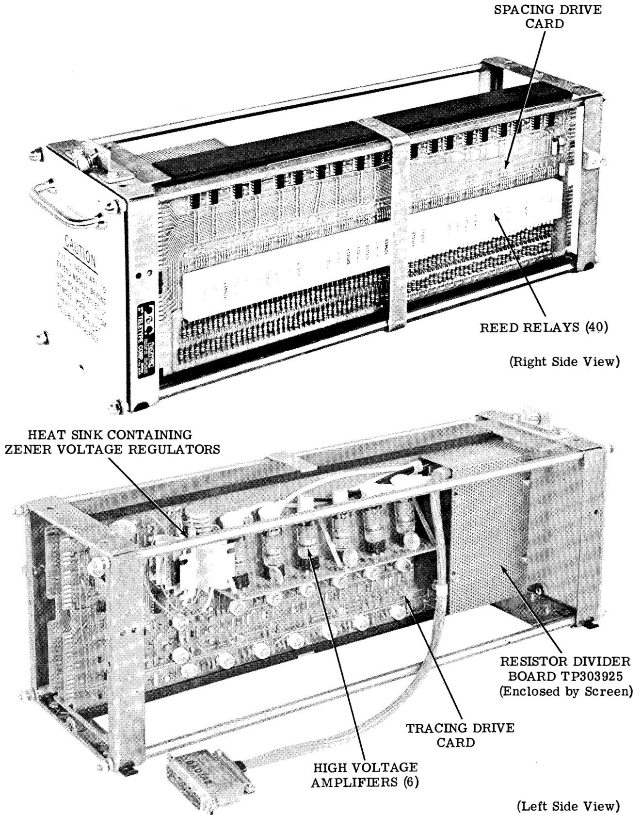
Figure 10 - Printer Drive (DAD) Module
