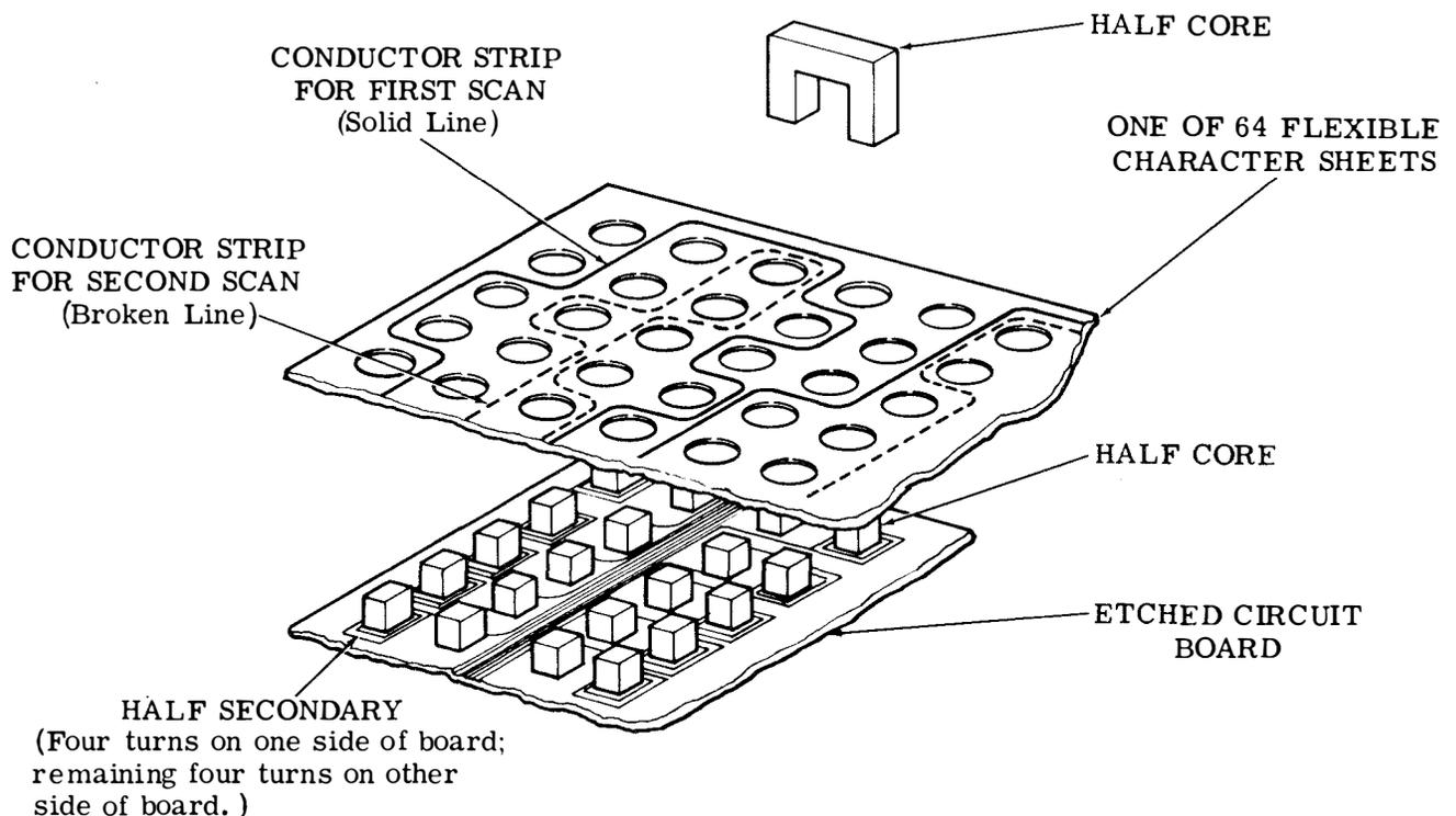
Figure 9 - Core Arrangement and Conductor Routing on Character Sheets
