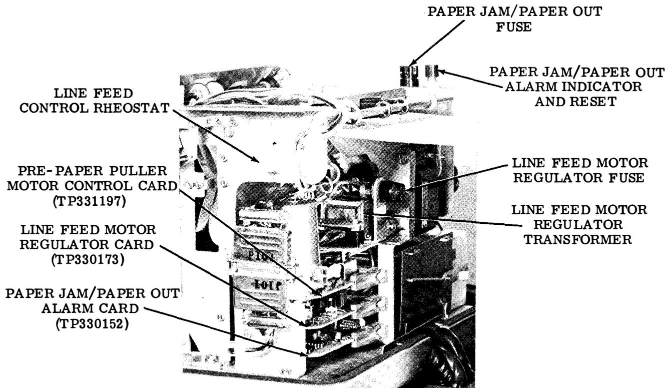
Figure 14 - Control Circuitry at Rear of Transport Base
