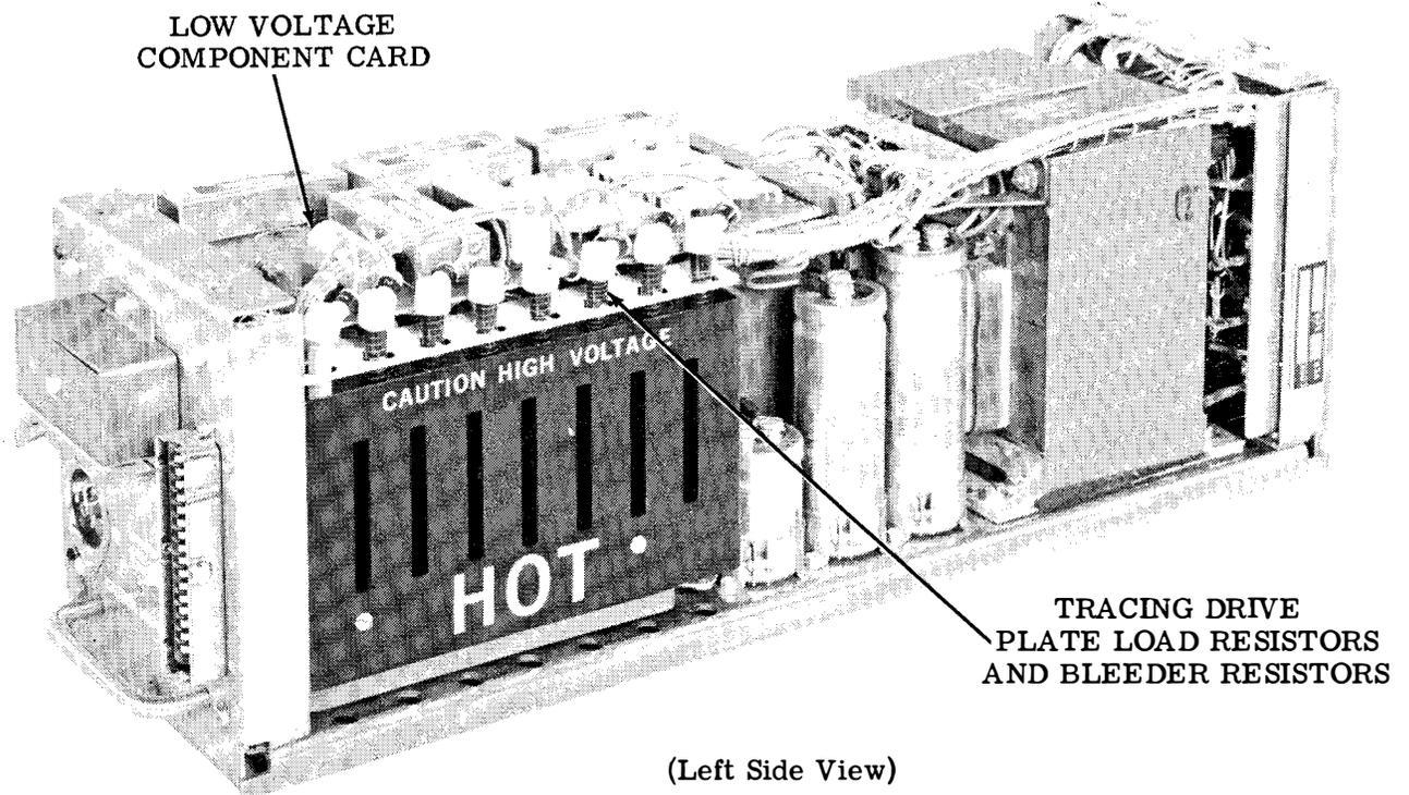
Figure 13 - Power Supply (DAPS) with Cover Removed
