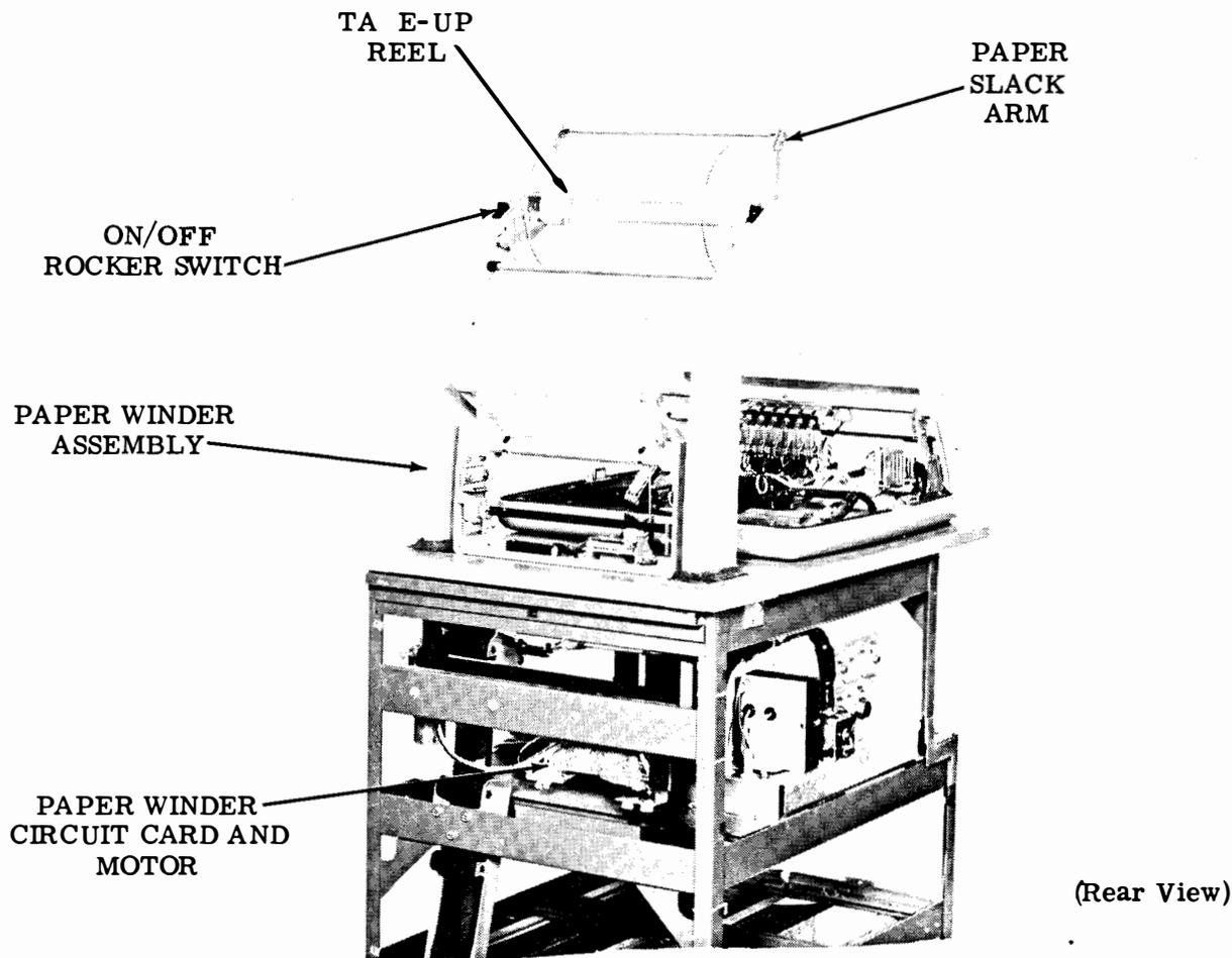
Figure 16 - Top Frame of DATASPEED Printer
