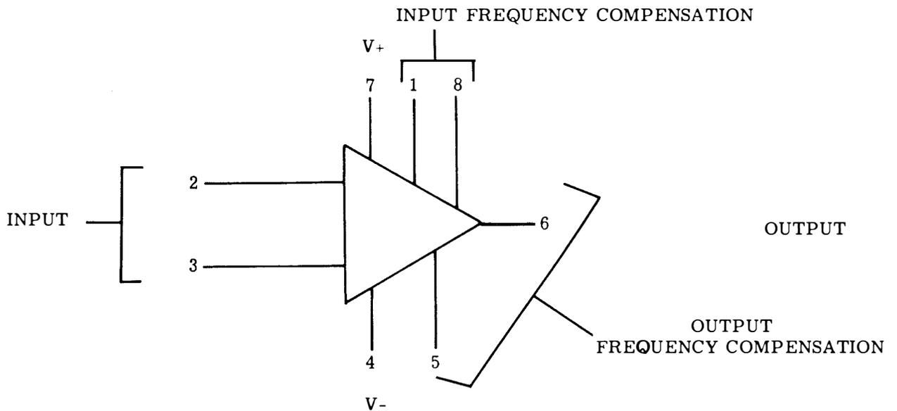
Figure 22 - Operational Amplifier (Op Amp)
