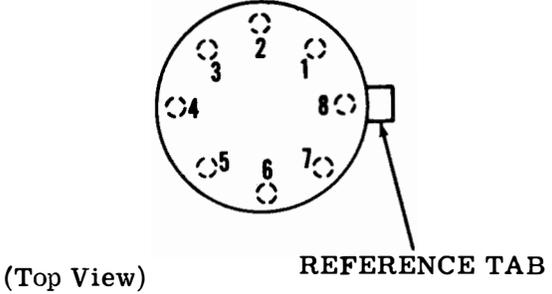
TO-Type Integrated Circuit Package
