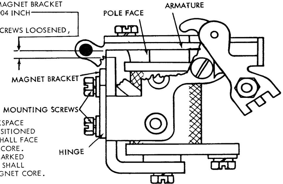
NOTE: FOR "DC" OPERATION, THE BACKSPACE MAGNET ARMATURE SHALL BE POSITIONED SO THAT THE SIDE MARKED "C" SHALL FACE THE POLE FACE OF THE MAGNET CORE. FOR "AC" OPERATION, THE UNMARKED SIDE OF THE MAGNET ARMATURE SHALL FACE THE POLE FACE OF THE MAGNET CORE.
