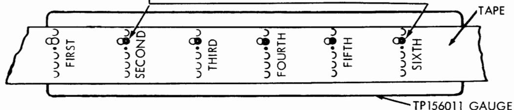
NOTE: THE FIRST FIVE HOLES IN GAUGE ARE THE SAME SIZE AS CODE HOLES IN TAPE (0.072 INCH DIAMETER) BUT THE SIXTH HOLE IN GAUGE IS LARGER THAN THE FIRST FIVE (0.086 INCH DIAMETER). THIS ARRANGEMENT ALLOWS  $\pm 0.007$  INCH VARIATION IN FIVE (5) INCHES.
