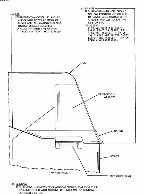
TO ADJUST----WITH WINDOW MOUNTING NUTS FRICTION TIGHT,
