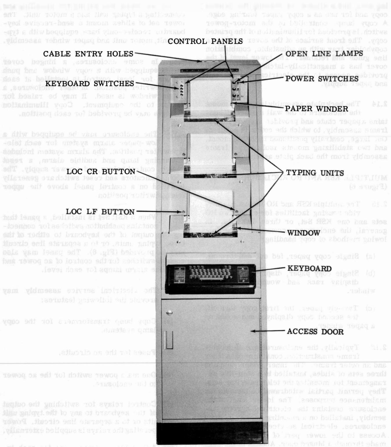
Figure 6 - Multiple KSR and RO Enclosure
