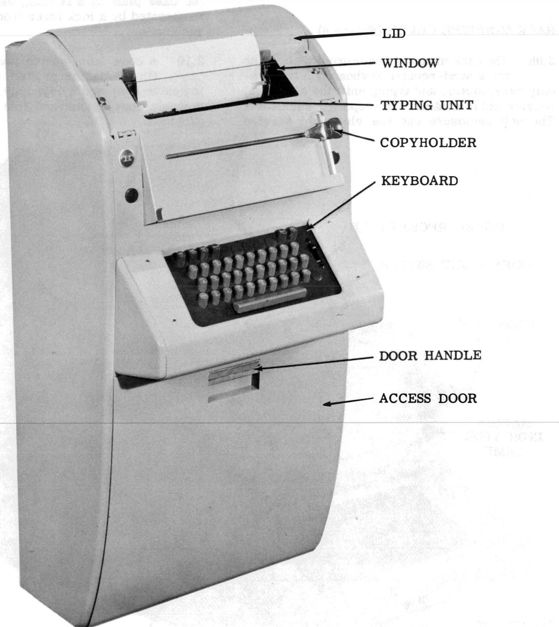
Figure 5 - Wall Mounted Enclosure
