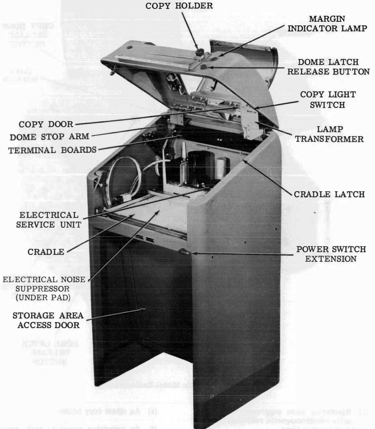
Figure 2 - Floor Model Enclosure (with Electrical Service Unit)
