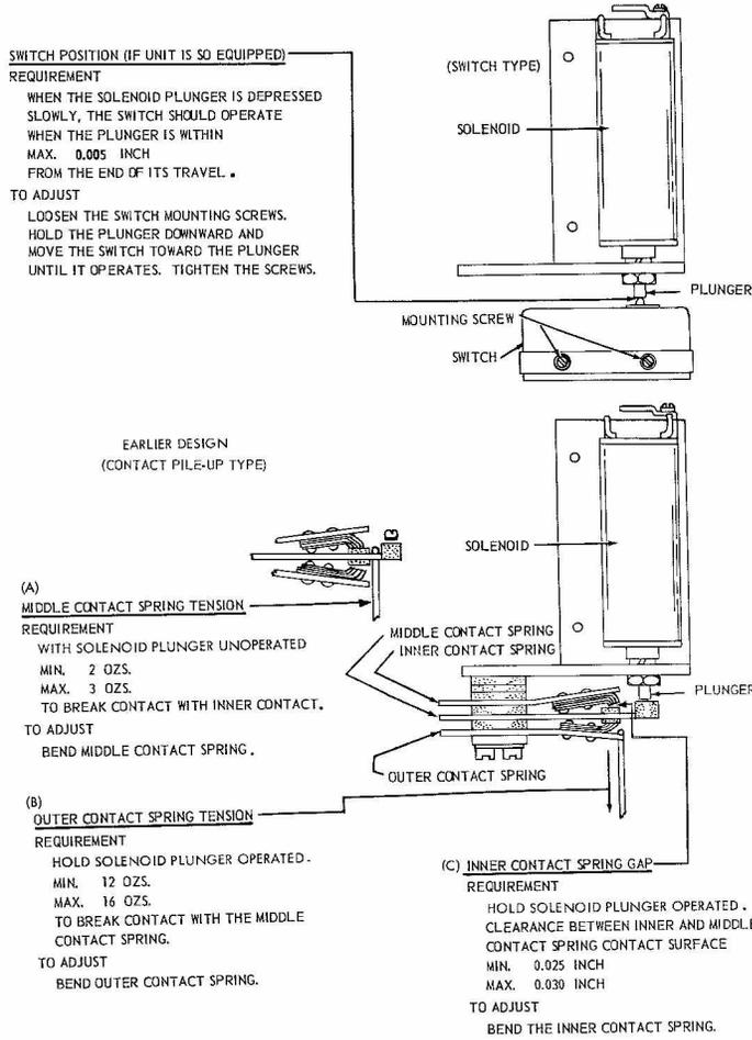
2.05 Line Test Key Assembly (if Equipped)
