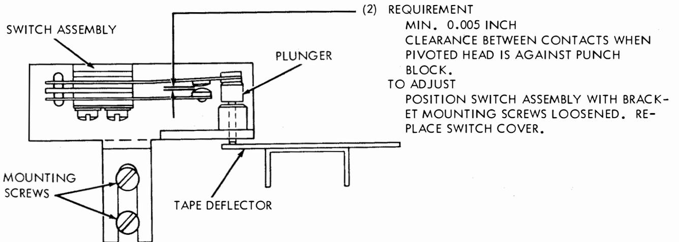
2.24 Tape-out and Tape-lid Switch (28B Unit Without START-STOP Lever)
