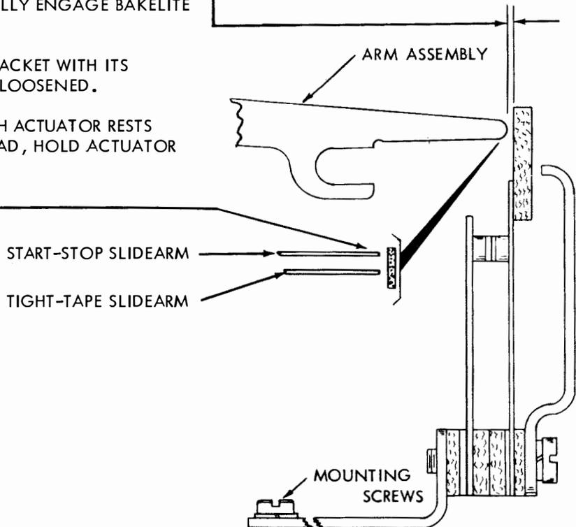
2.30 Contact Timing Requirements for Pivoted Sensing Head (One-cycle Cam)
