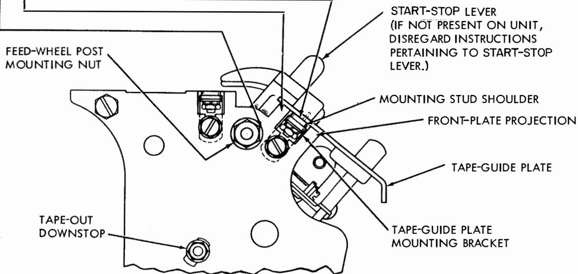
2.12 Tape Feed Mechanism (28B Unit)
