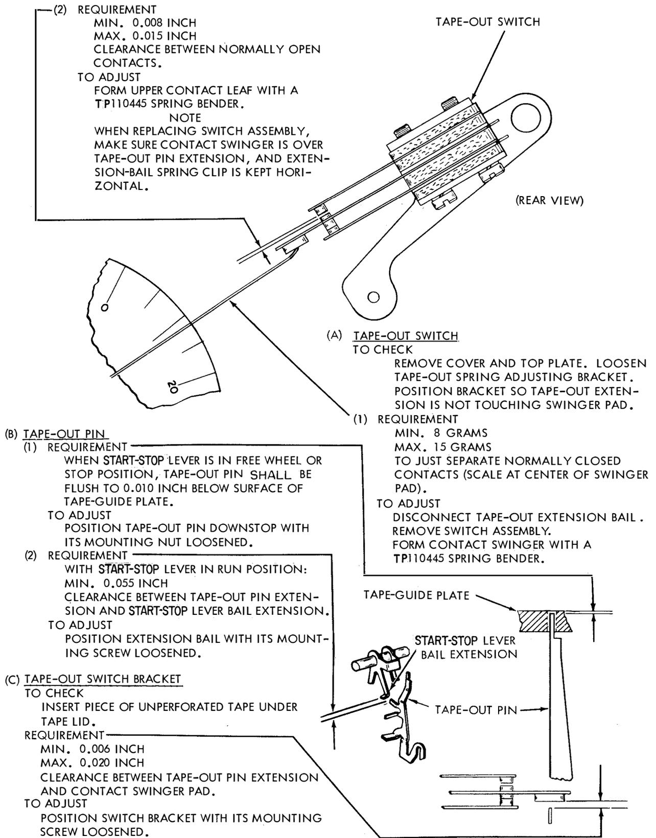
2.28 Tape-out Pin and Bail Assembly (28B Unit With START-STOP Lever)
