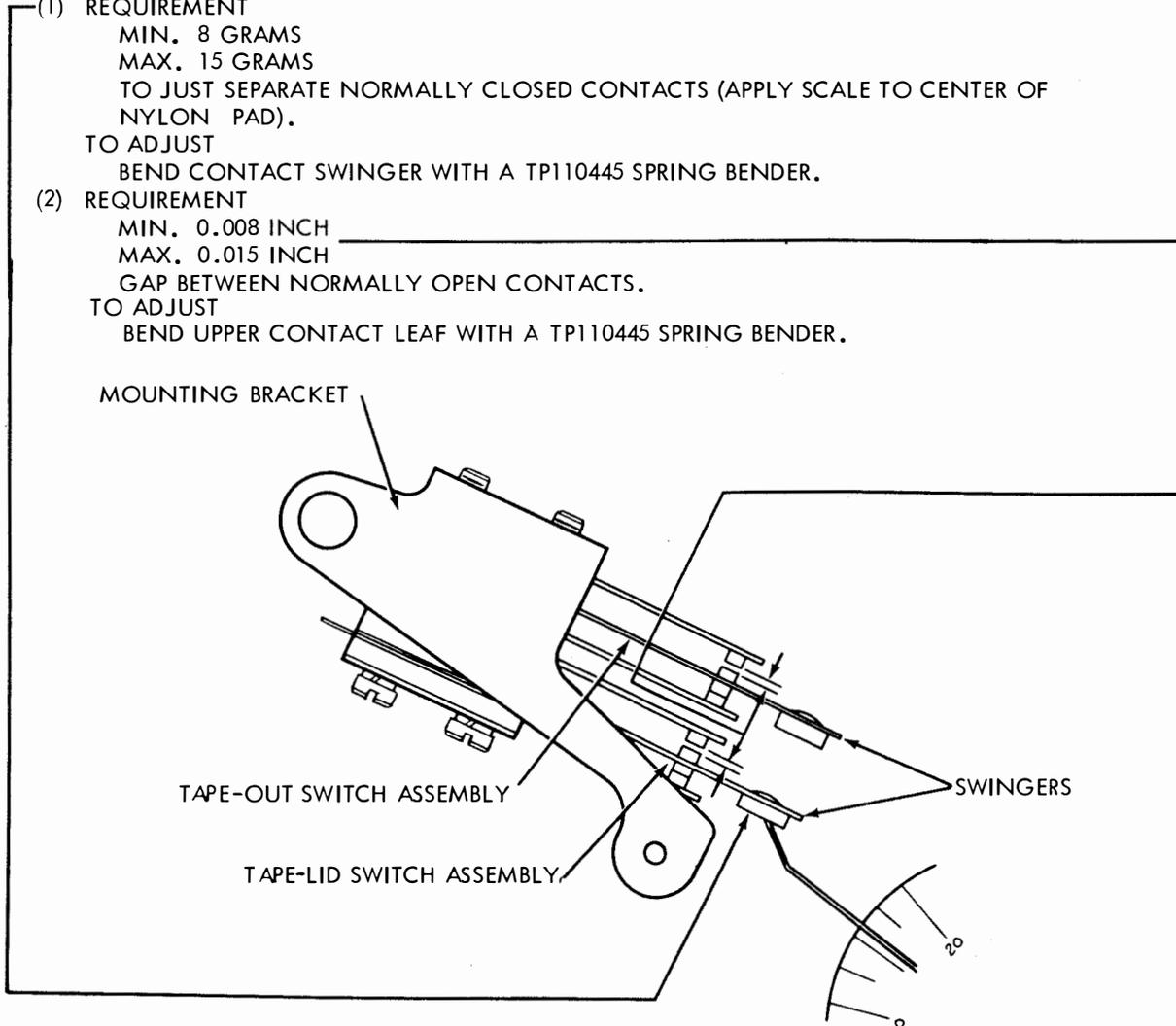
INSTRUCTIONS FOR REMOVING TAPE-OUT AND TAPE-LID SWITCH ASSEMBLY
