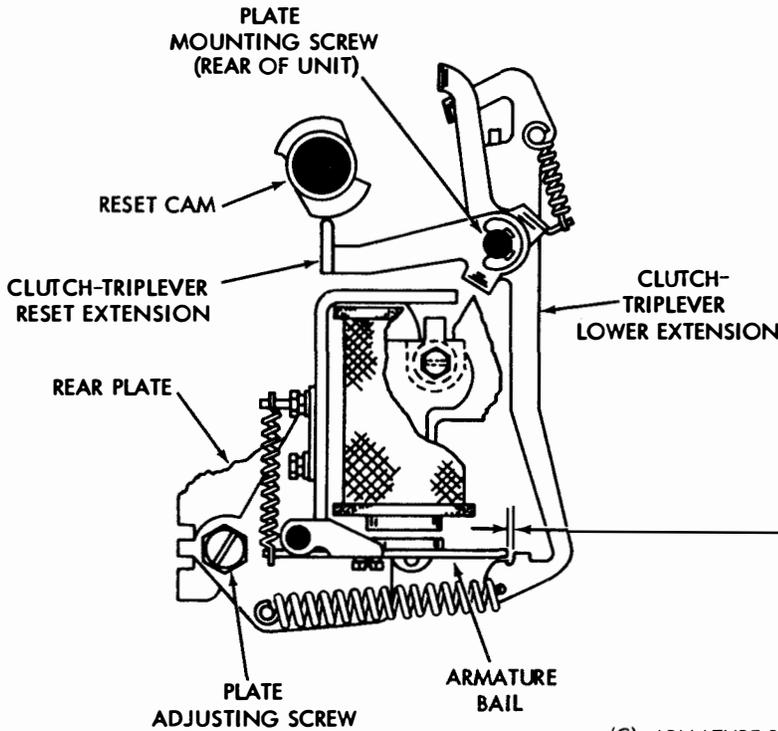
(B) CLUTCH TRIP ASSEMBLY MOUNTING PLATE
