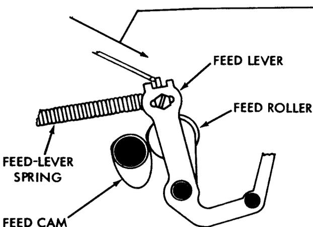
(B) FEED-LEVER SPRING (PIVOTED HEAD)
