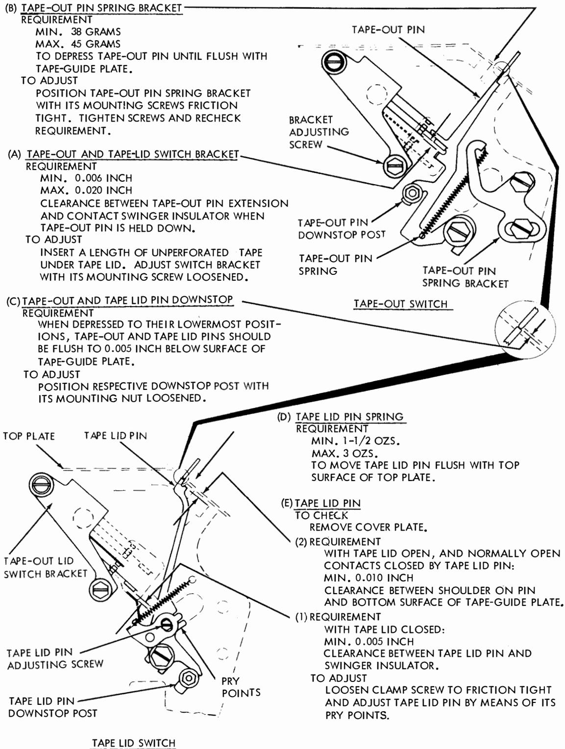
2.26 Tight-Tape Switch Assembly (28B Unit)
