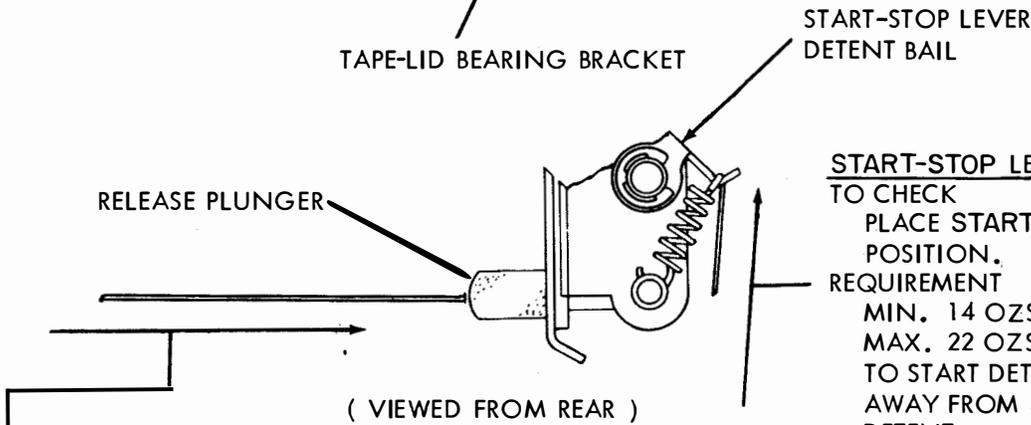
START-STOP LEVER DETENT SPRING TO CHECK
