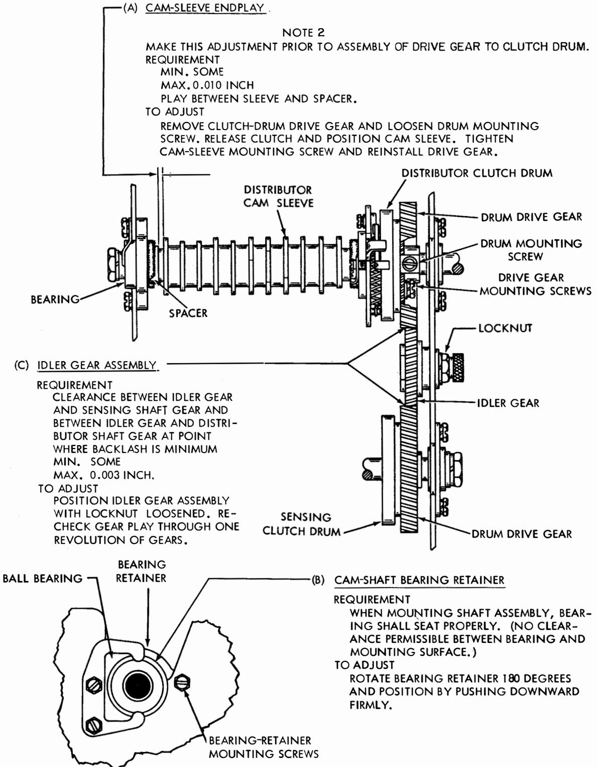
2.03 Clutch Trip Mechanism
