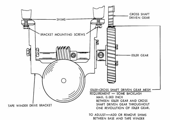
DRIVE BRACKET. KEEP EQUAL NUMBER OF SHIMS ON EACH SIDE.
