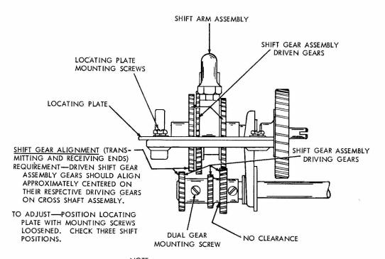
MAKE CERTAIN THAT THE TWO PORTIONS OF THE SHIFT GEARS ON THE CROSS SHAFT ASSEMBLY ARE MOUNTED WITH NO CLEARANCE BETWEEN THEM. IF THERE IS CLEARANCE, LOOSEN DUAL GEAR MOUNTING SCREW AND ELIMINATE CLEARANCE BEFORE MAKING ABOVE ADJUSTMENT.
