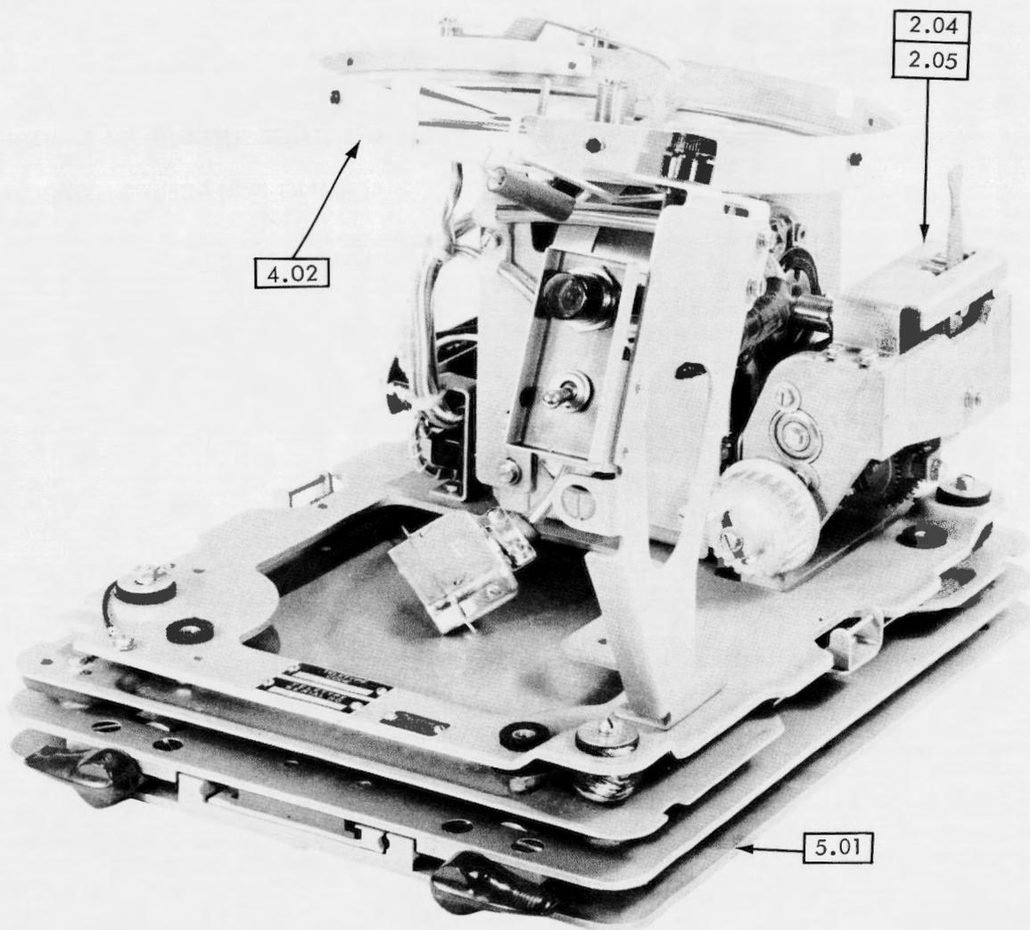
4.02 Low Tape Alarm Switch (Top View)
