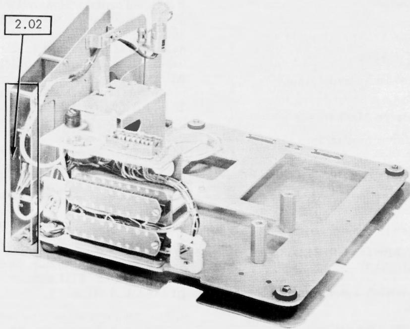
2.02 Low-Tape Alarm Switch Mechanism (Right-side View)
