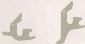
In addition to providing an anchor for one end of the function lever spring—the function latch will engage a function lever with a latch extension, and hold the lever in the operated position until released by the stripper blade during the next cycle of operation.
