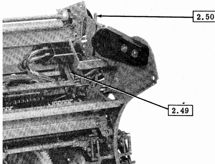
2.49 Line Feed Mechanism (Friction Feed)
