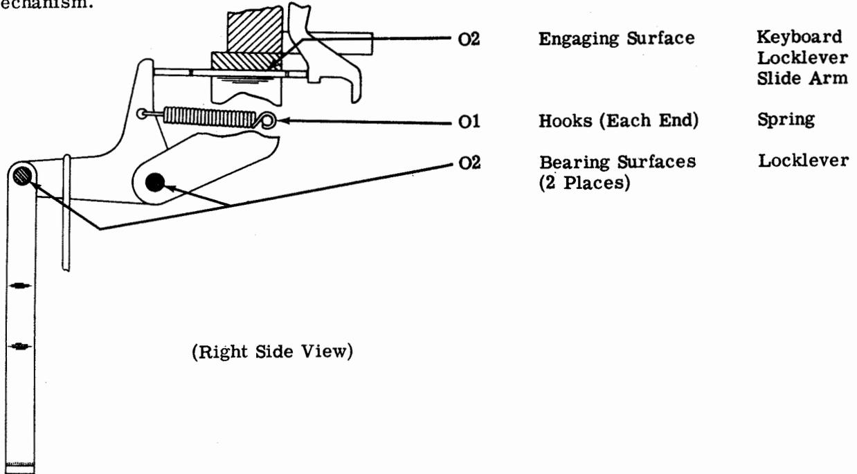
3.21 Paper Jam Alarm (Sprocket Feed)
