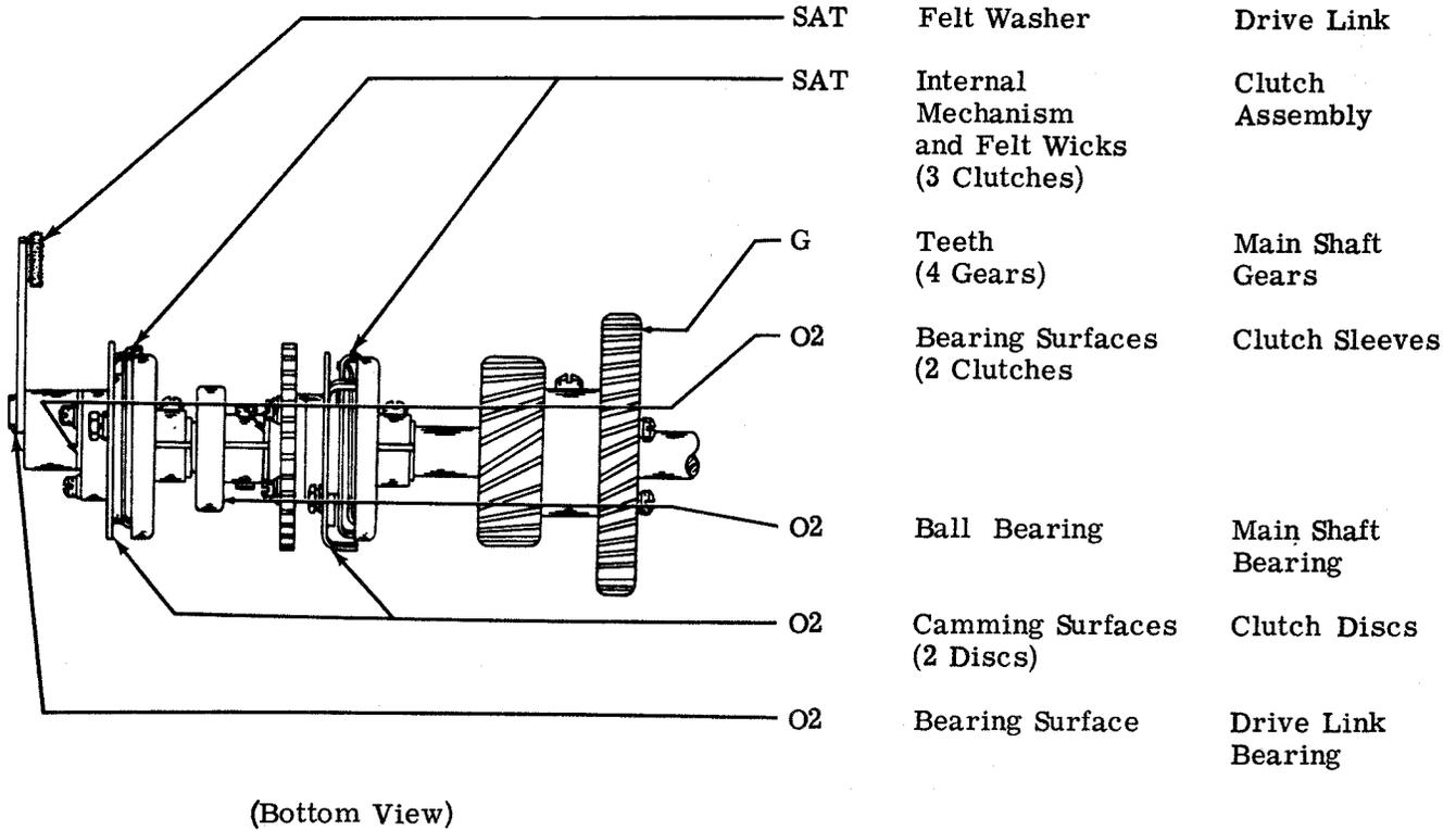
2.40 Main Shaft (Clutches, Gears, etc) (continued)
