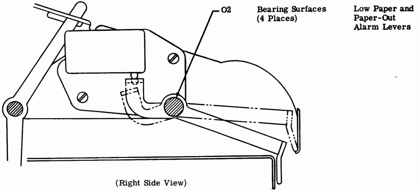
3.20 Keyboard Lock Mechanism
