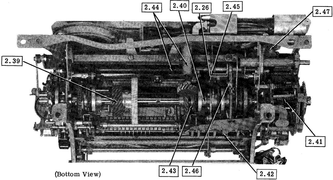
2.39 Main Shaft (Clutches, Gears, etc)
