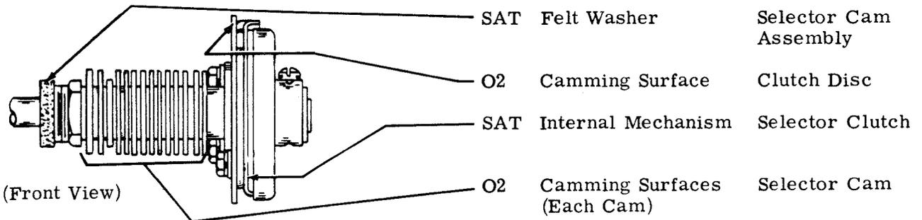
2.42 Trip Shaft Mechanism
