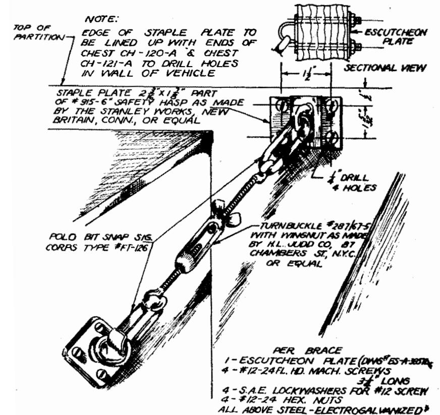
FIGURE 2.—Drawing of turnbuckle brace used to hold chest in shelter.
