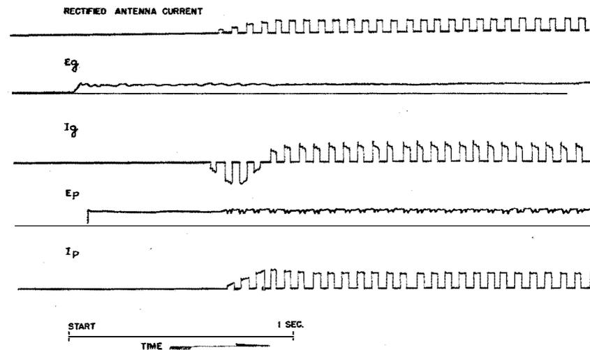
FIGURE 5.—Oscillographs with equipment operating on M. C. W. and keyed at 40 words per minute.
