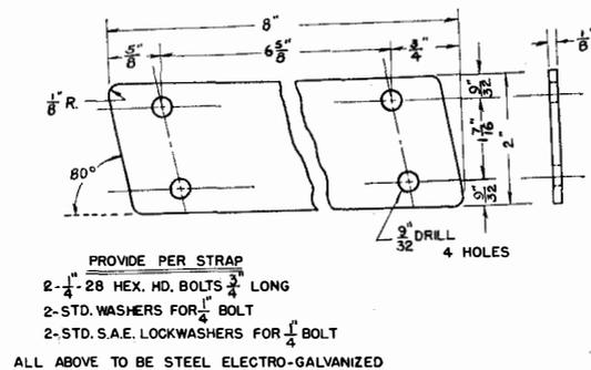
FIGURE 6.—Detail of reinforcing strap for cover.
