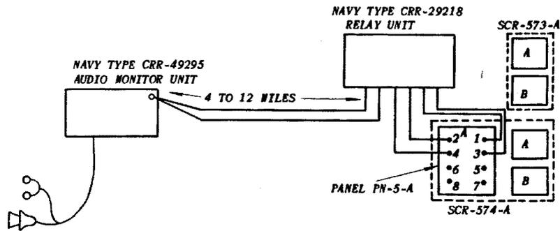
FIGURE 4.—Audio monitor unit, with relay unit, for controlling one truck with two transmitters and one truck with two receivers, in block diagram relationship.
