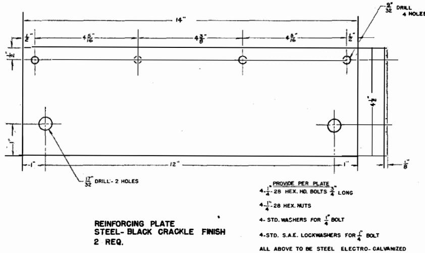
FIGURE 3.—Detail of reinforcing plate.
