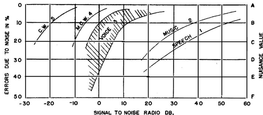
FIGURE 1.—Graph showing effect of signal to noise ratio on the intelligibility of signals.
