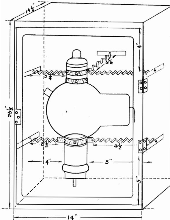
FIGURE 1.—Drawing showing outline of protective cage for type 861 spare vacuum tubes.
