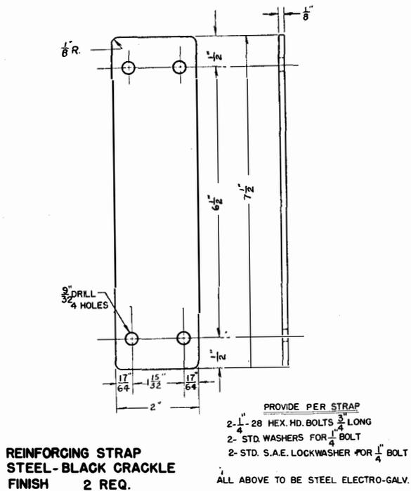
FIGURE 5.—Detail of reinforcing strap for cover.
