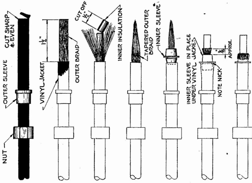
1. CUT END OF CABLE EVEN & SLIDE THE OUTER SLEEVE AND THE NUT OVER CABLE
