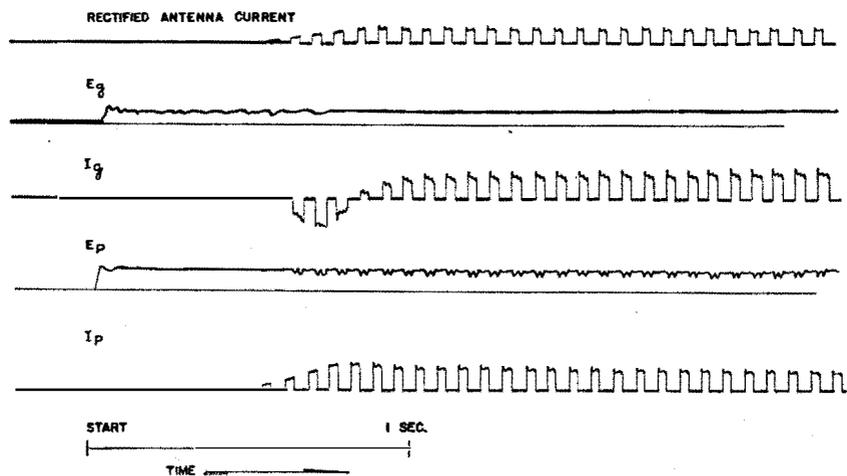
FIGURE 4.—Oscillographs with equipment operating on C. W. and keyed at 40 words per minute.
