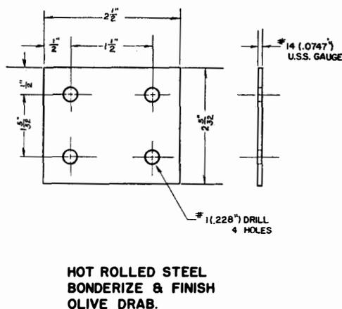
FIGURE 8.—Detail of escutcheon plate.
