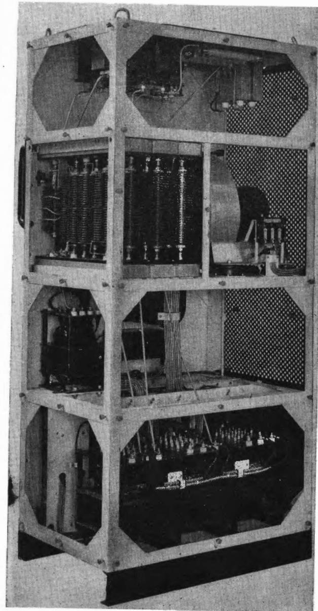
FIGURE 2.—Navy type CAY-20167, copper oxide rectifier power unit, rear view, shields removed.
