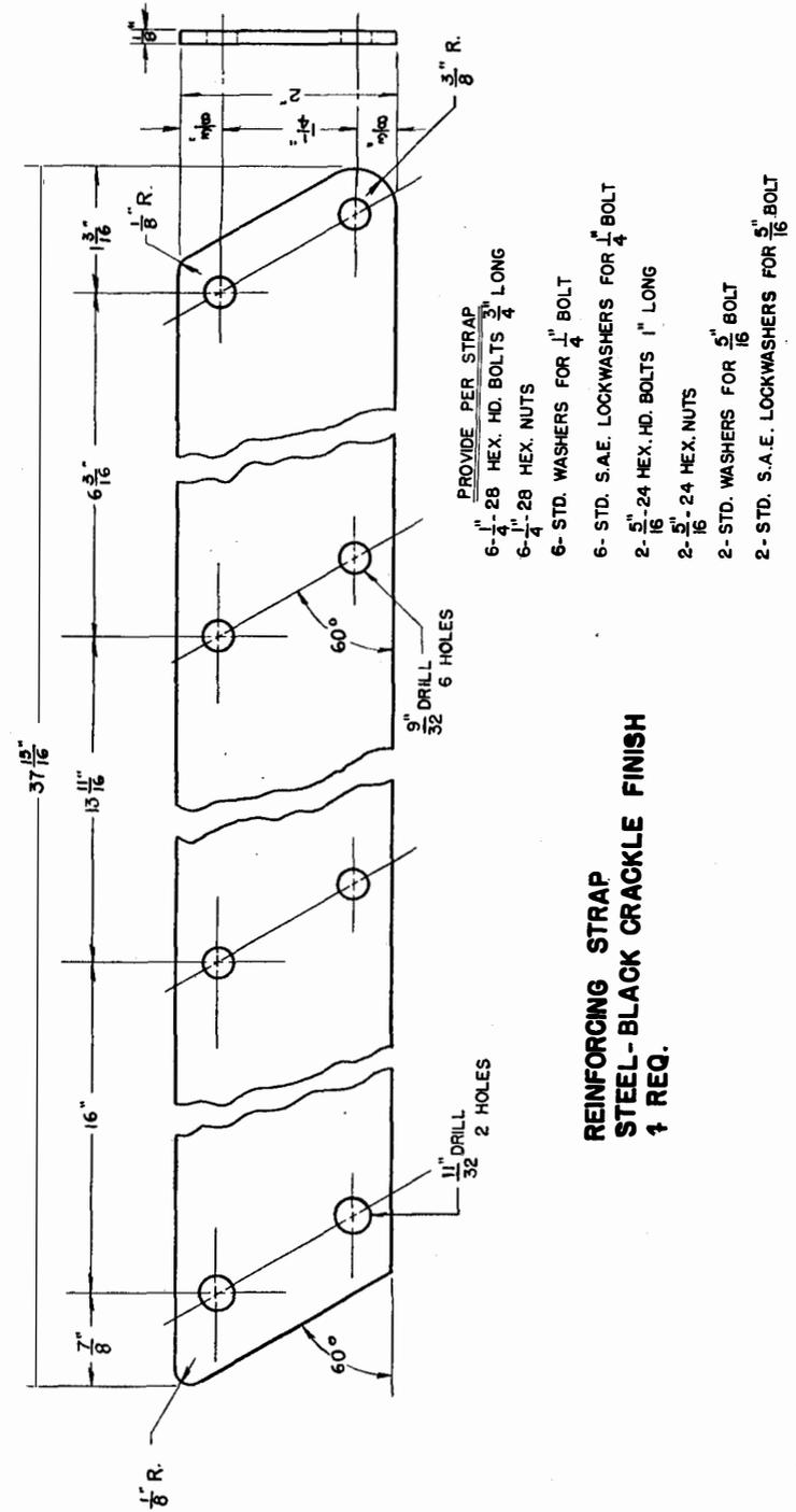
FIGURE 4.—Detail of reinforcing strap.
