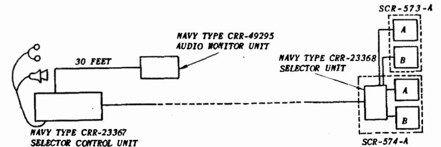
FIGURE 3.—Audio monitor unit, one selector control unit, one truck with two transmitters, and one truck with two receivers in block diagram relationship.
