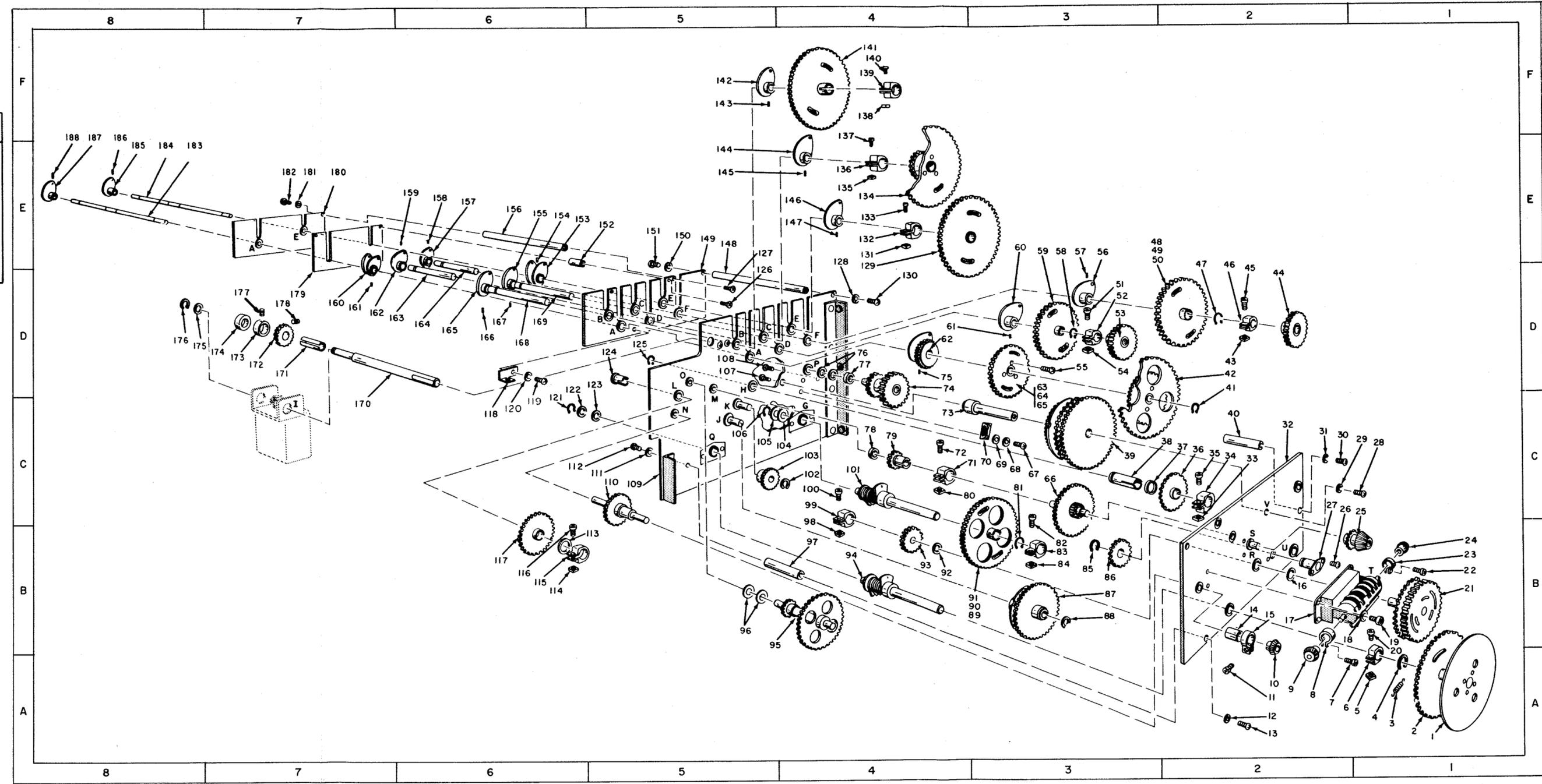
Figure 6-36. RF Gear Train Assembly, Exploded View
