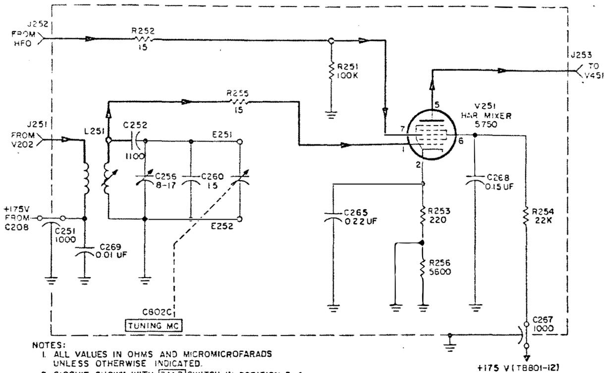
Figure 4-21. Harmonic Mixer, Simplified Schematic Diagram
