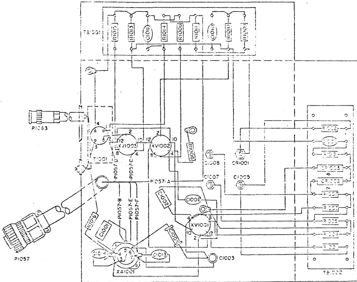
Figure 6-20. 100-Kc Oscillator-Amplifier, Wiring Diagram
