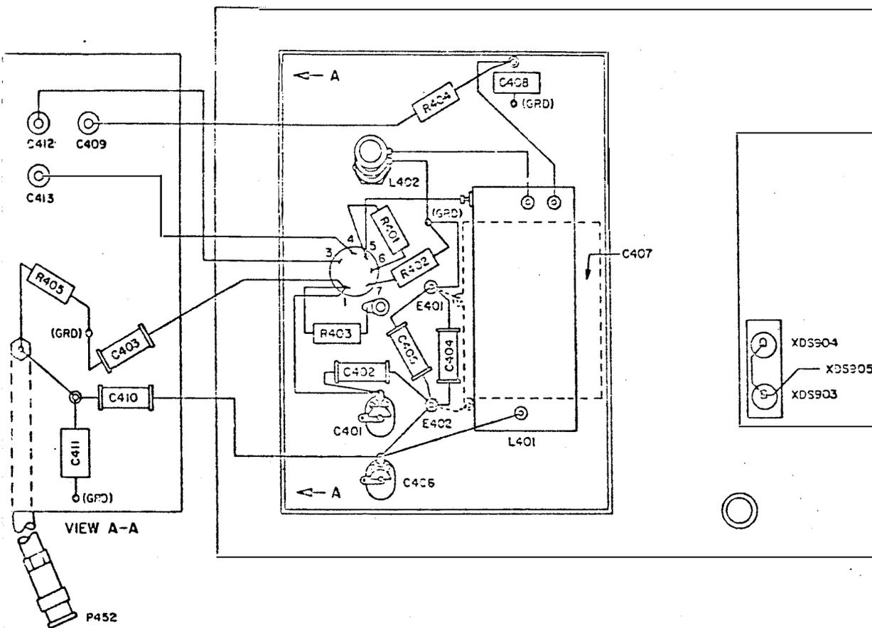
Figure 6-30. Interpolation Oscillator, Wiring Diagram
