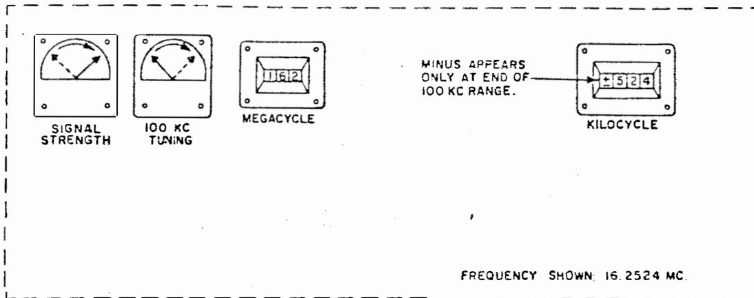
Figure 3-2. Frequency Counter and Meter Presentations
