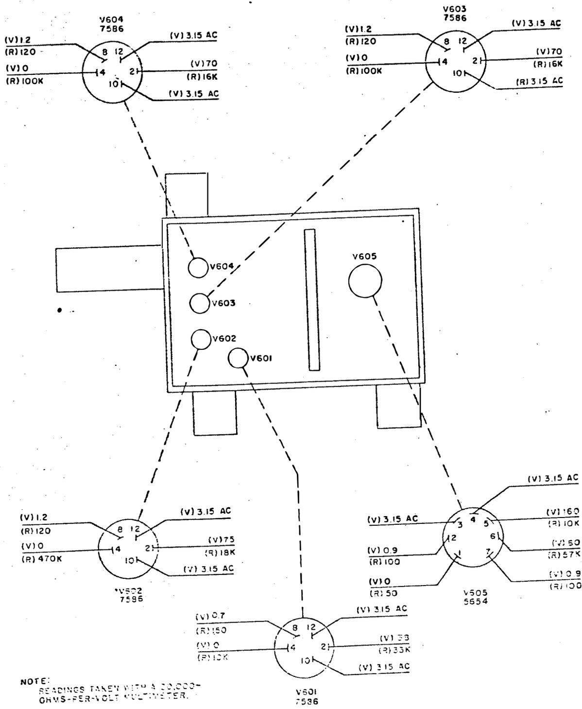
Figure 5-49. AGC Amplifier, Voltage and Resistance Diagram
