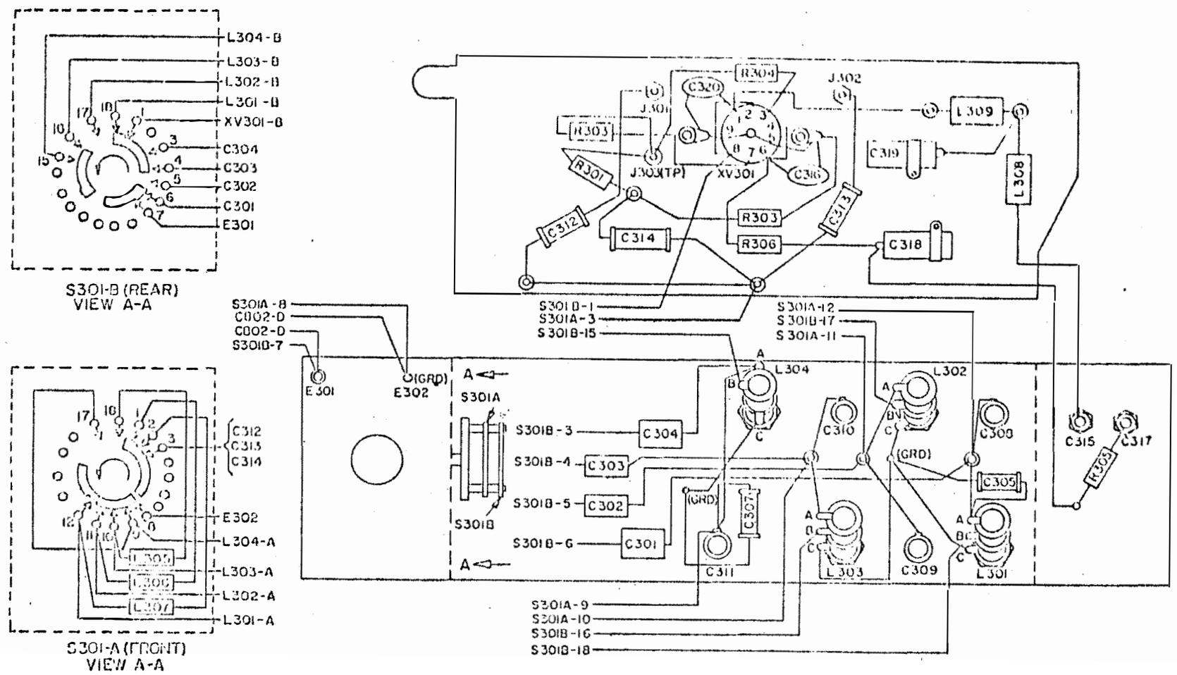
Figure 6-29. High-Frequency Oscillator, Wiring Diagram
