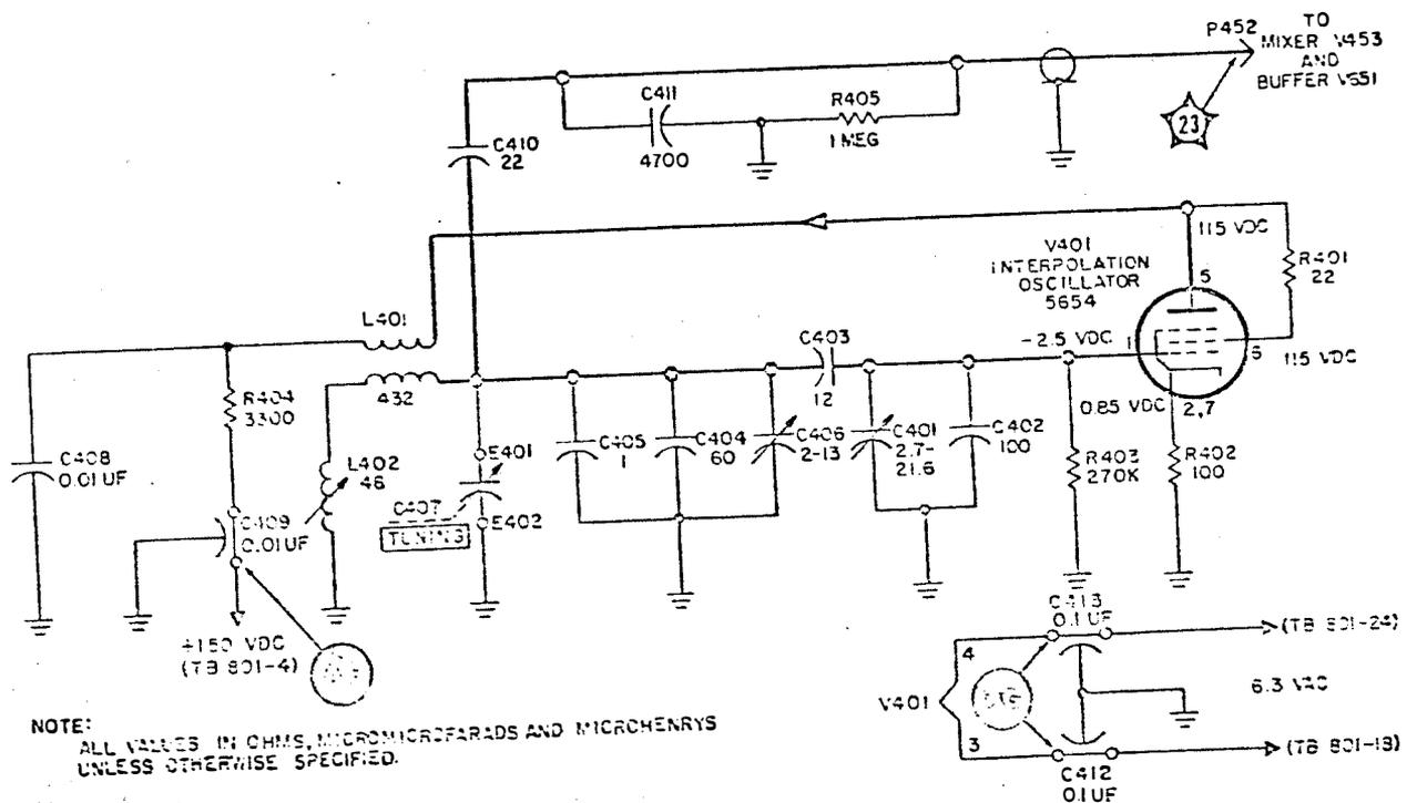
Figure 5-56. Interpolation Oscillator, Functional Schematic Diagram
