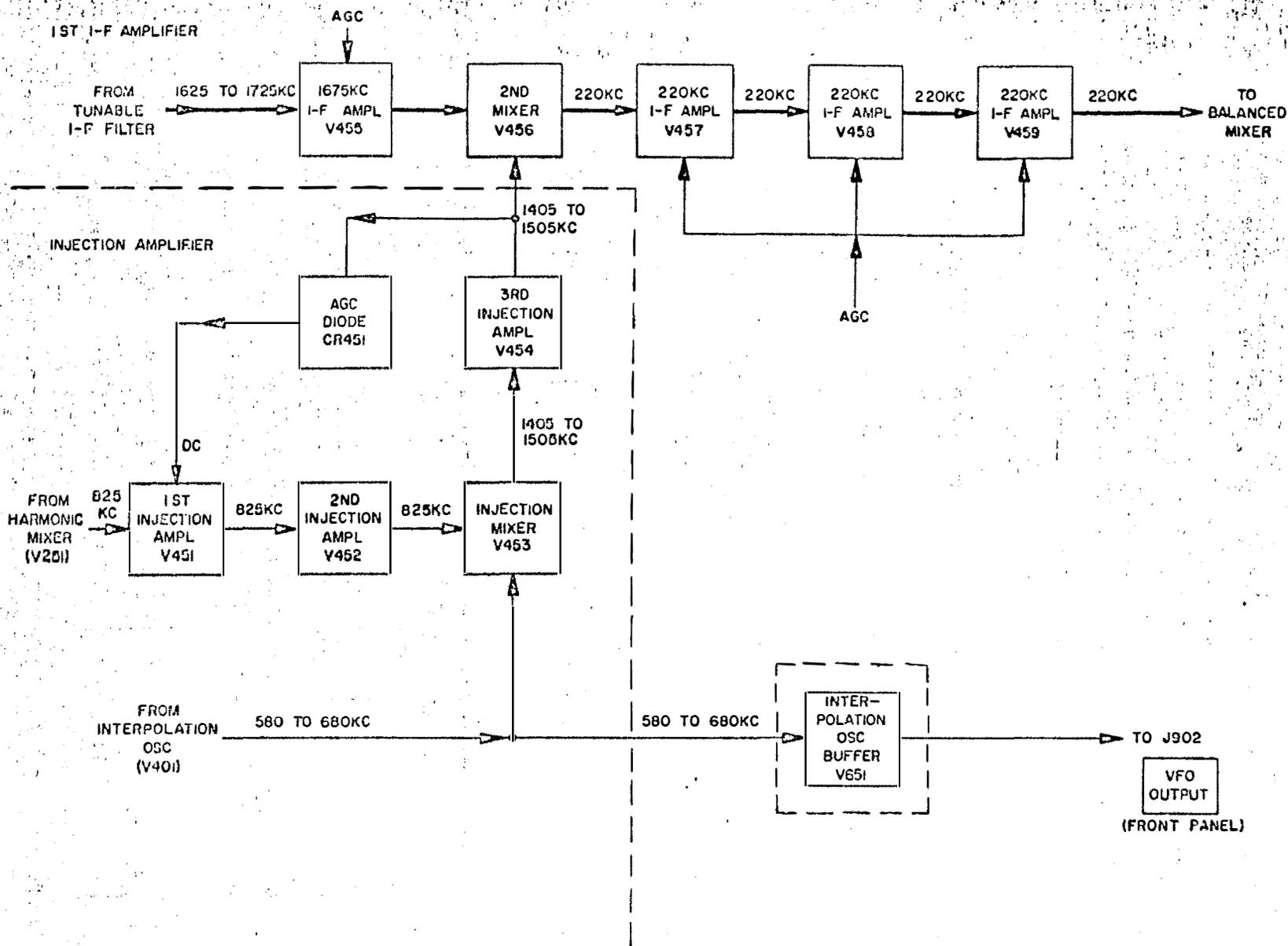
Figure 4-9. First I-F and Injection Amplifier, Block Diagram
