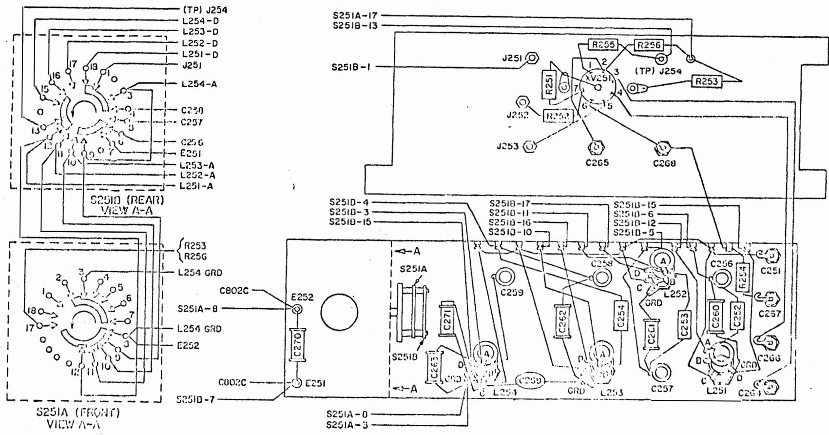
Figure 6-32. Harmonic Mixer, Wiring Diagram
