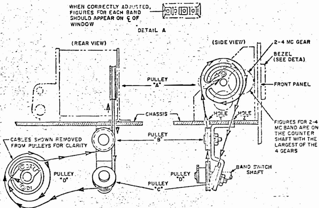
Figure 6-6. Megacycle Counter, Drive Cable Installation
