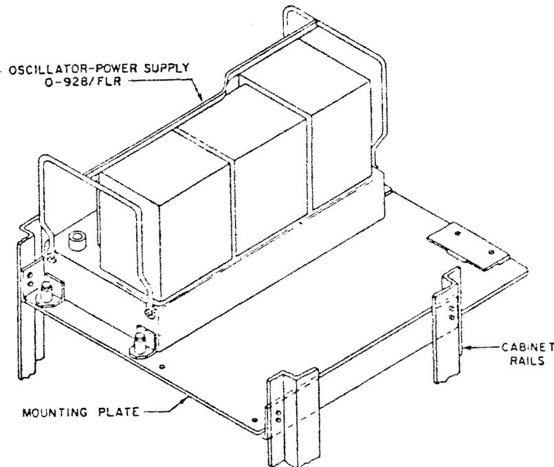
Figure 2-6. Mounting Plate, Installation Details
