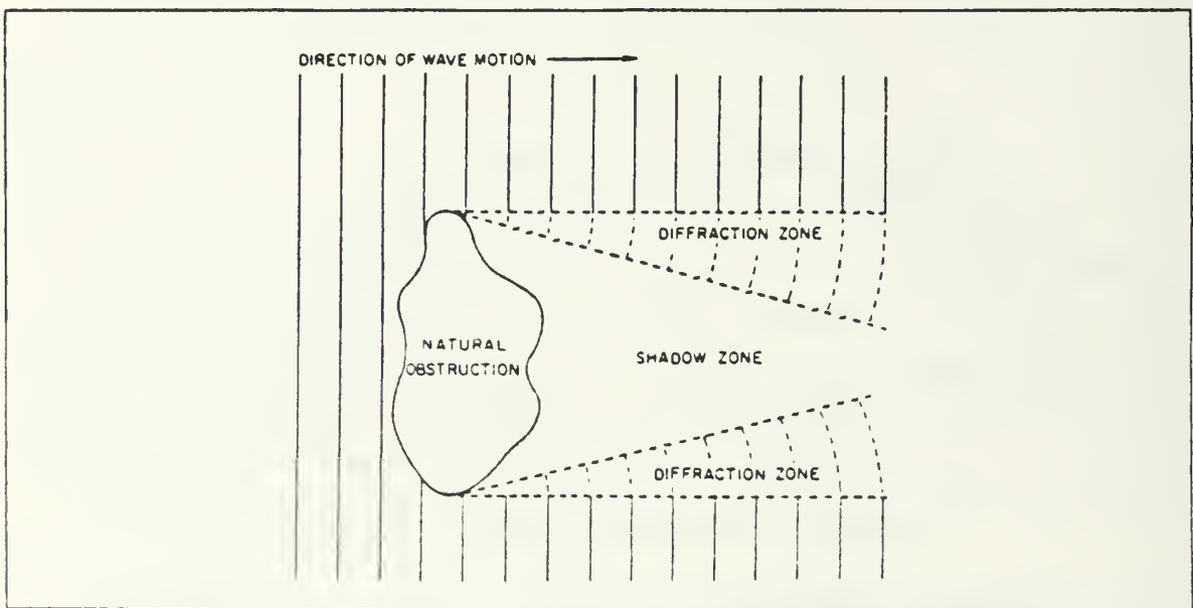
Figure B.2 Diffraction of Waves.
