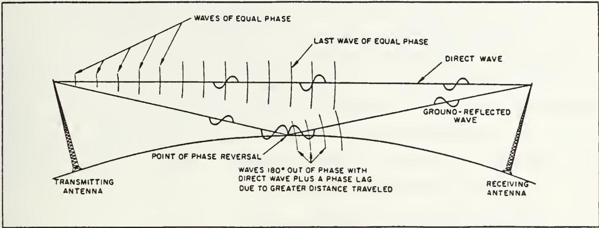
Figure B.9 Direct and ground reflected waves.
