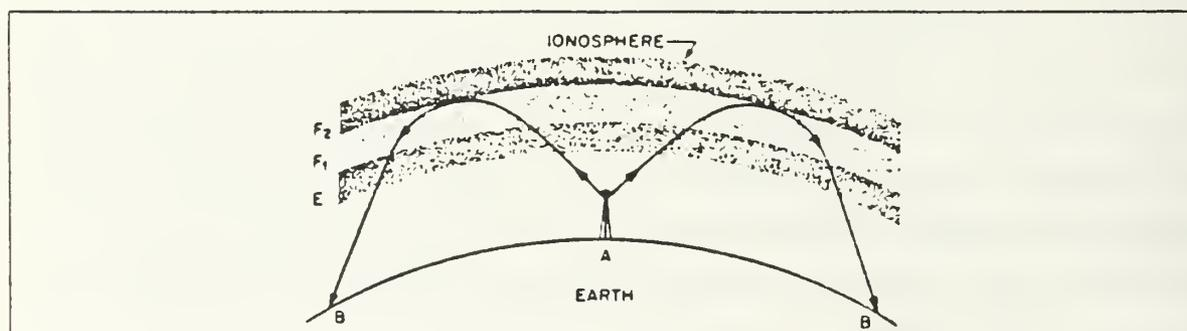
Figure B.13 Ionosphere bends waves back to earth.
