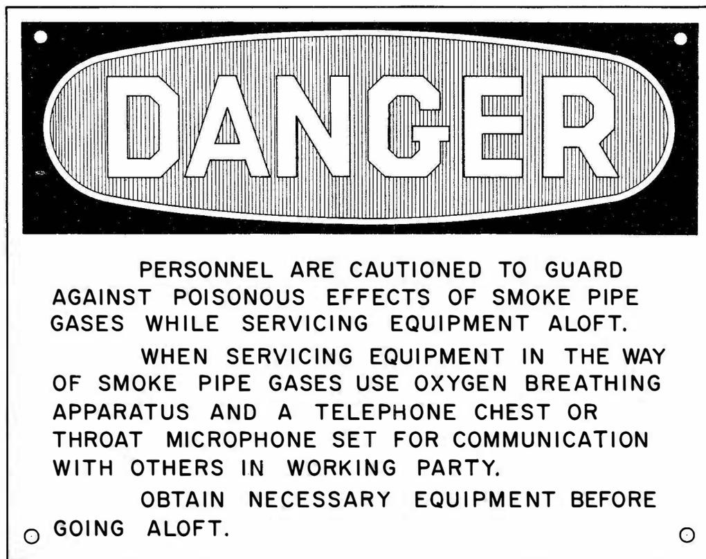
FIG. 3-4-2, Smoke Pipe Gases Warning Sign.
