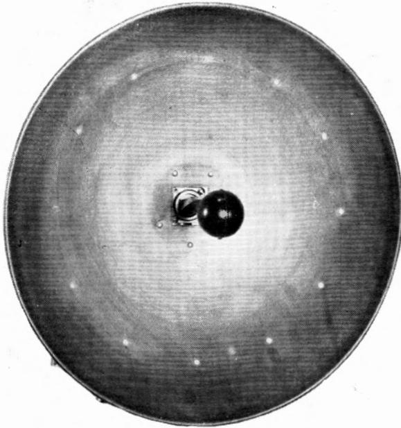
*Antenna dipoles of the AN/APS-3A equipment are enclosed in a plastic sphere, as shown above. The RF plumbing is pressurized from magnetron to antenna.*
