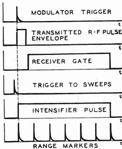
Fig. 2. Control pulses furnished by the timer of Fig. 1.
