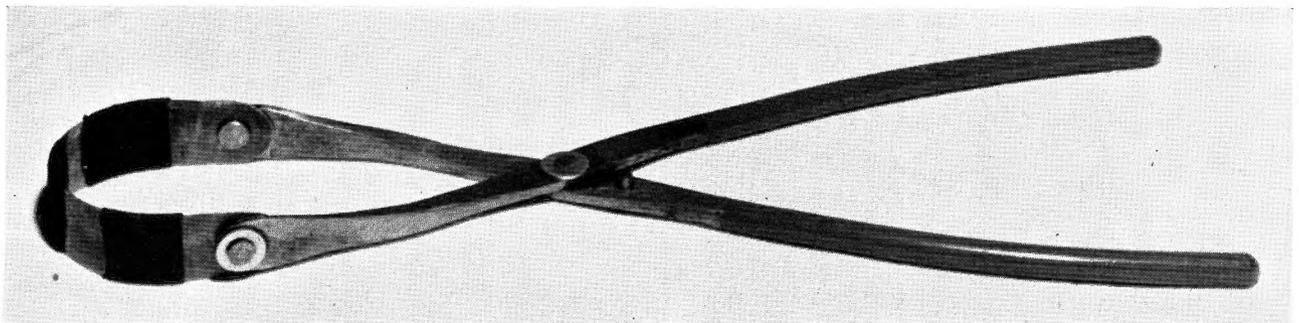
*The two views above show how the band on the vacuum tube extractor is flexible so that it may be used in flat or upright position.*
