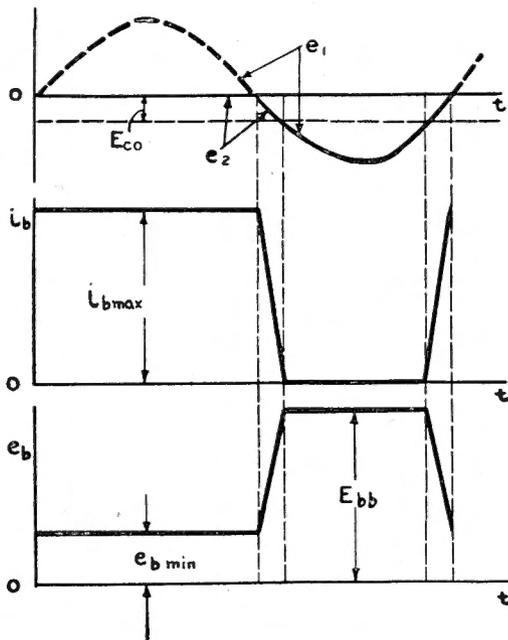
Fig. 10. Waveforms in clipper.
