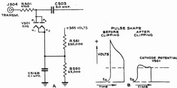
Indicator Limiter Stage—Circuit and Wave Shapes.
