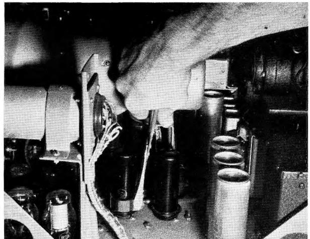
*The above photos demonstrate how the vacuum tube extractor may be used in tight and awkward places.*
