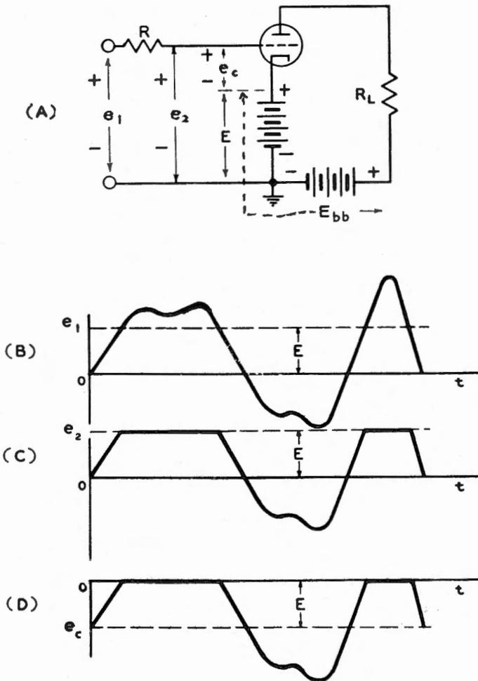
Fig. 7. Grid-circuit clipping.
