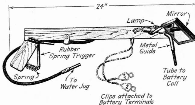
To use the gun, the operator simply removes the vent cap from each cell and holds or places the water container above the level of the battery. The gun is directed over each cell, in turn, and the level of the electrolyte is noted. If additional water is needed, the trigger is pulled and a stream of water flows into the cell until the correct operating level is attained.
