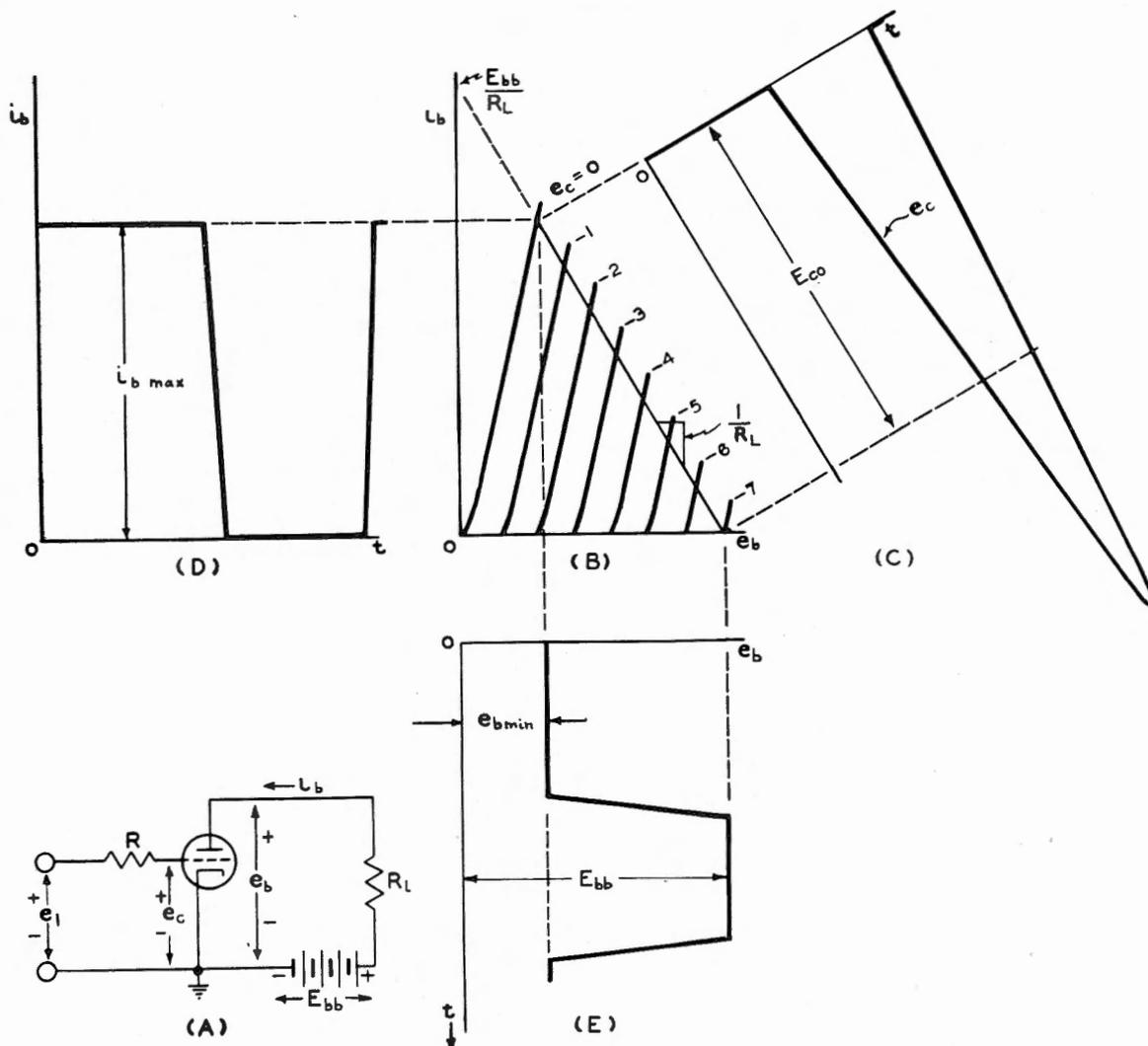
Fig. 9. Formation of a square wave by clipping a sine wave.
