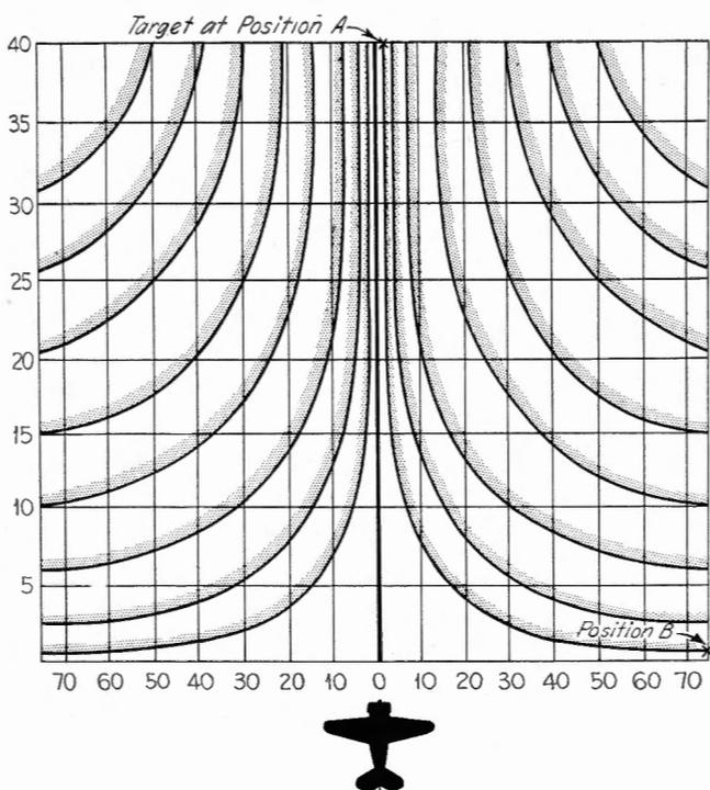
**Figure 1.** If an aircraft is flying parallel to an approximately straight coastline and its radar sights a target at position A, the target indication will move down the scope and veer off to the right as the plane approaches. When the aircraft is almost abeam of the target, the indication is at point B.
