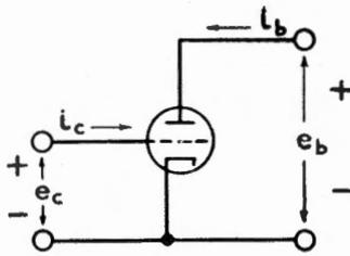
Fig. 6. Voltages and currents in amplifier-type tube.
