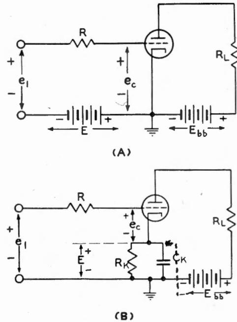
Fig. 8. Additional grid-circuit clippers.
