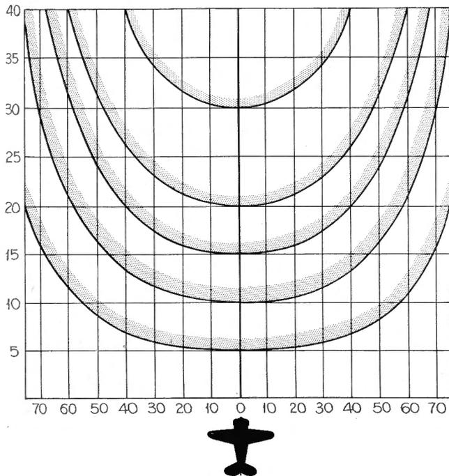
Figure 2. If an aircraft is flying perpendicular to an approximately straight coastline, the shore will appear as above. The closer the aircraft, the broader the indication will "fan out".
