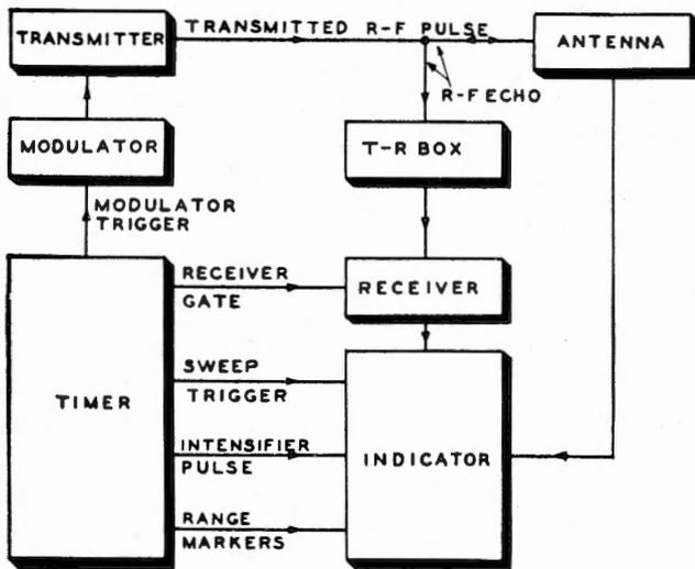
Fig. 1. Possible functions of a radar timer.
