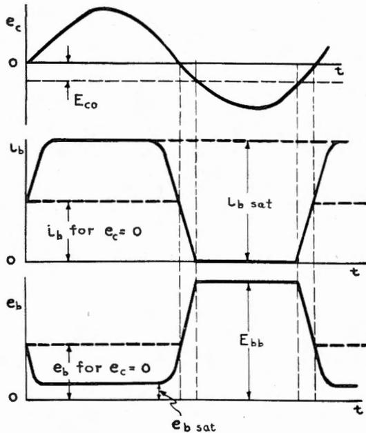
Fig. 11. Clipping by plate-current saturation.
