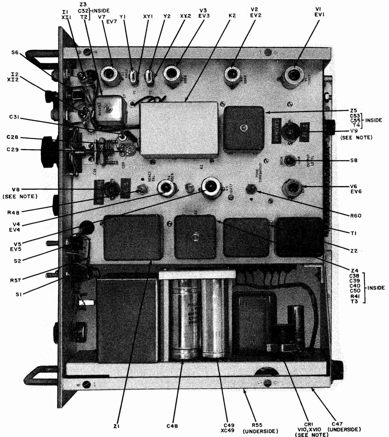
Figure 6-5. Single Sideband Converter CV-591A/URR, Top View, Parts Location
