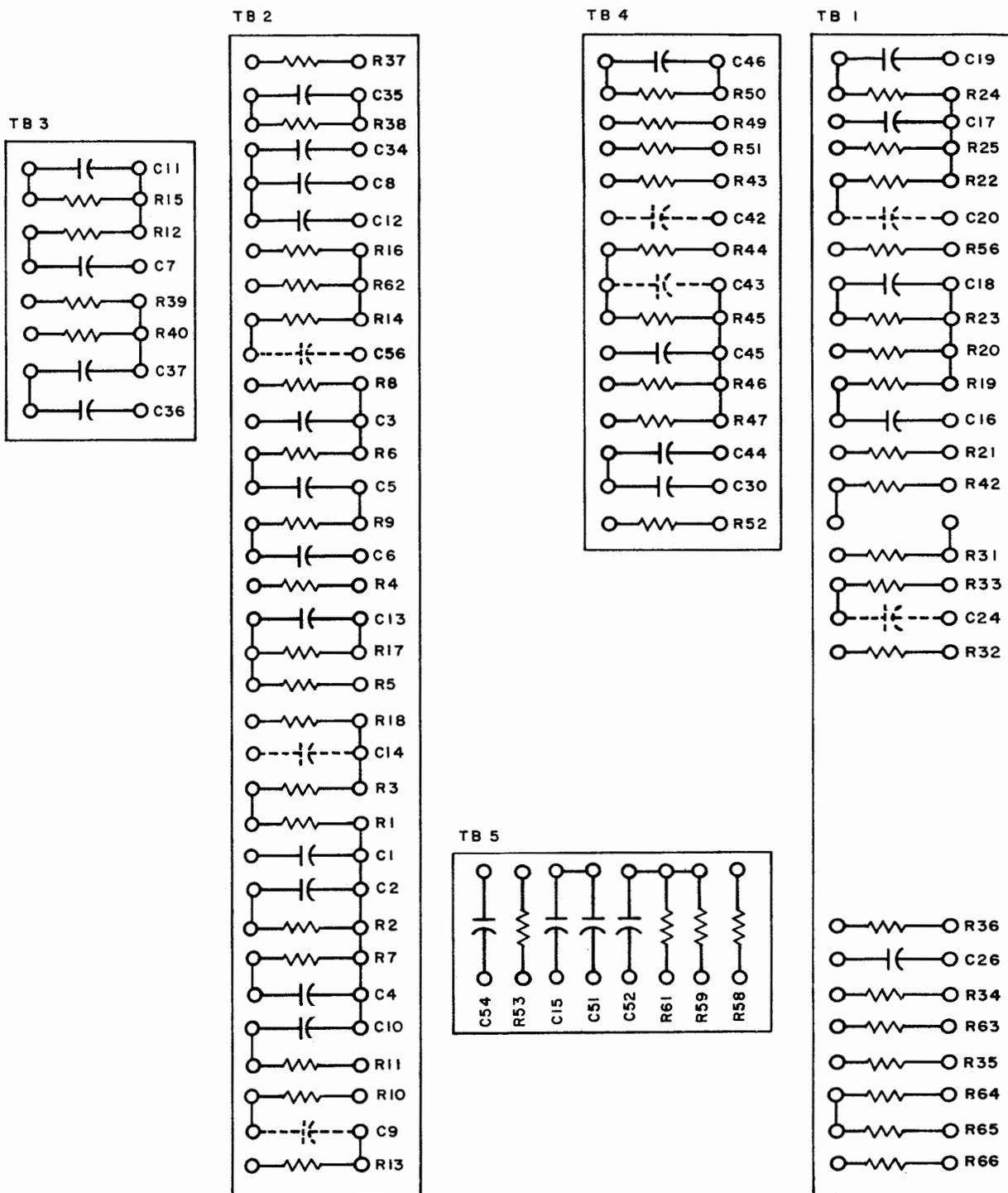
Figure 6-4. Single Sideband Converter CV-591A/URR, Parts Location on Terminal Boards
