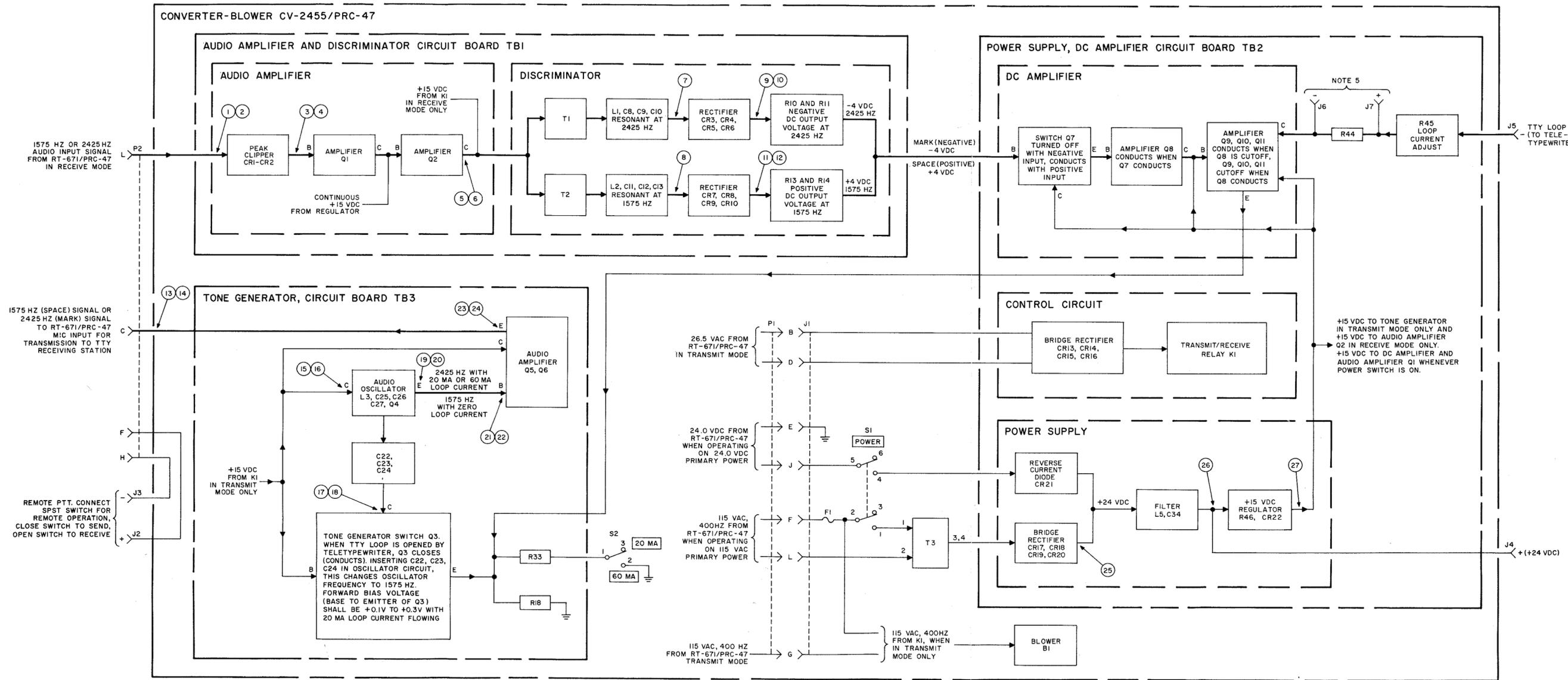
IN TRANSMIT MODE: FOR MARK OPERATION, THE TELETYPEWRITER CLOSSES THE LOOP CIRCUIT AND LOOP CURRENT (20 OR 60 MA) FLOWS. FOR SPACE CONDITION, THE LOOP CIRCUIT IS OPEN (ZERO LOOP CURRENT FLOW). WHEN LOOP CURRENT FLOWS FREQUENCY CONTROL TRANSISTOR Q3 CUTS OFF, RESULTING IN 2425 HZ OUTPUT TO RT-671/PRC-47. IF LOOP CURRENT IS ZERO, FREQUENCY CONTROL TRANSISTOR Q3 CONDUCTS, RESULTING IN 1575 HZ OUTPUT TO RT-671/PRC-47.
