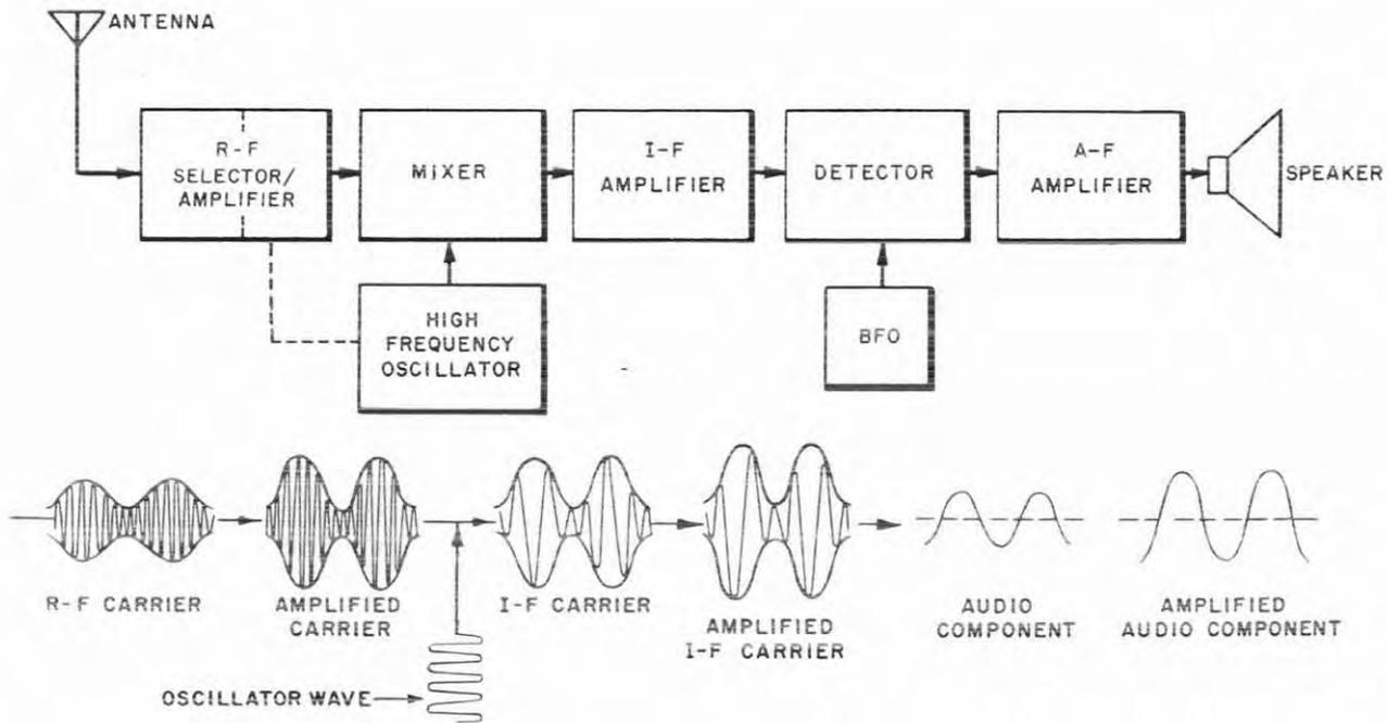
Figure 3-2.—Block diagram of a superheterodyne receiver.
