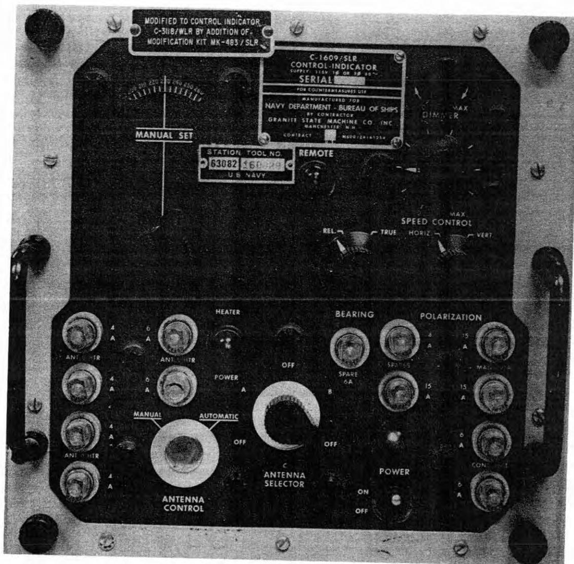
Figure 3-11.—C-3118/WLR antenna control unit.
