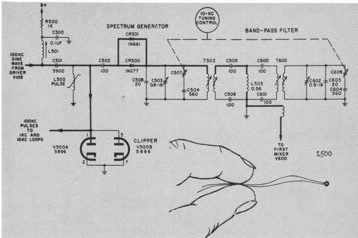
Figure 7 (above). Pulse generator.
