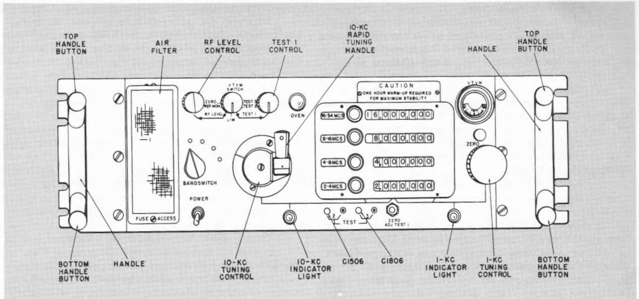
Figure 4. Front panel of synthesizer.
