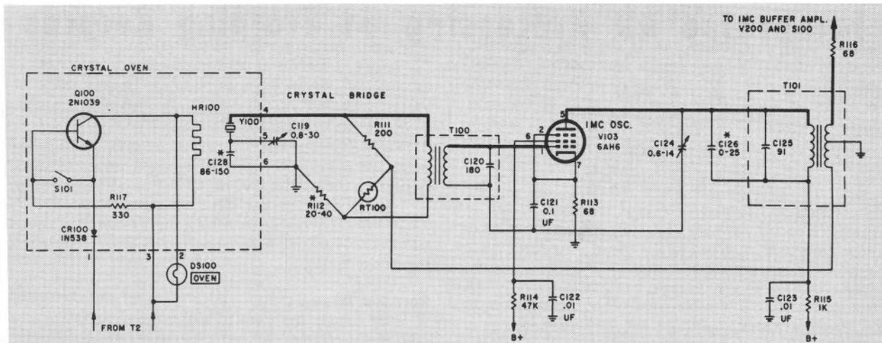
Figure 9. Meacham oscillator schematic.
